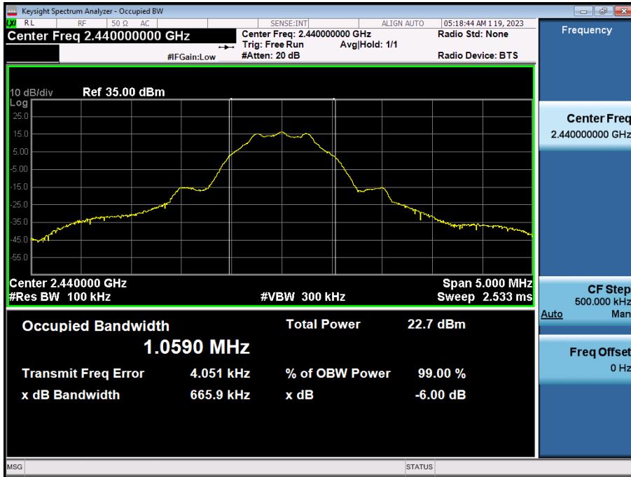
6 dB Bandwidth plot (Mid-CH 19)
