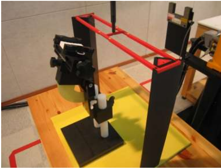
Figure 2. HAC Phantom & Device Holder
