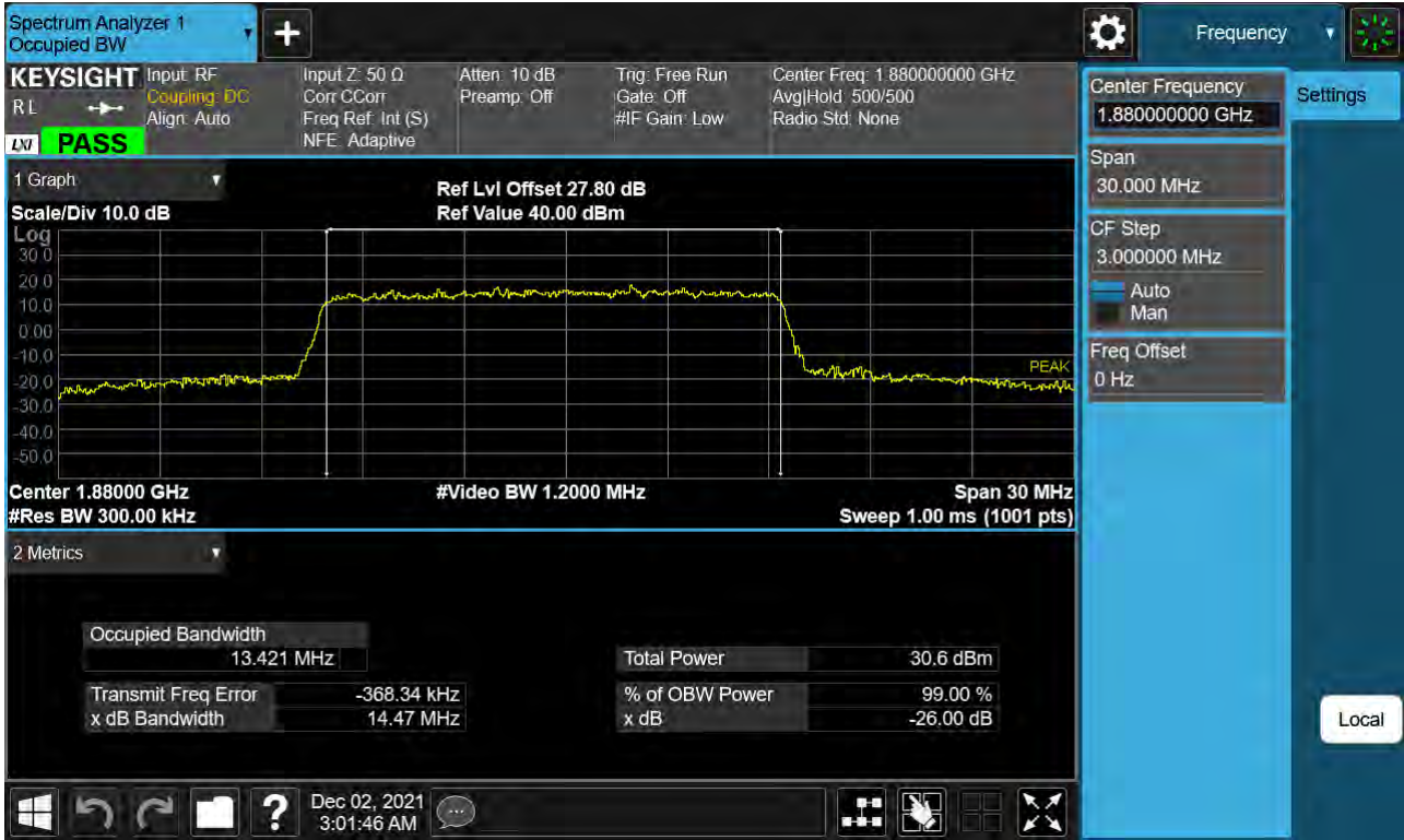
Sub6 n2. Occupied Bandwidth Plot (15 M BW Ch.376000 16QAM RB 75_0)
