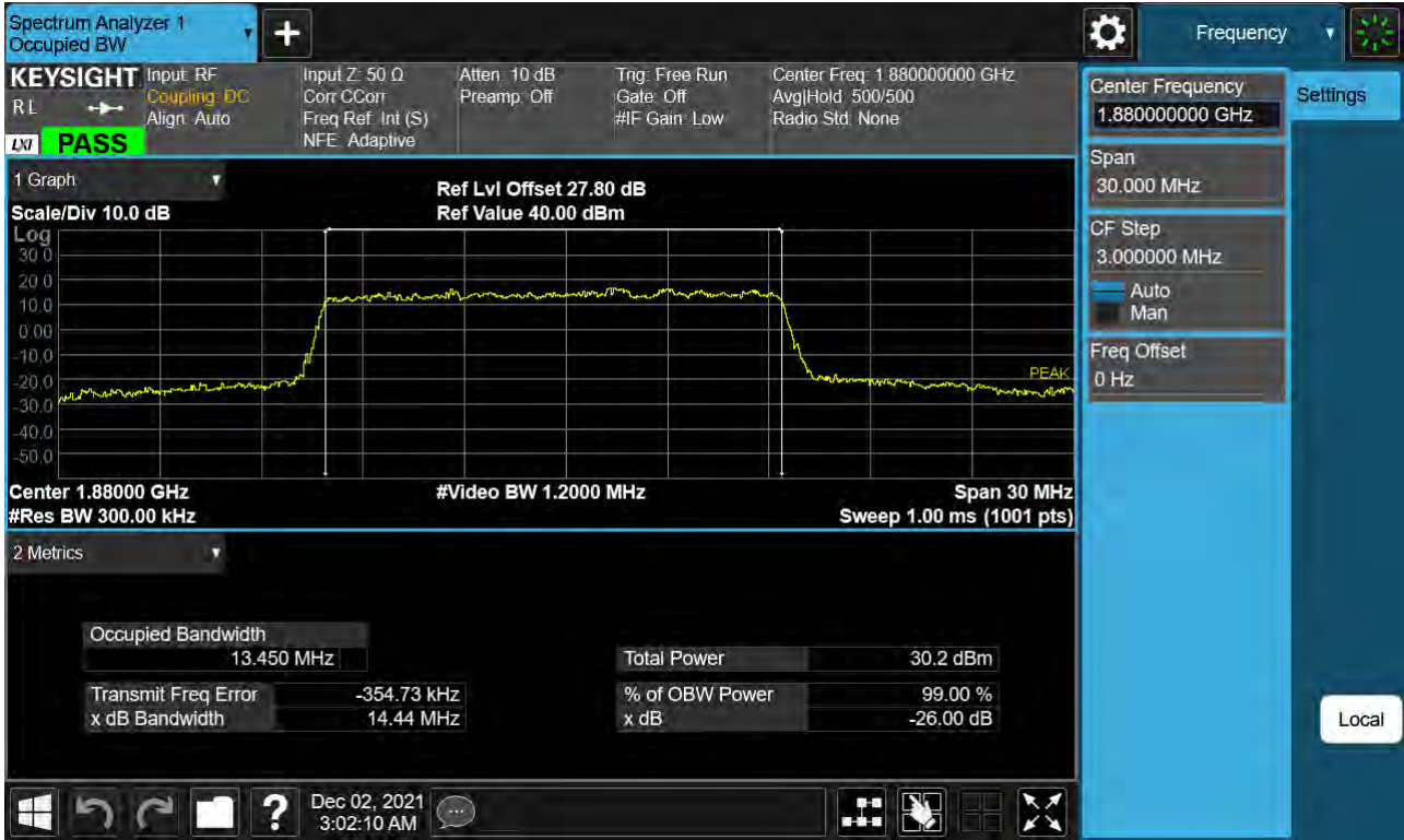
Sub6 n2. Occupied Bandwidth Plot (15 M BW Ch.376000 64QAM RB 75_0)
