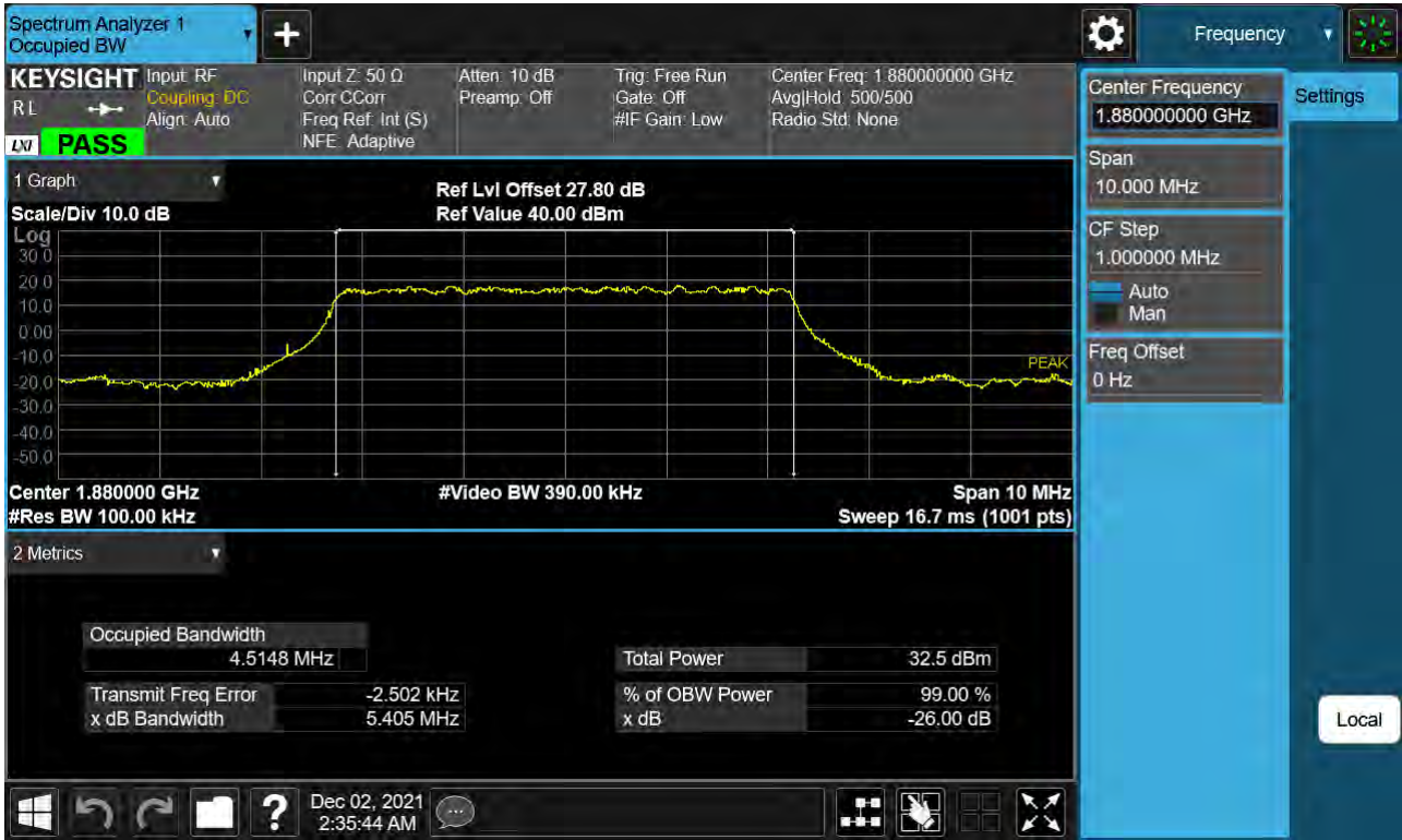
Sub6 n2. Occupied Bandwidth Plot (5 M BW Ch.376000 BPSK RB 25_0)
