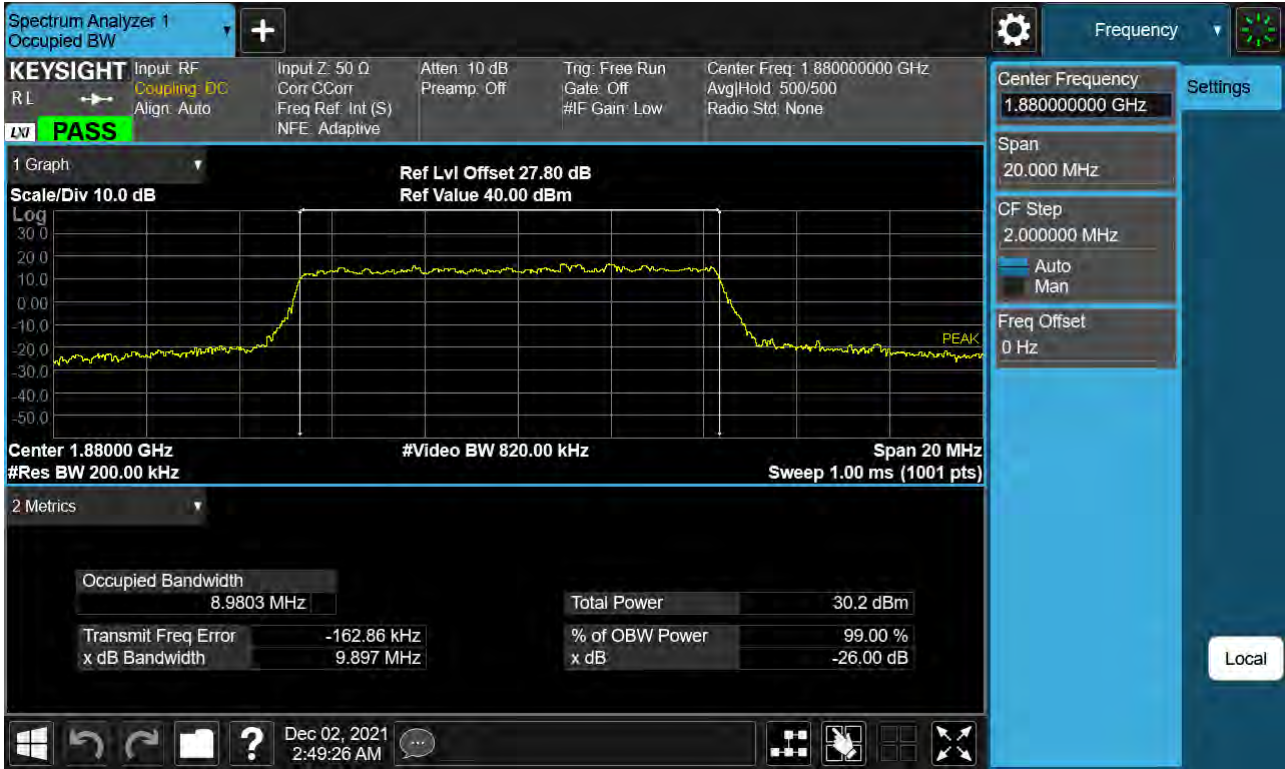
Sub6 n2. Occupied Bandwidth Plot (10 M BW Ch.376000 64QAM RB 50_0)
