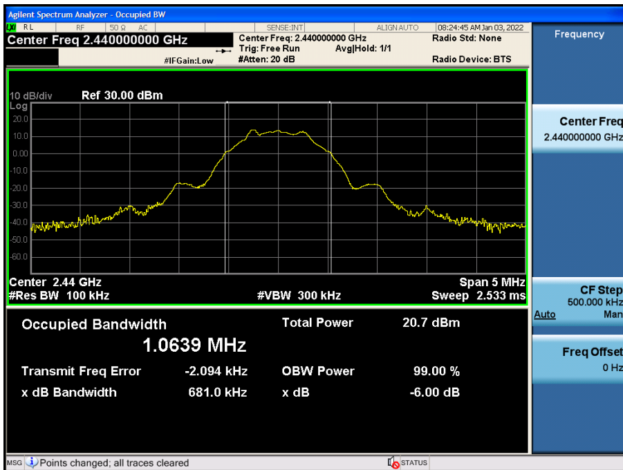
6 dB Bandwidth plot (Mid-CH 19)
