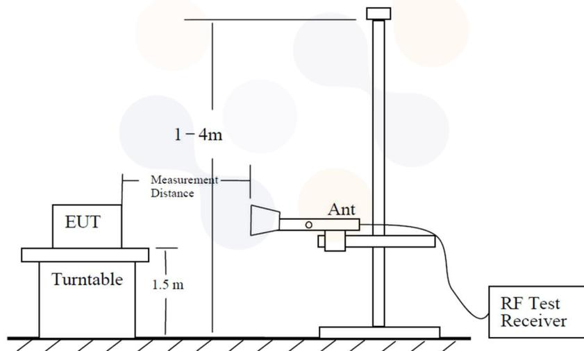
The diagram below shows the test setup for substituted method.
