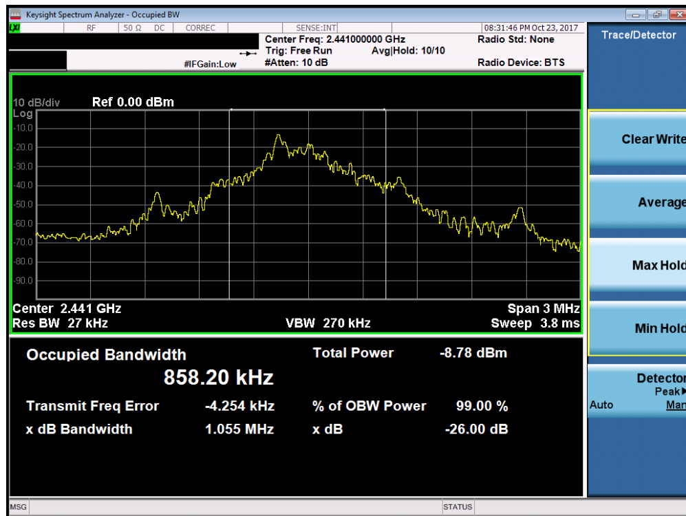
Plot 7-1. Occupied Bandwidth Plot (ANT+ – Ch. 39)
