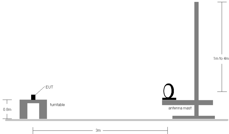
Figure 7-7. Radiated Test Setup < 30Mhz
