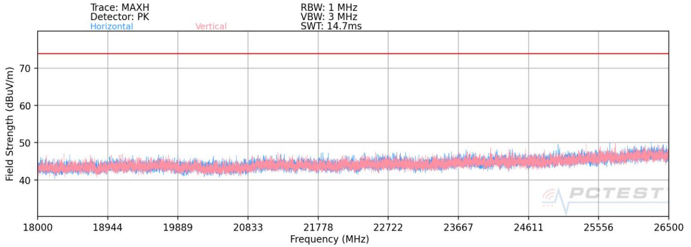
Plot 7-137. Radiated Spurious Plot 18GHz - 26.5GHz (802.11a)
