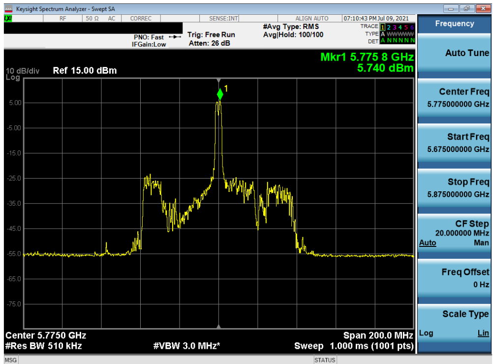
Plot 7-81. Power Spectral Density Plot (80MHz BW 802.11ax – 26 Tones (UNII Band 3) – Ch. 155)
