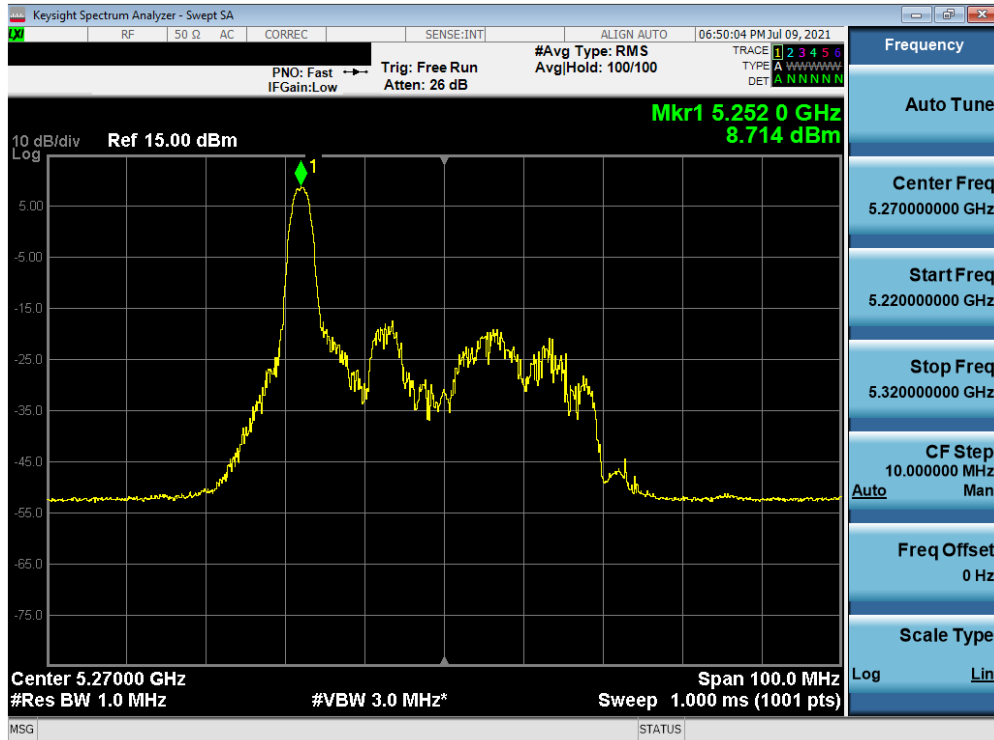
Plot 7-64. Power Spectral Density Plot (40MHz BW 802.11ax – 26 Tones (UNII Band 2A) – Ch. 54)
