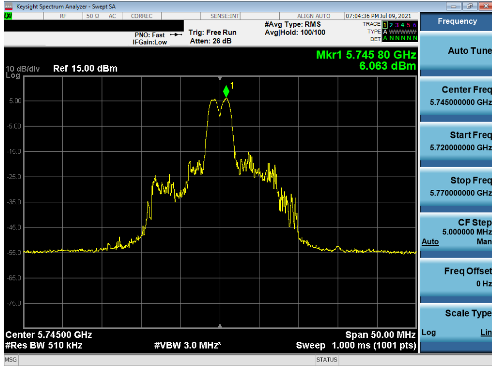
Plot 7-76. Power Spectral Density Plot (20MHz BW 802.11ax – 26 Tones (UNII Band 3) – Ch. 149)
