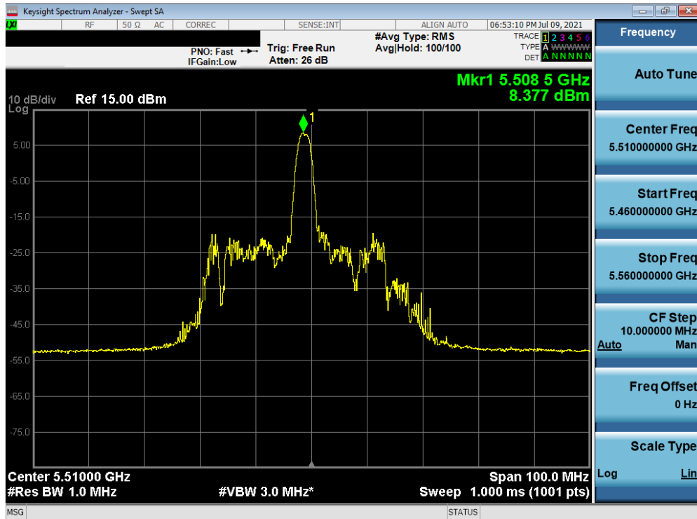
Plot 7-70. Power Spectral Density Plot (40MHz BW 802.11ax – 26 Tones (UNII Band 2C) – Ch. 102)
