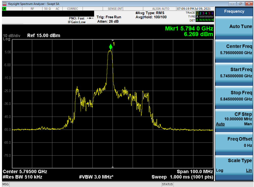
Plot 7-80. Power Spectral Density Plot (40MHz BW 802.11ax – 26 Tones (UNII Band 3) – Ch. 159)
