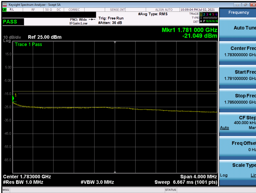
Plot 7-123. Upper Extended Band Edge Plot (NR Band n66 – 15.0MHz - Full RB)
