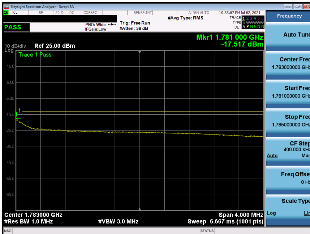
Plot 7-127. Upper Extended Band Edge Plot (NR Band n66 – 10.0MHz - Full RB)
