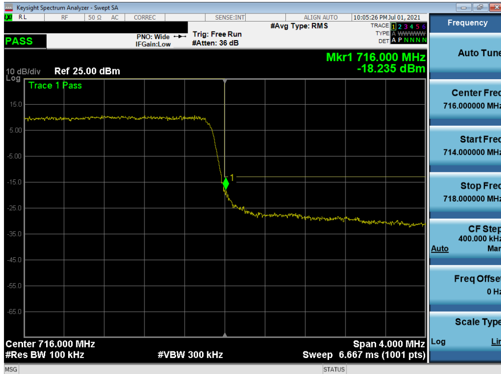
Plot 7-77. Upper Band Edge Plot (LTE Band 12/17 - 3MHz QPSK – Full RB)
