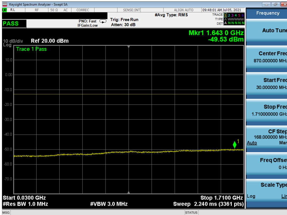
Plot 7-46. Conducted Spurious Plot (WCDMA Ch. 1413- Mid Channel)
