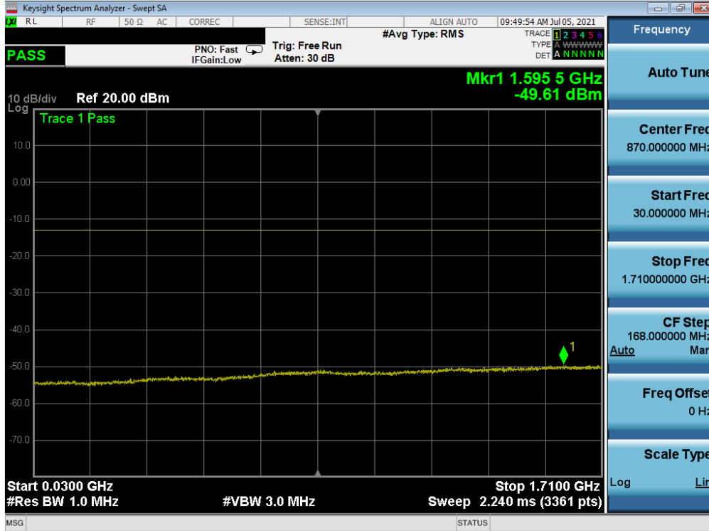
Plot 7-49. Conducted Spurious Plot (WCDMA Ch. 1513- High Channel)
