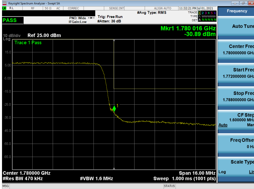
Plot 7-84. Upper Band Edge Plot (LTE Band 66 - 20MHz QPSK – Full RB)
