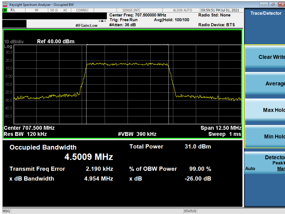
Plot 7-4. Occupied Bandwidth Plot (LTE Band 12/17 - 5MHz 16-QAM - Full RB)
