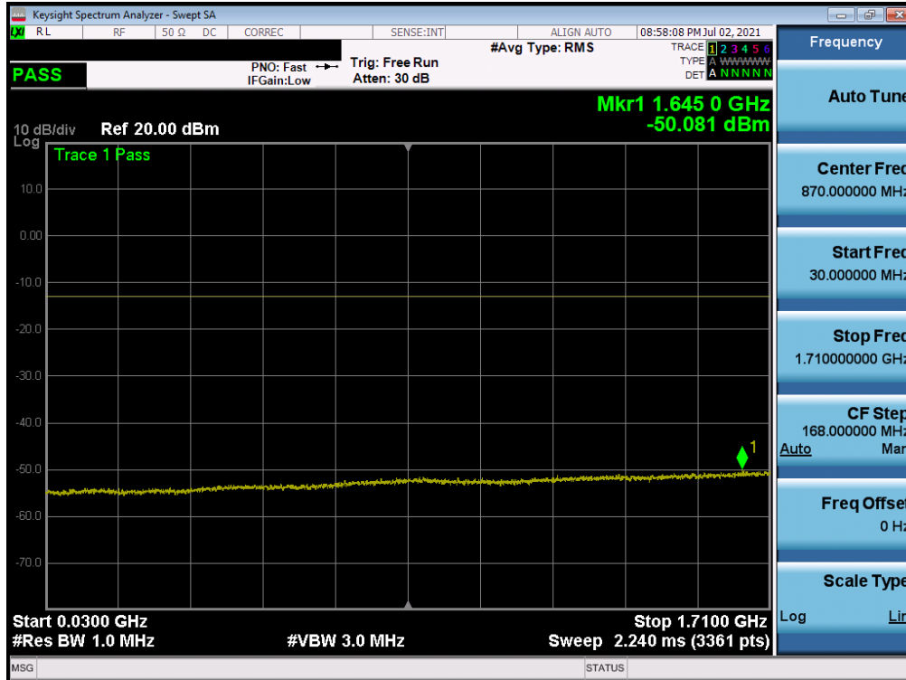
Plot 7-67. Conducted Spurious Plot (NR Band n66 - 20.0MHz - 1 RB - High Channel)
