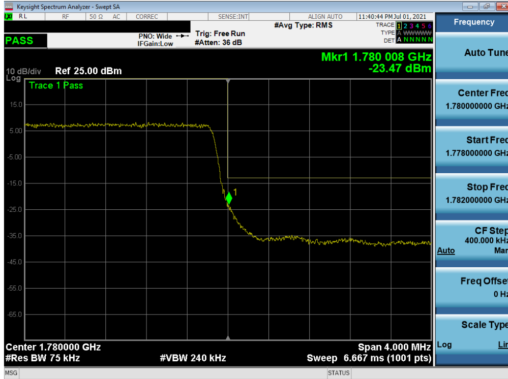
Plot 7-108. Upper Band Edge Plot (LTE Band 66 - 3MHz QPSK – Full RB)
