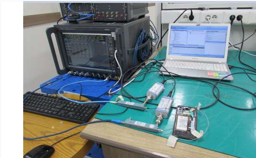
Test setup photo- 3 (7-1(c)NR FR1power measurement)
