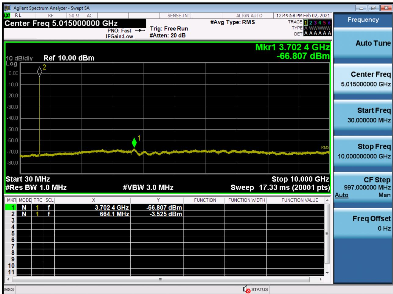
BAND 71. Conducted Spurious Plot \_ (133297ch\_10MHz\_QPSK\_RB 1\_0)
