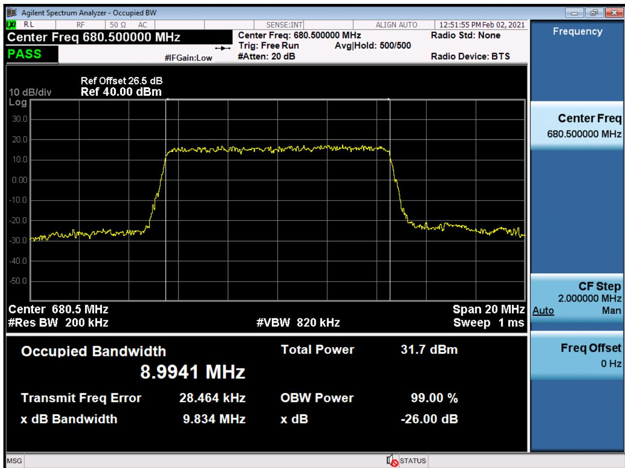
BAND 71. Occupied Bandwidth Plot (10M BW Ch.133297 16QAM\_RB15\_0)
