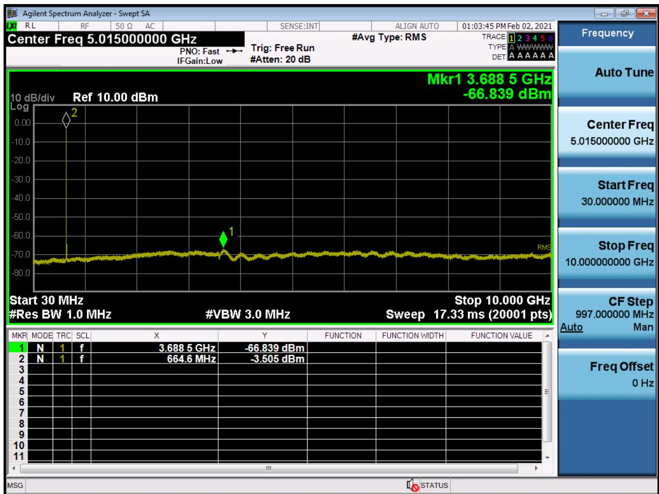
BAND 71. Conducted Spurious Plot \_ (133297ch\_20MHz\_QPSK\_RB 1\_0)
