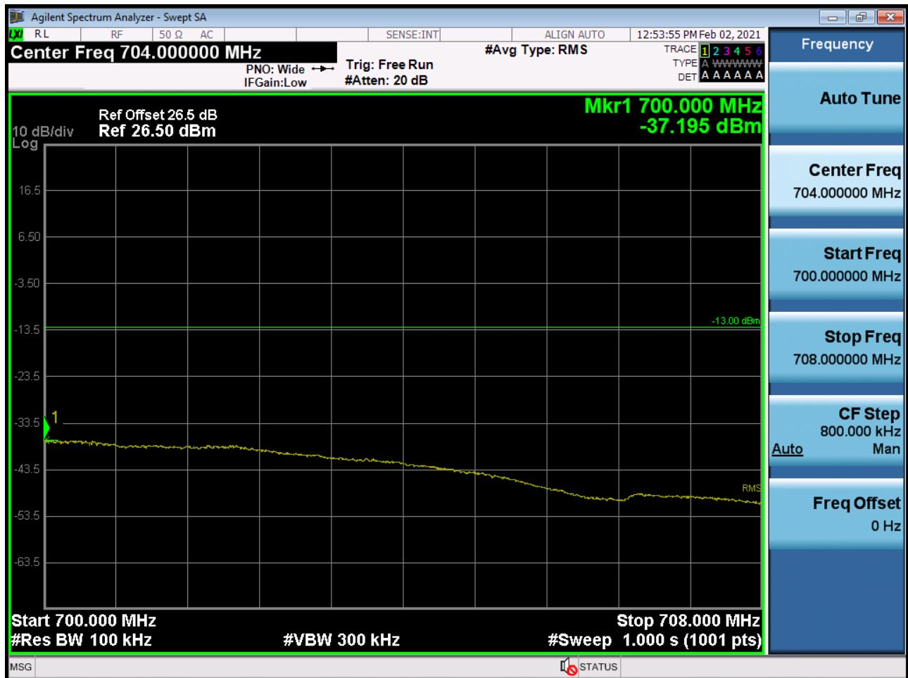
BAND 71. Upper Band Edge Plot (15M BW Ch.133397 QPSK\_RB1\_Offset 24)
