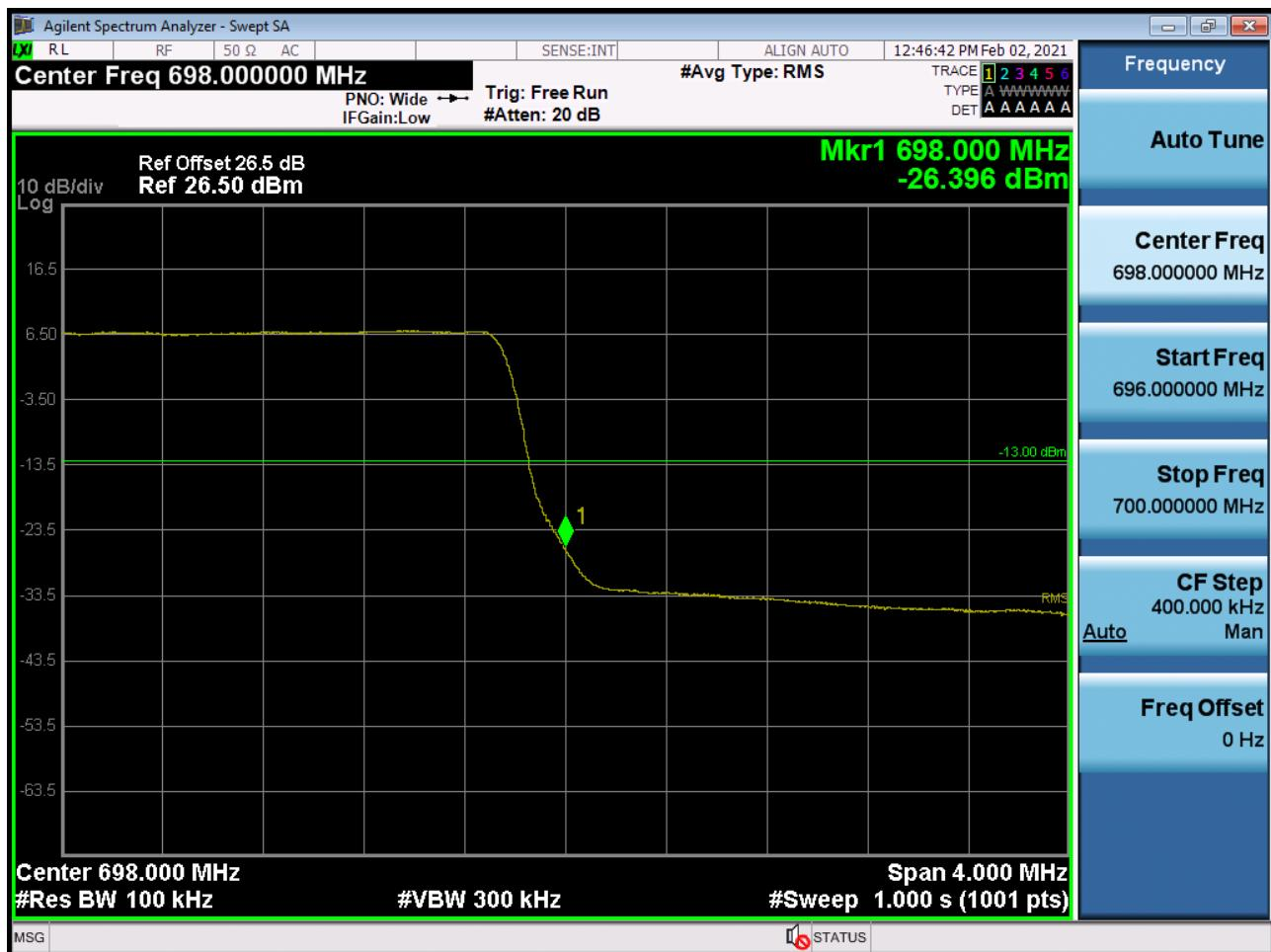
BAND 71. Upper Extended Band Edge Plot (5M BW Ch.133447 QPSK\_RB6\_0)
