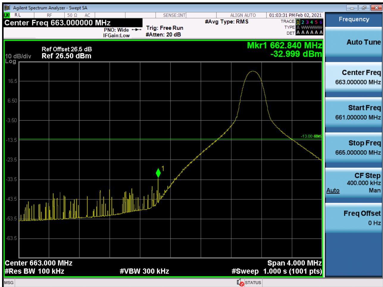
BAND 71. Lower Band Edge Plot (20M BW Ch.133222 QPSK\_RB50\_Offset 0)
