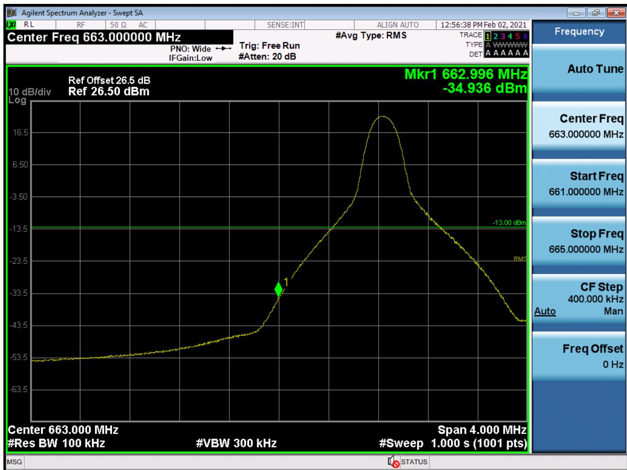
BAND 71. Lower Band Edge Plot (15M BW Ch.133197 QPSK\_RB25\_Offset 0)
