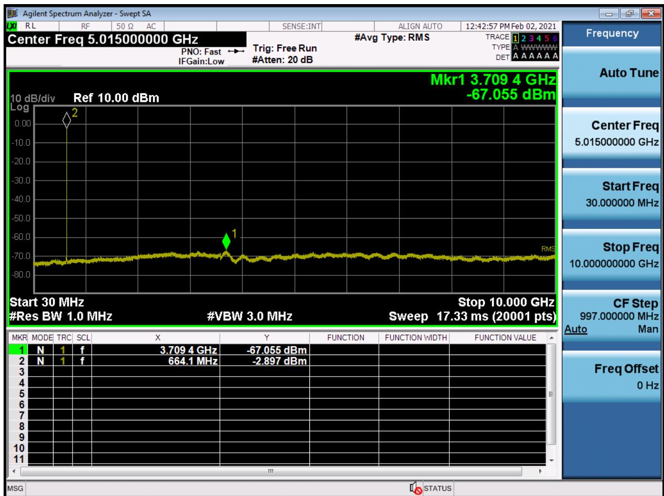
BAND 71. Conducted Spurious Plot \_ (133297ch\_5MHz\_QPSK\_RB 1\_0)
