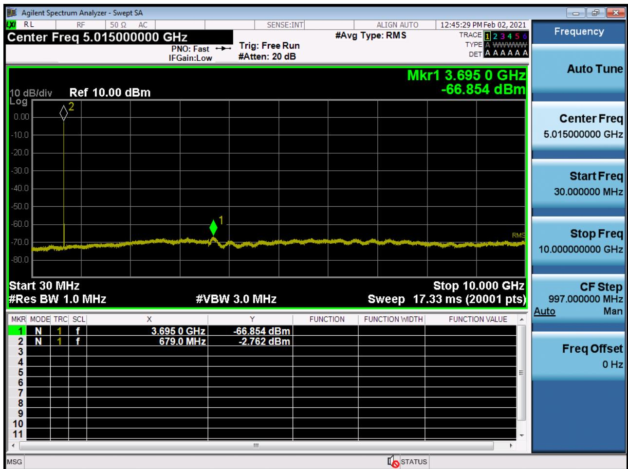
BAND 71. Conducted Spurious Plot \_ (133447ch\_5MHz\_QPSK\_RB 1\_0)
