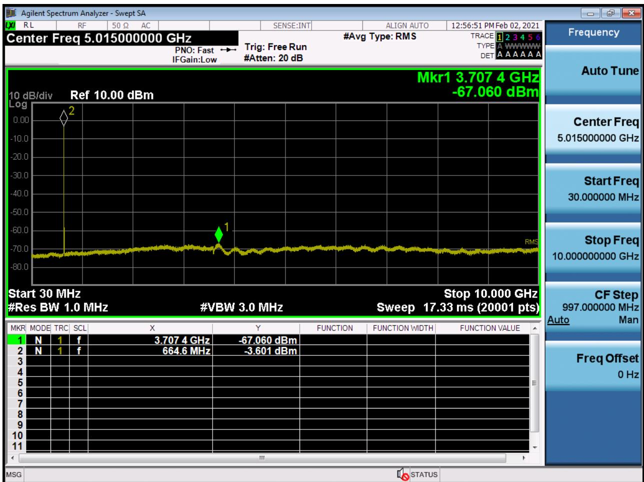
BAND 71. Conducted Spurious Plot \_ (133297ch\_15MHz\_QPSK\_RB 1\_0)
