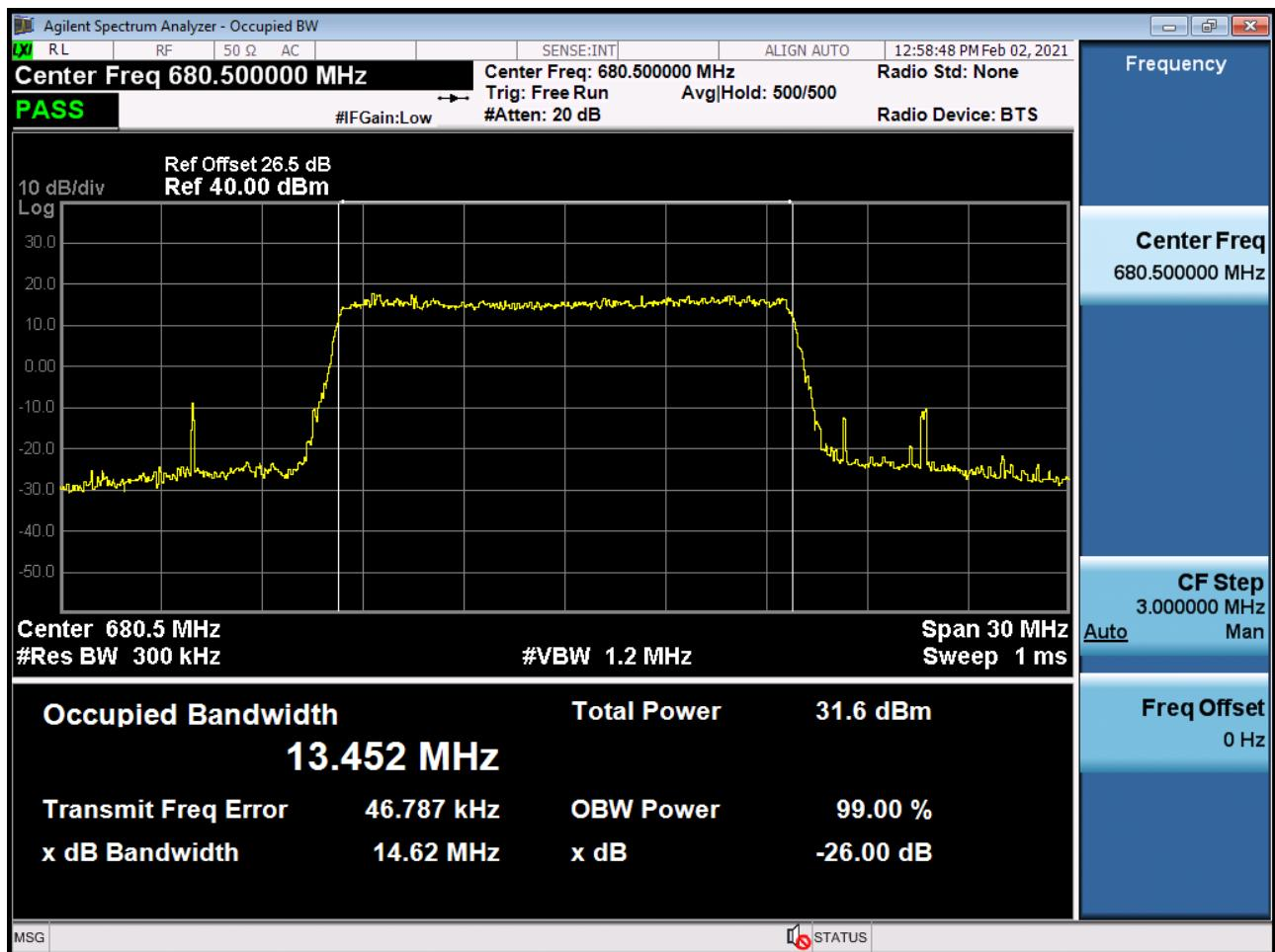
BAND 71. Occupied Bandwidth Plot (15M BW Ch.133297 16QAM\_RB25\_0)
