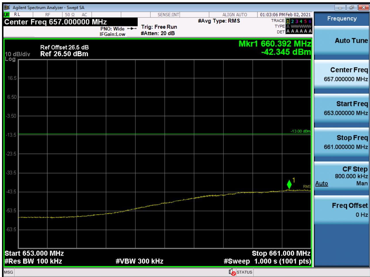
BAND 71. Upper Band Edge Plot (5M BW Ch.133447 QPSK\_RB1\_Offset 5)
