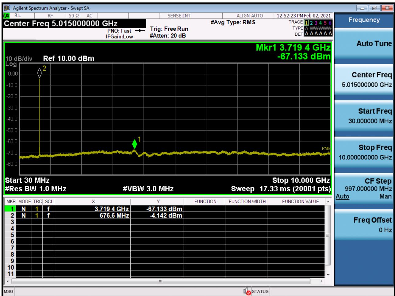
BAND 71. Conducted Spurious Plot \_ (133422ch\_10MHz\_QPSK\_RB 1\_0)
