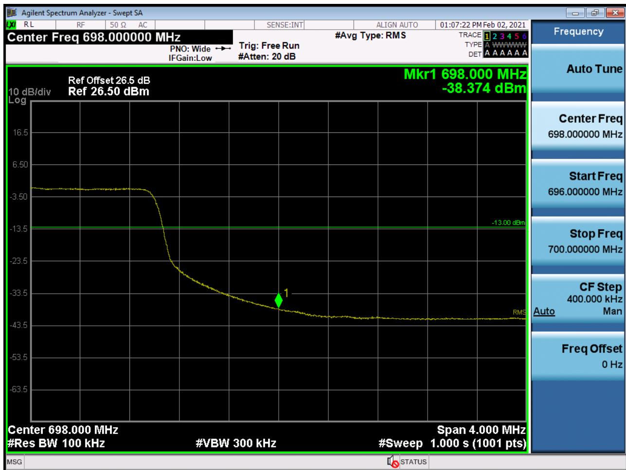
BAND 71. Upper Extended Band Edge Plot (20M BW Ch.133372 QPSK\_RB50\_0)
