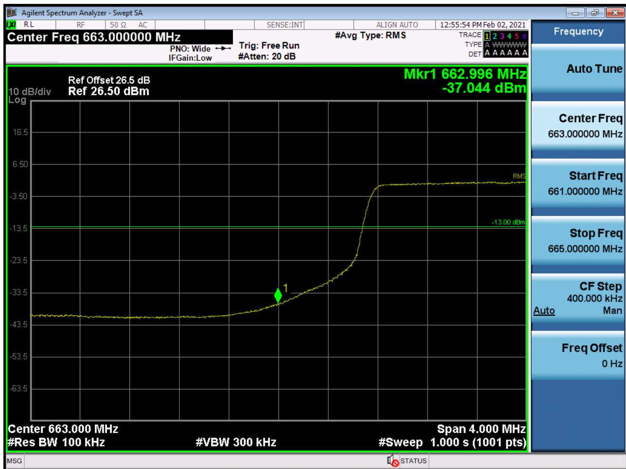
BAND 71. Lower Extended Band Edge Plot (15M BW Ch.133197 QPSK\_RB25\_0)
