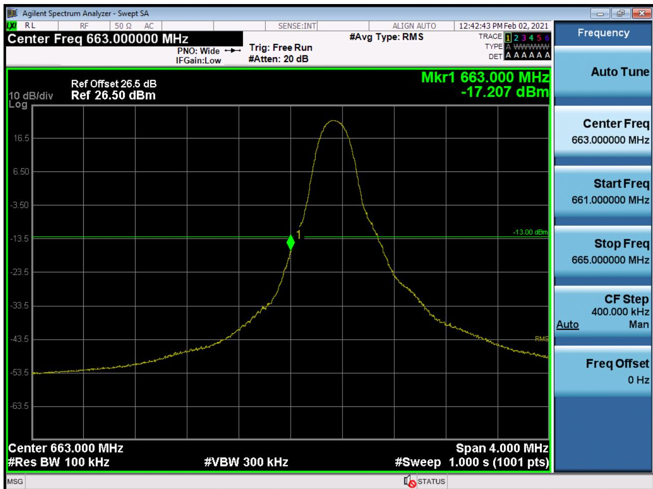
BAND 71. Lower Band Edge Plot (5M BW Ch.133147 QPSK\_RB6\_Offset 0)
