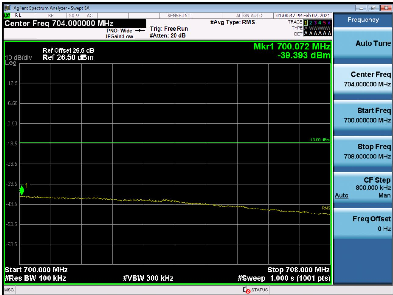
BAND 71. Upper Band Edge Plot (20M BW Ch.133372 QPSK\_RB1\_Offset 49)
