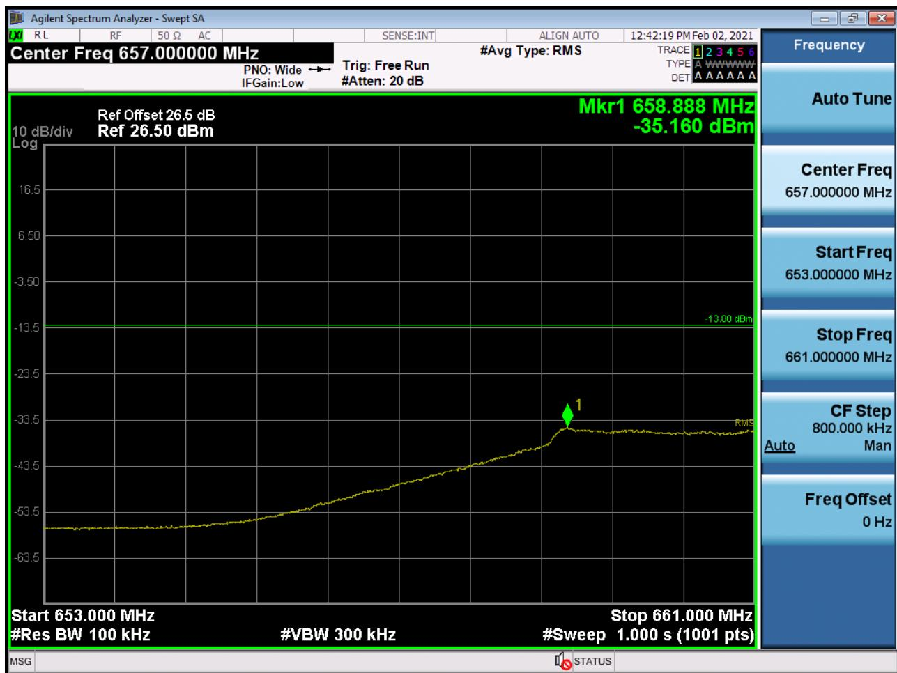
BAND 71. Lower Band Edge Plot (10M BW Ch.133172 QPSK\_RB1\_Offset 0)
