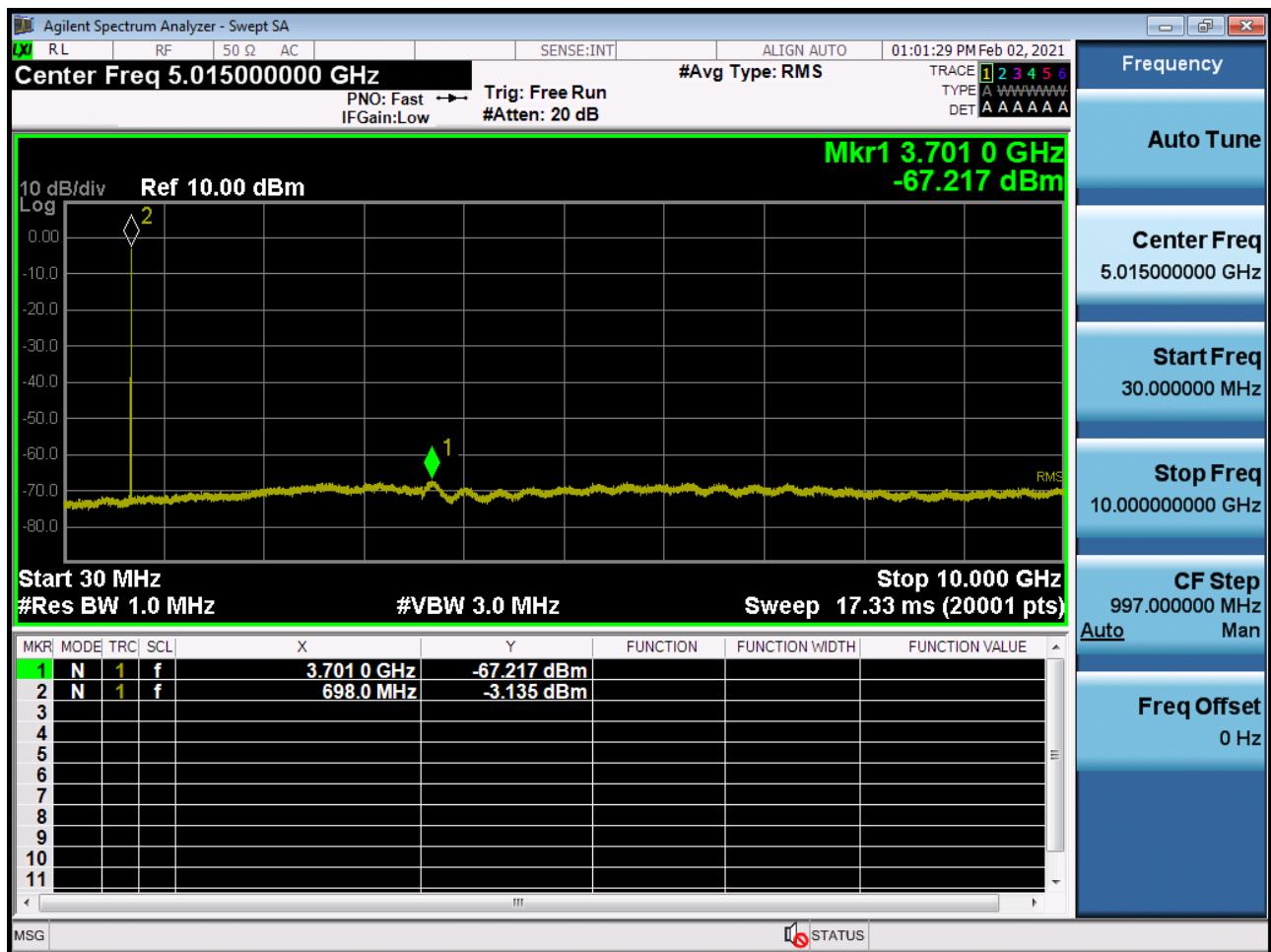
BAND 71. Conducted Spurious Plot \_ (133222ch\_20MHz\_QPSK\_RB 1\_0)
