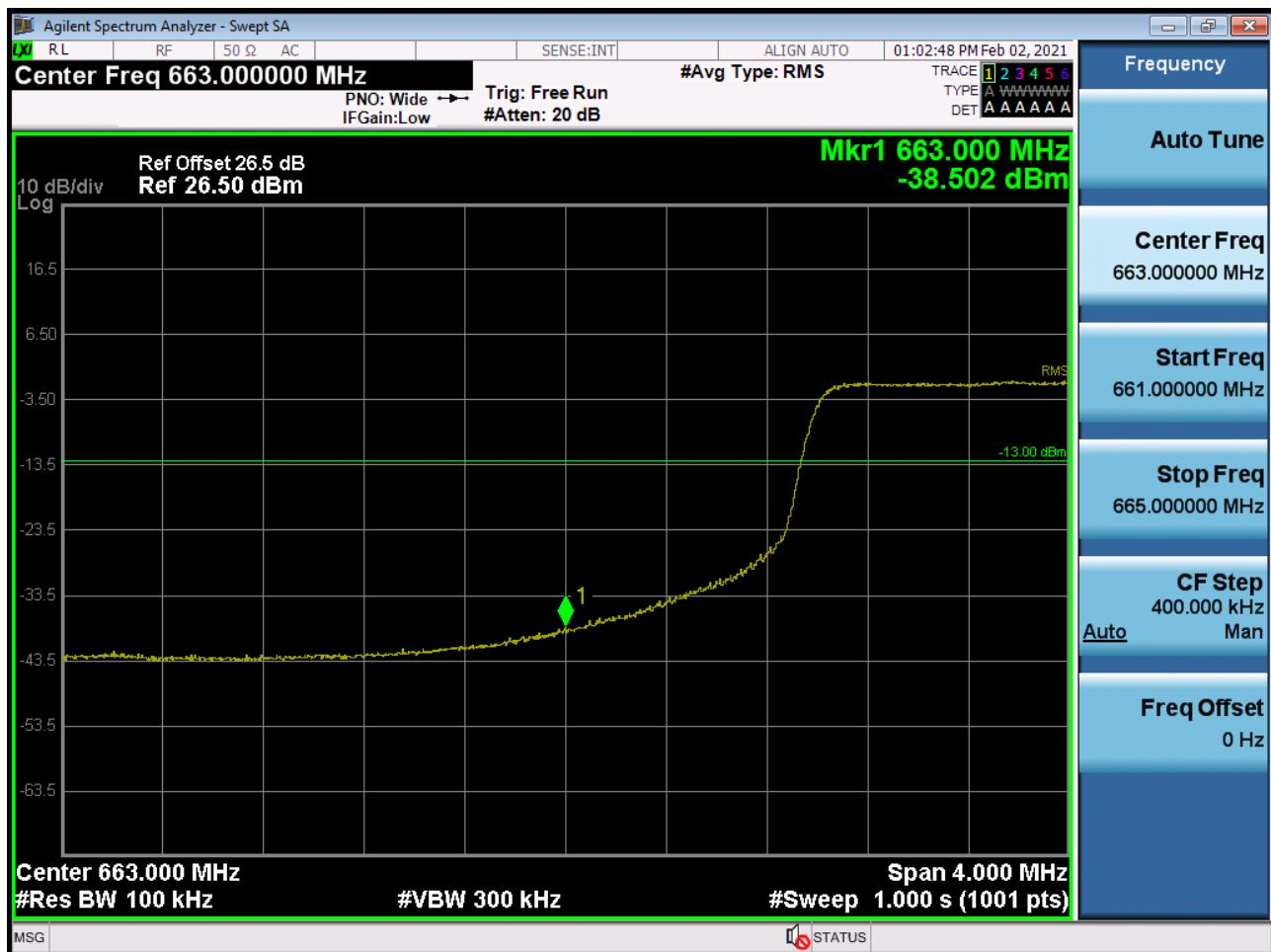
BAND 71. Lower Extended Band Edge Plot (20M BW Ch.133222 QPSK\_RB50\_0)
