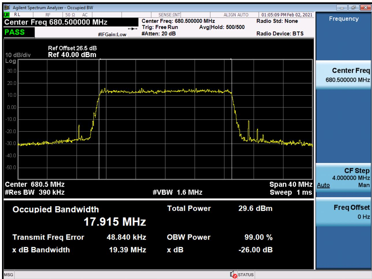
BAND 71. Lower Band Edge Plot (5M BW Ch.133147 QPSK\_RB1\_Offset 0)
