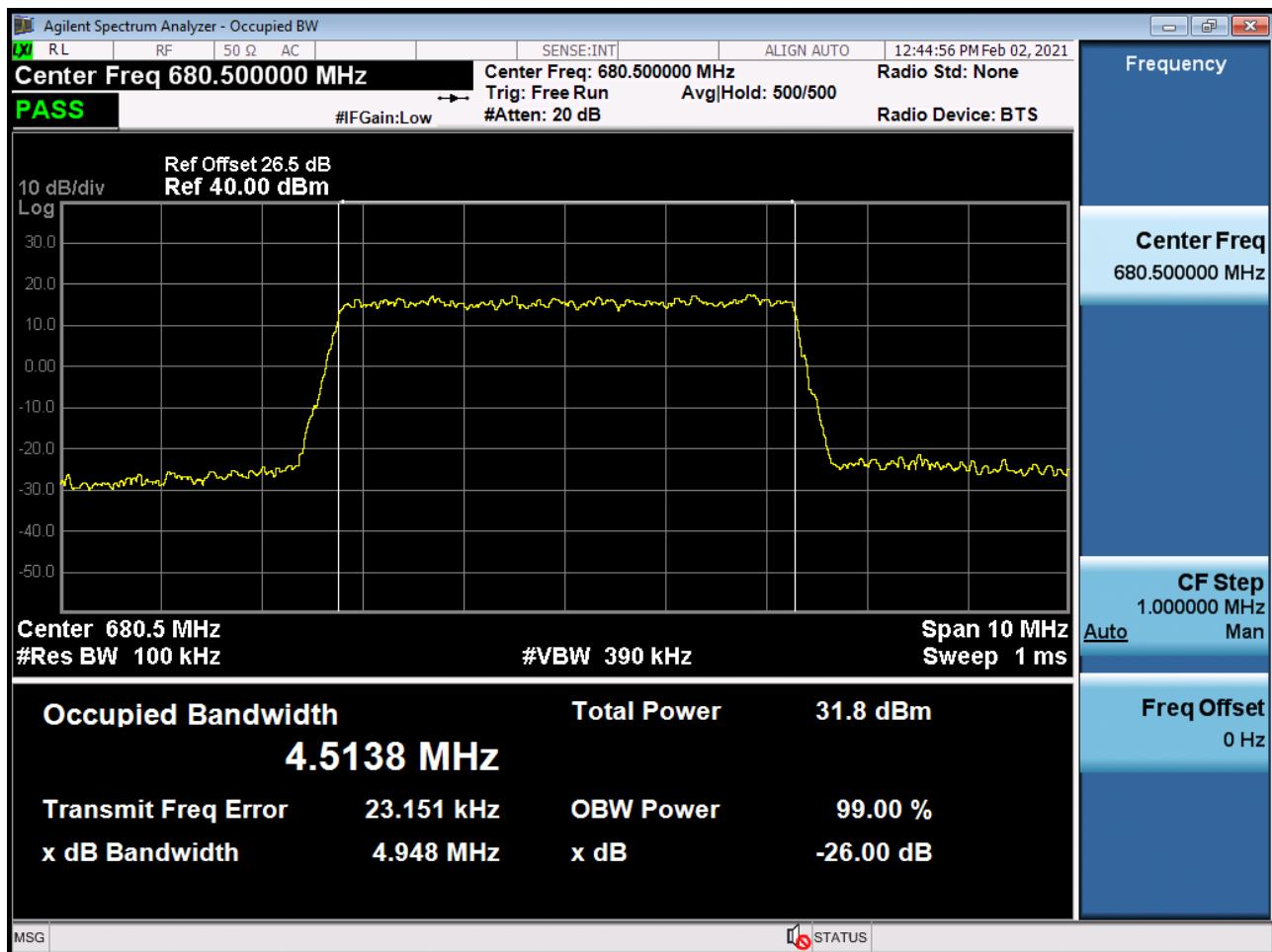
BAND 71. Occupied Bandwidth Plot (5M BW Ch.133297 16QAM\_RB6\_0)
