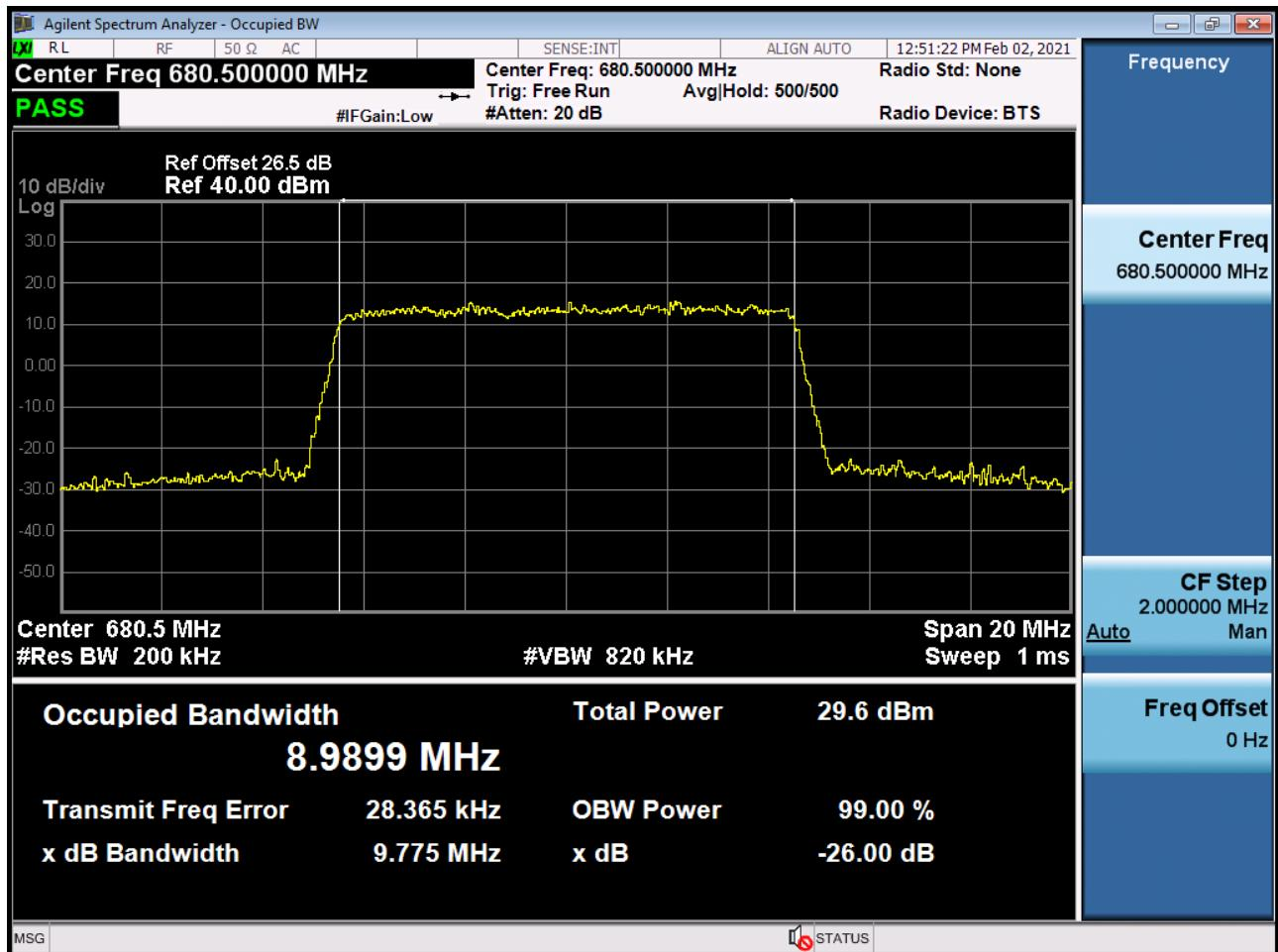
BAND 71. Occupied Bandwidth Plot (15M BW Ch.133297 QPSK\_RB25\_0)
