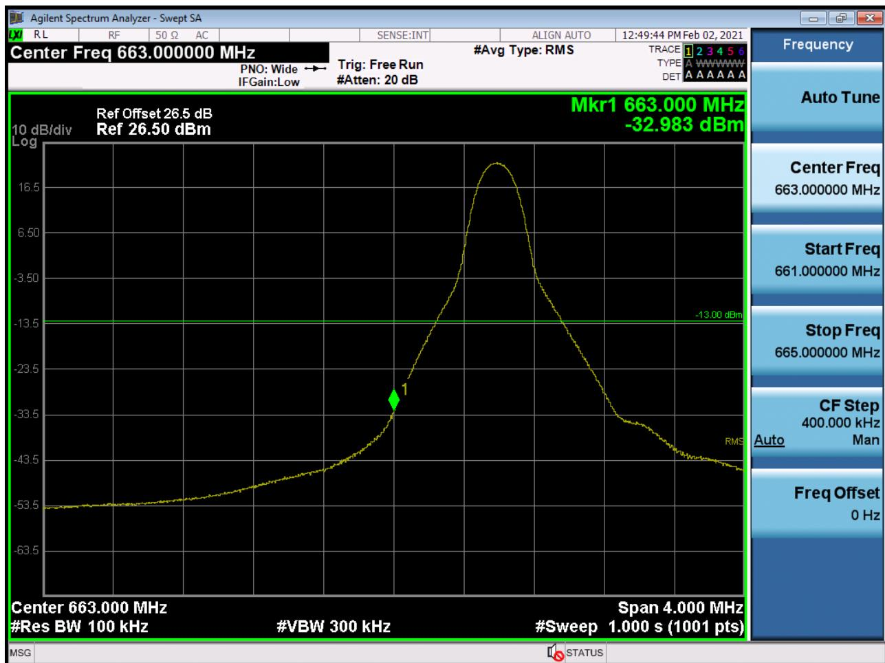
BAND 71. Lower Band Edge Plot (10M BW Ch.133172 QPSK\_RB15\_Offset 0)
