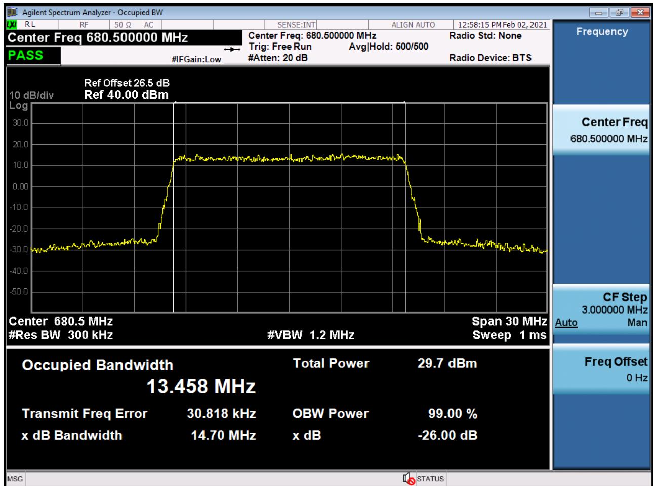
BAND 71. Occupied Bandwidth Plot (20M BW Ch.133297 QPSK\_RB50\_0)
