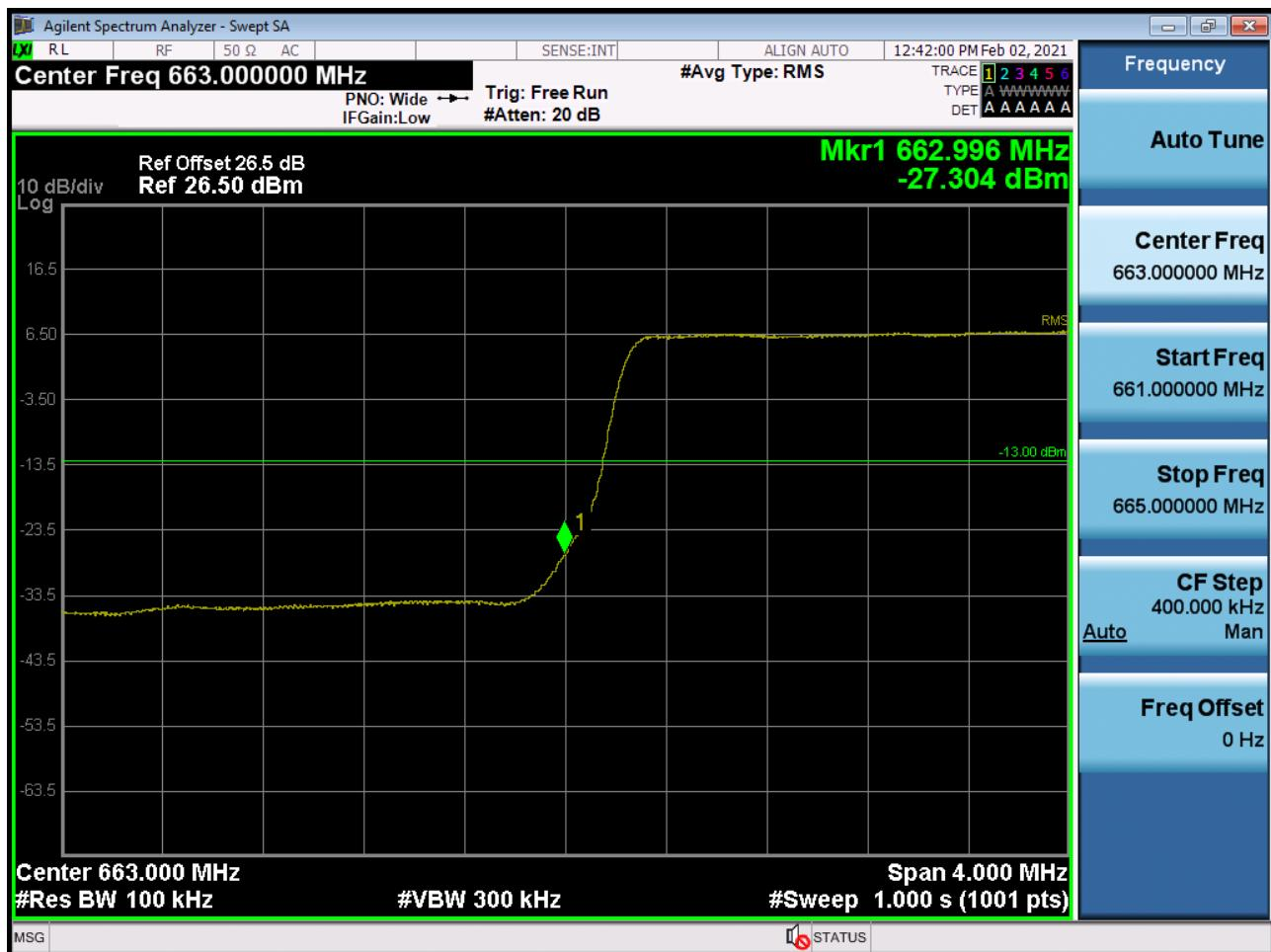
BAND 71. Lower Extended Band Edge Plot (5M BW Ch.133147 QPSK\_RB6\_0)
