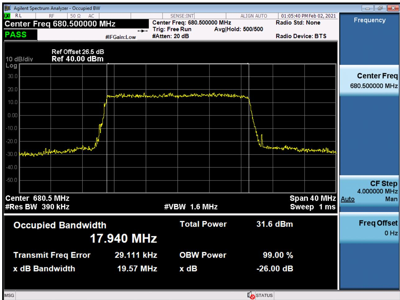
BAND 71. Occupied Bandwidth Plot (20M BW Ch.133297 16QAM\_RB50\_0)
