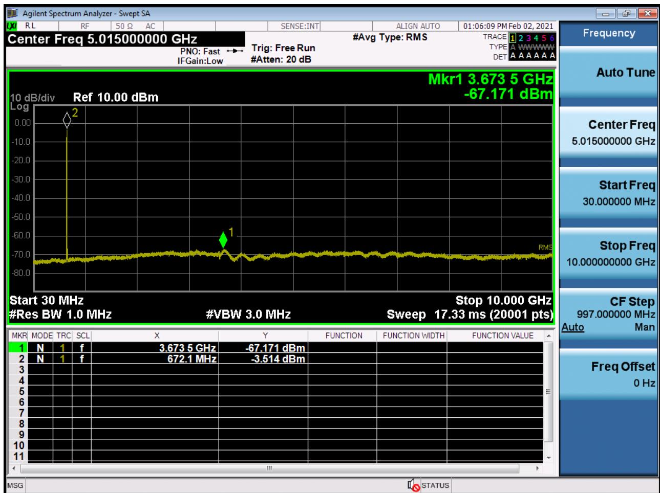
BAND 71. Conducted Spurious Plot \_ (133372ch\_20MHz\_QPSK\_RB 1\_0)
