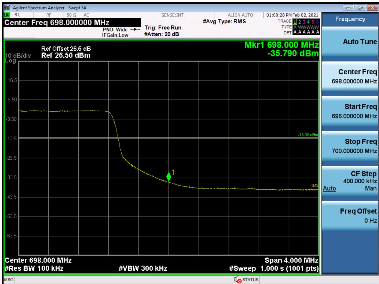
BAND 71. Upper Extended Band Edge Plot (15M BW Ch.133397 QPSK\_RB25\_0)
