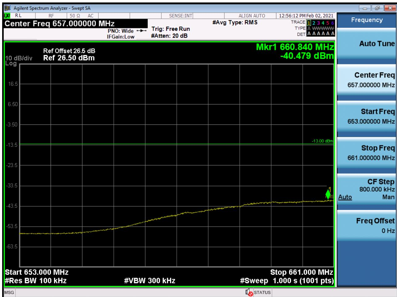
BAND 71. Lower Band Edge Plot (20M BW Ch.133222 QPSK\_RB1\_Offset 0)
