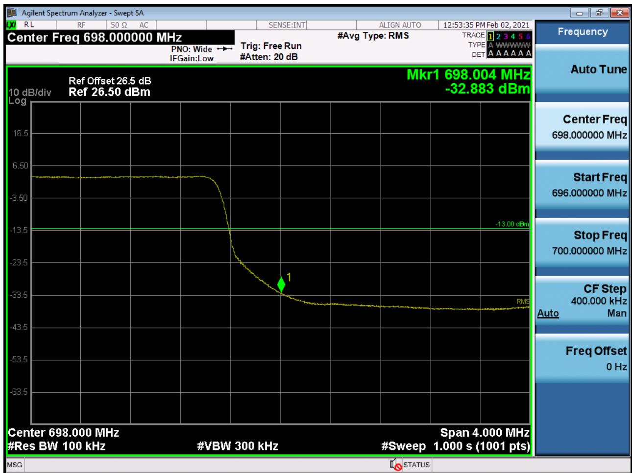
BAND 71. Upper Extended Band Edge Plot (10M BW Ch.133422 QPSK\_RB15\_0)
