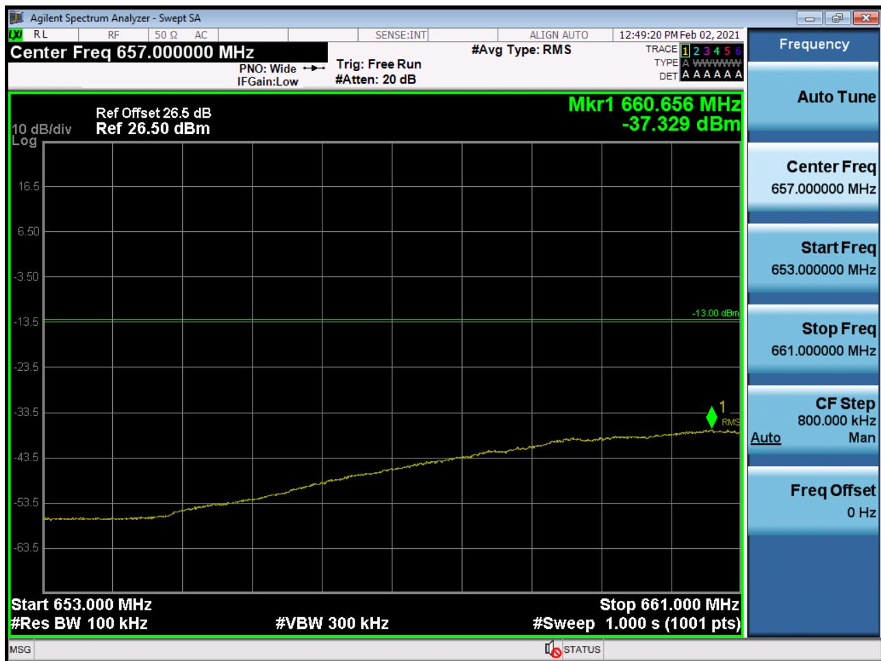
BAND 71. Lower Band Edge Plot (15M BW Ch.133197 QPSK\_RB1\_Offset 0)
