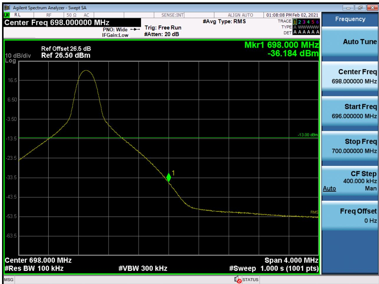
BAND 71. Upper Band Edge Plot (20M BW Ch.133372 QPSK\_RB50\_Offset 0)
