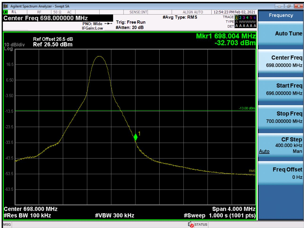
BAND 71. Upper Band Edge Plot (10M BW Ch.133422 QPSK\_RB1\_Offset 14)
