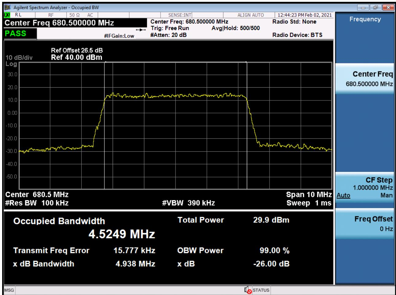
BAND 71. Occupied Bandwidth Plot (10M BW Ch.133297 QPSK\_RB15\_0)
