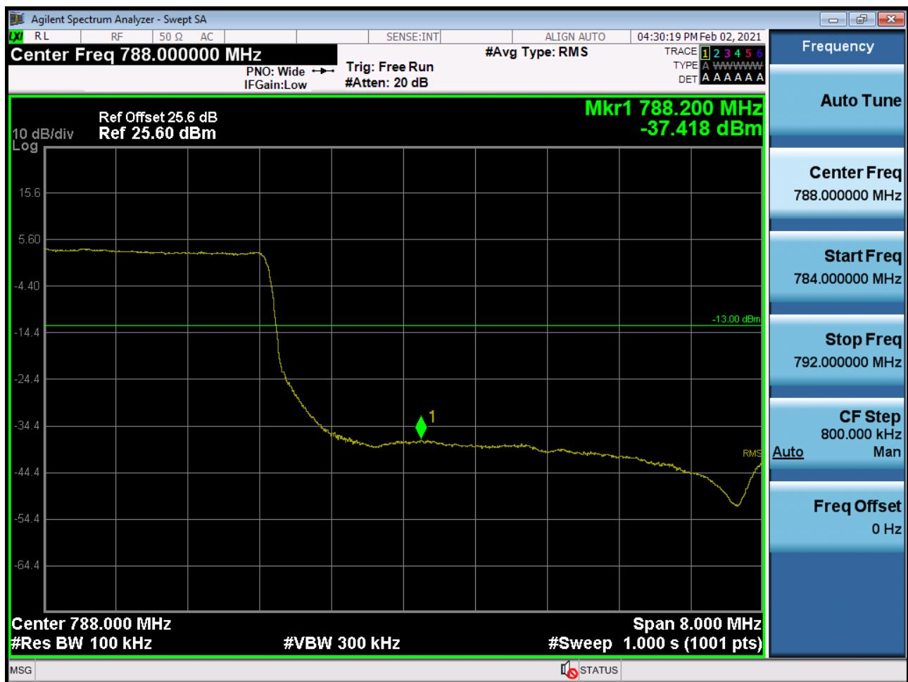
Band 13 Upper Emission Mask (793 MHz ~805 MHz) Plot (10M BW Ch.23230 QPSK\_RB50\_0)-2
