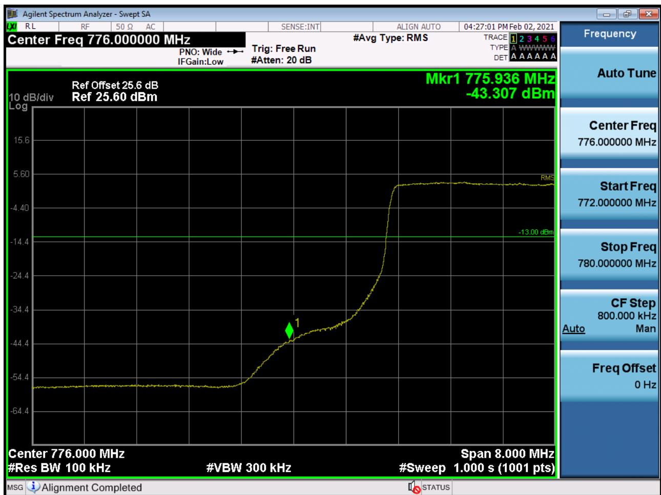
Band 13 Lower Emission Mask (763 MHz ~ 775 MHz) Plot (10M BW Ch.23230 QPSK\_RB50\_0)-2
