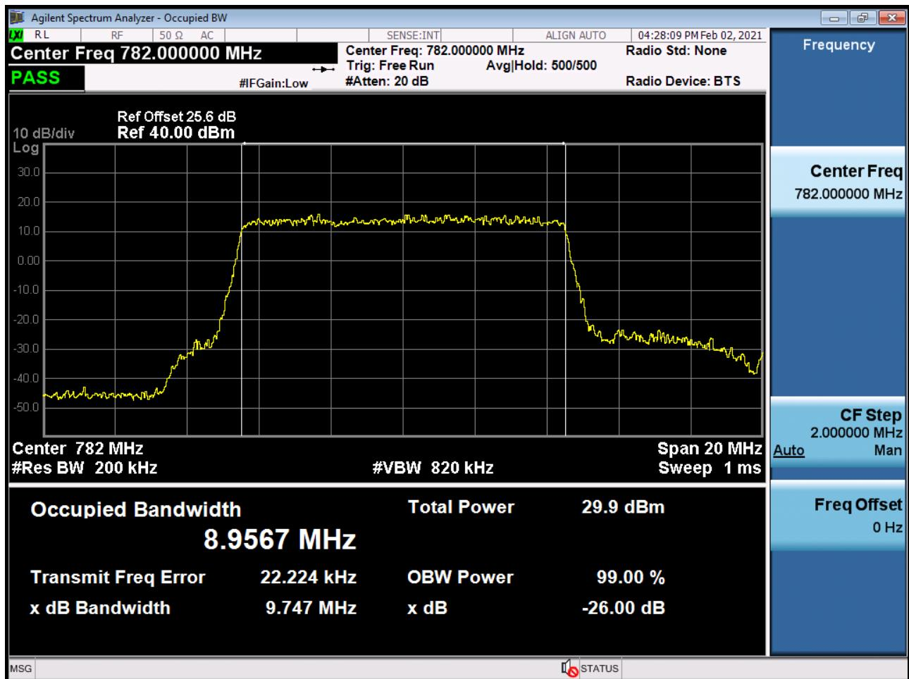
BAND 13. Occupied Bandwidth Plot (Ch.23230 64-QAM RB 50) 10 MHz
