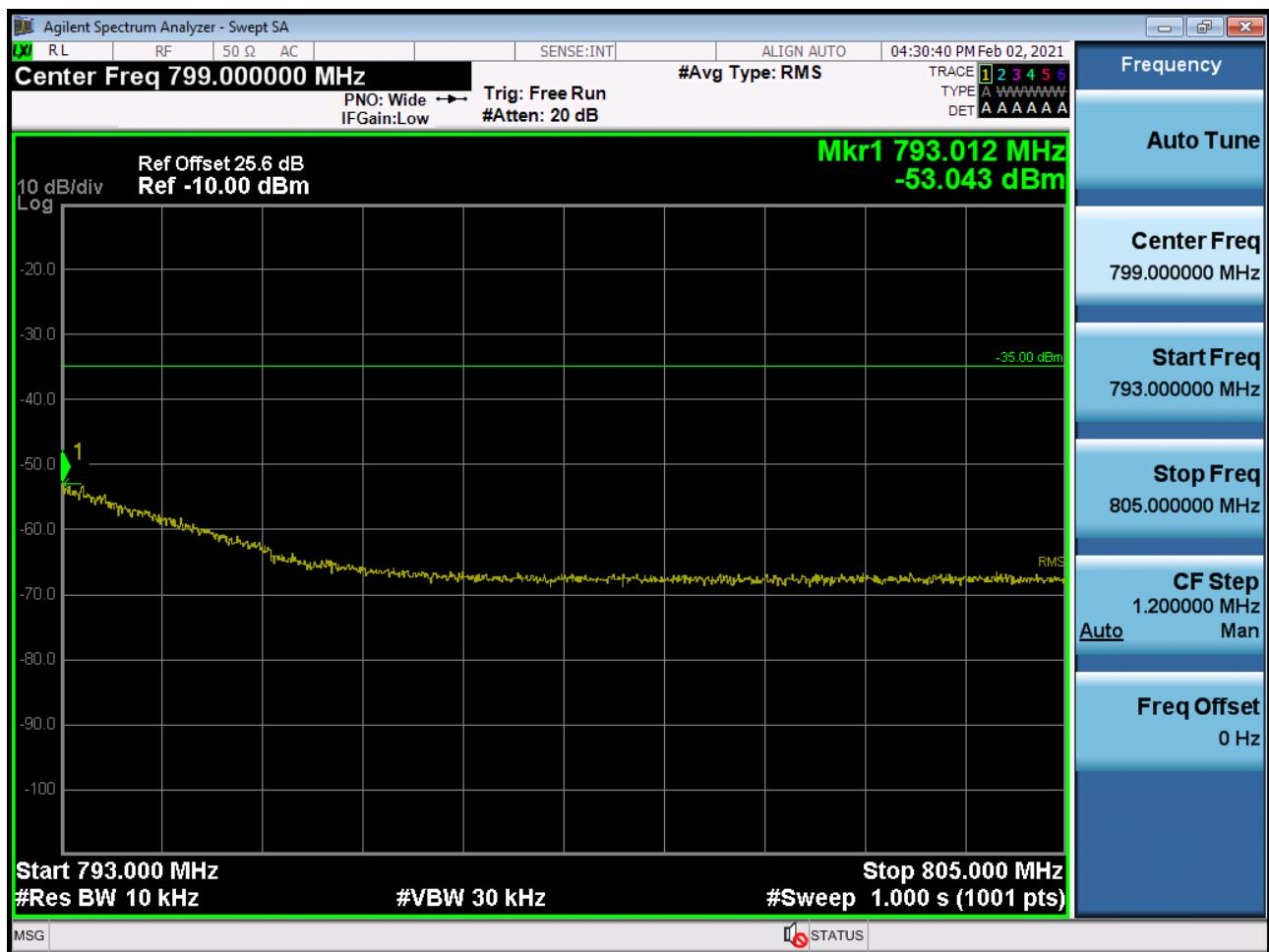
BAND 13. Conducted Spurious Plot (23205ch\_5MHz\_QPSK\_RB 1\_0)
