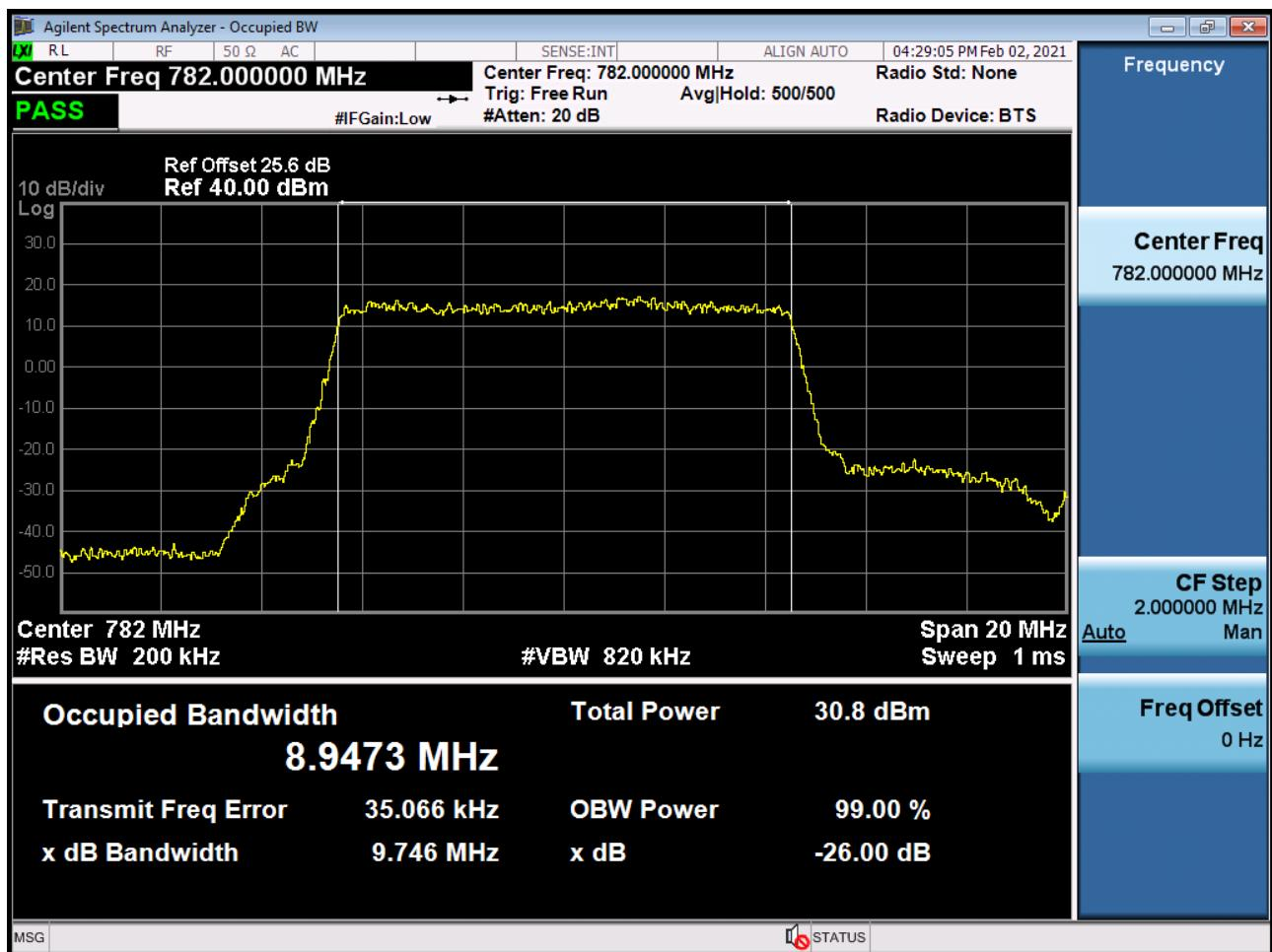
BAND 13. Occupied Bandwidth Plot (Ch.23230 16-QAM RB 50) 10 MHz
