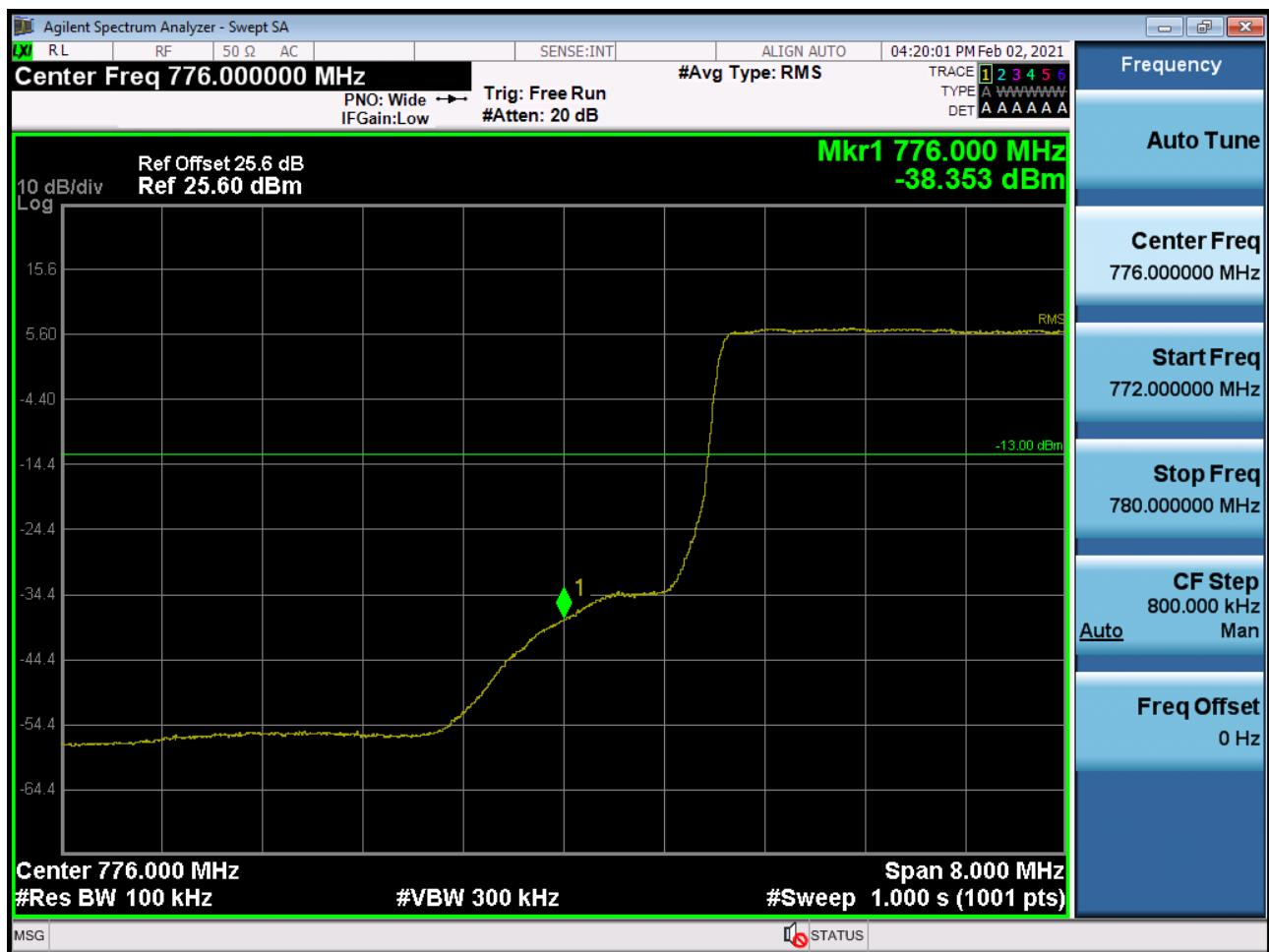
Band 13 Lower Emission Mask (763 MHz ~ 775 MHz) Plot (5M BW Ch.23205 QPSK\_RB25\_0)-2
