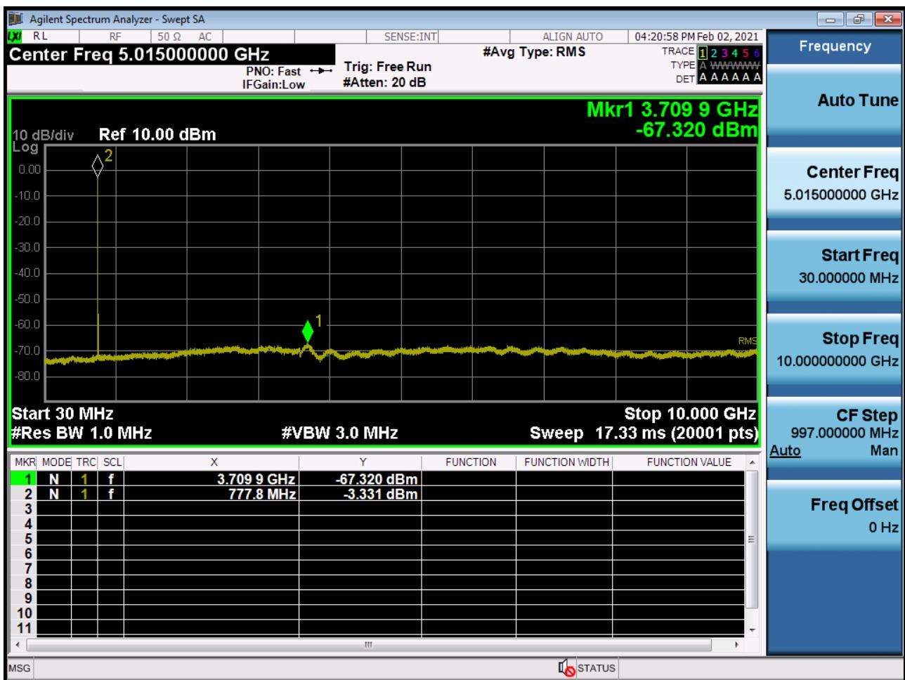
BAND 13. Conducted Spurious Plot (23230ch\_5MHz\_QPSK\_RB 1\_0)
