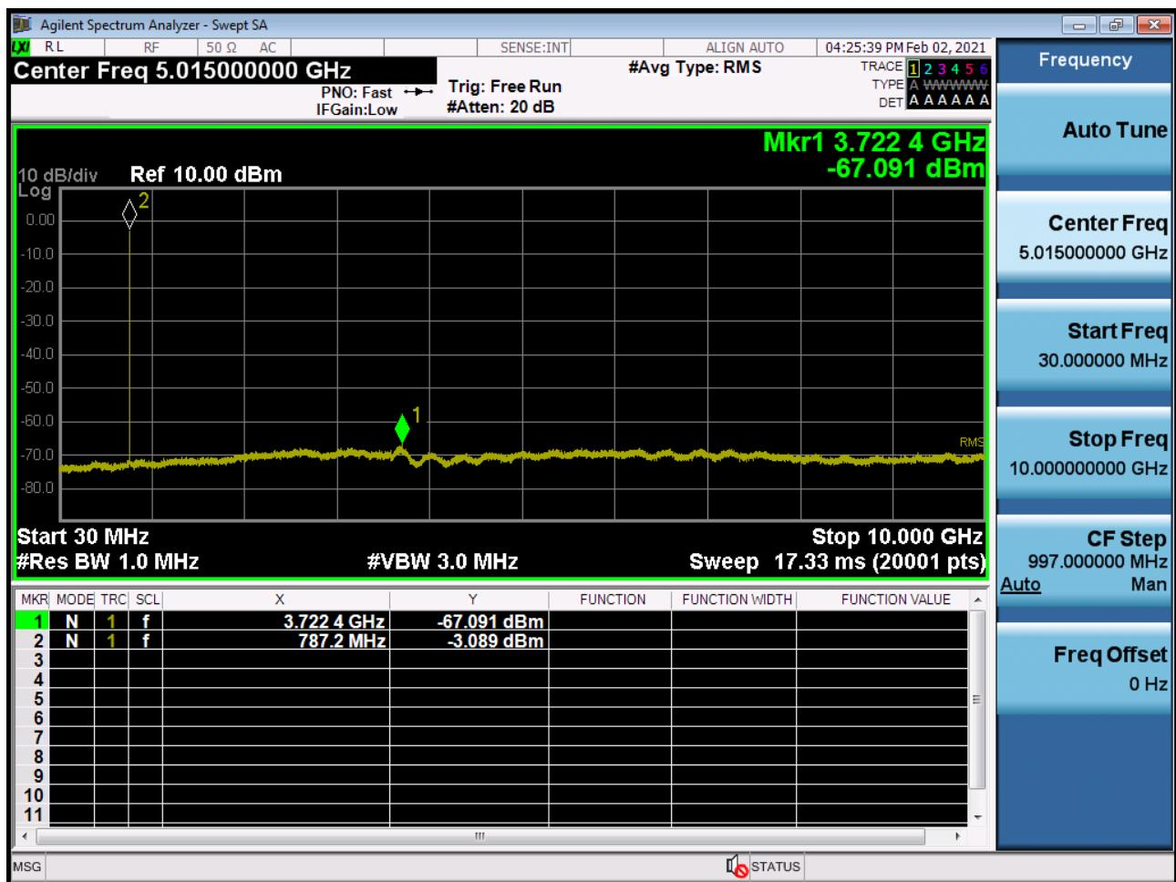
BAND 13. Conducted Spurious Plot (Ch.23230 10 MHz QPSK RB 1\_0)
