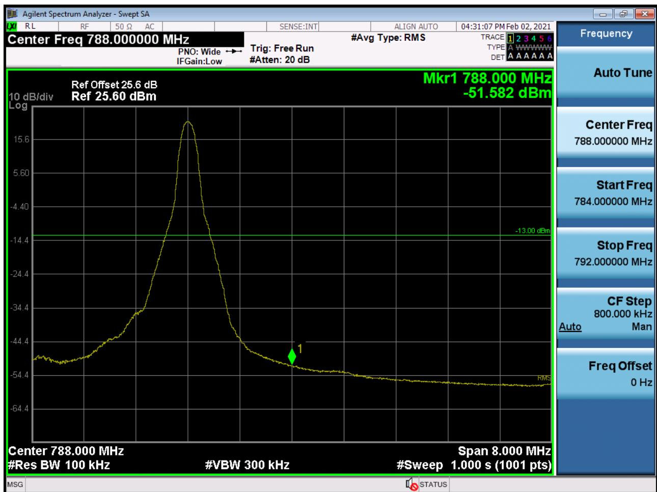
Band 13 Upper Band Edge Plot (10M BW Ch.23230 QPSK\_QPSK\_RB\_50\_0)-1
