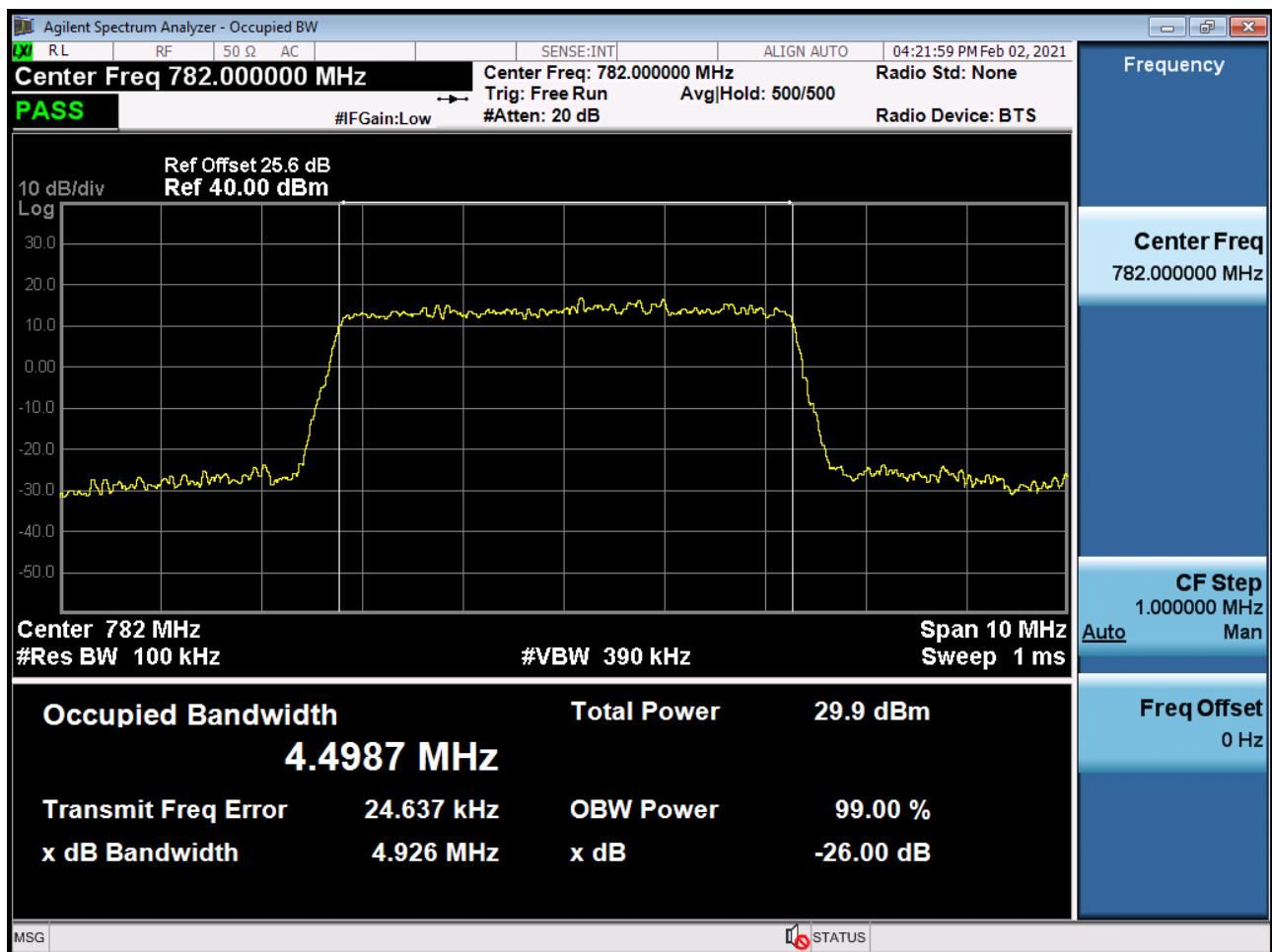
BAND 13. Occupied Bandwidth Plot (Ch.23230 64-QAM RB 25) 5 MHz
