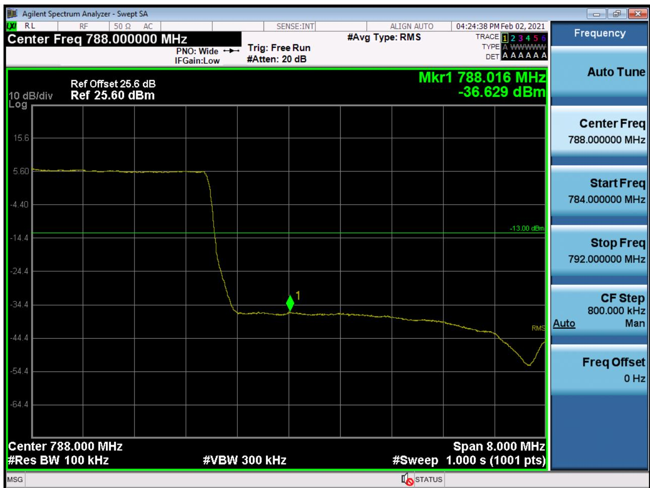
Band 13 Upper Emission Mask (793 MHz ~805 MHz) Plot (5M BW Ch.23255 QPSK\_RB25\_0)-2
