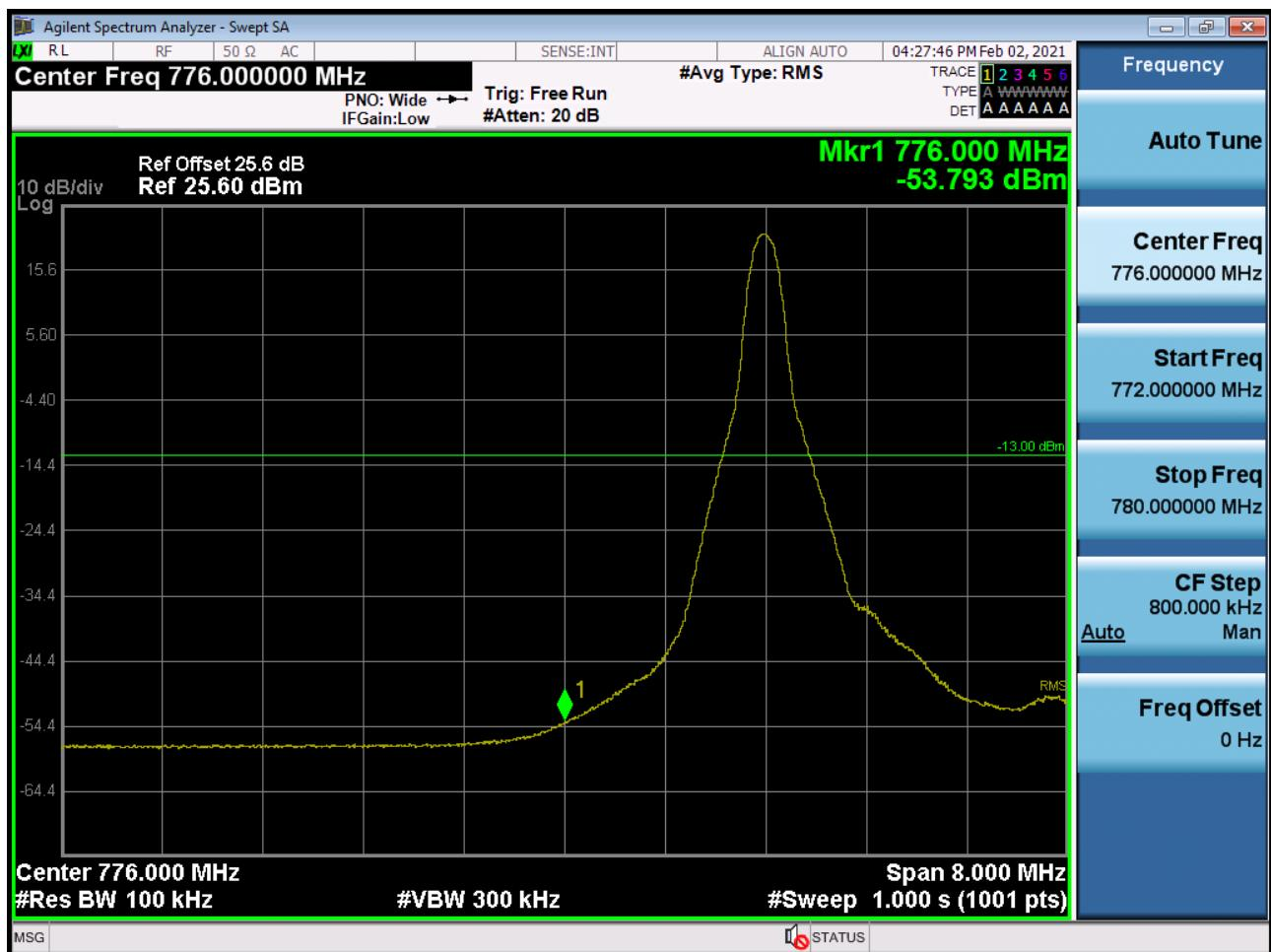
BAND 13. Lower & Upper Band Edge Plot (10M BW Ch.23230 QPSK RB\_50\_0)-1
