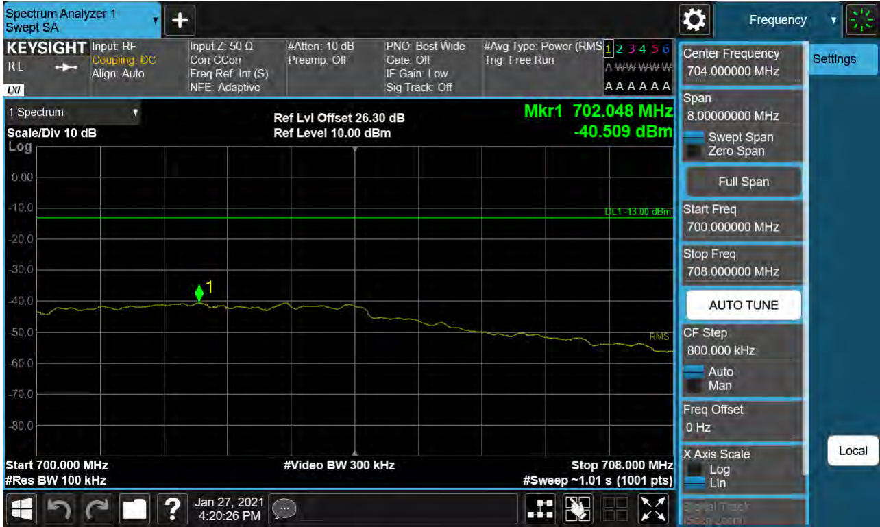
Sub6 n71. Upper Extended Band Edge Plot (10M BW Ch.138600 BPSK_RB52_0)
