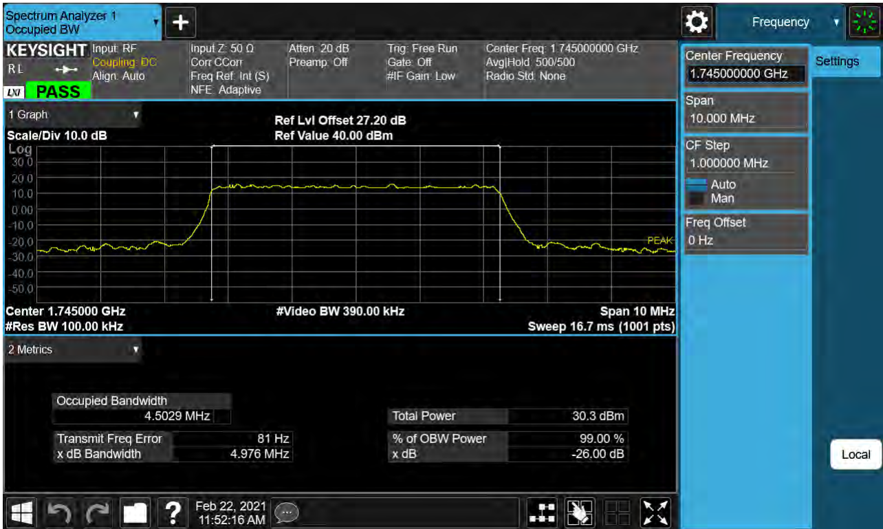
Sub6 n66. Occupied Bandwidth Plot (5M BW Ch.349000 64QAM RB 25)
