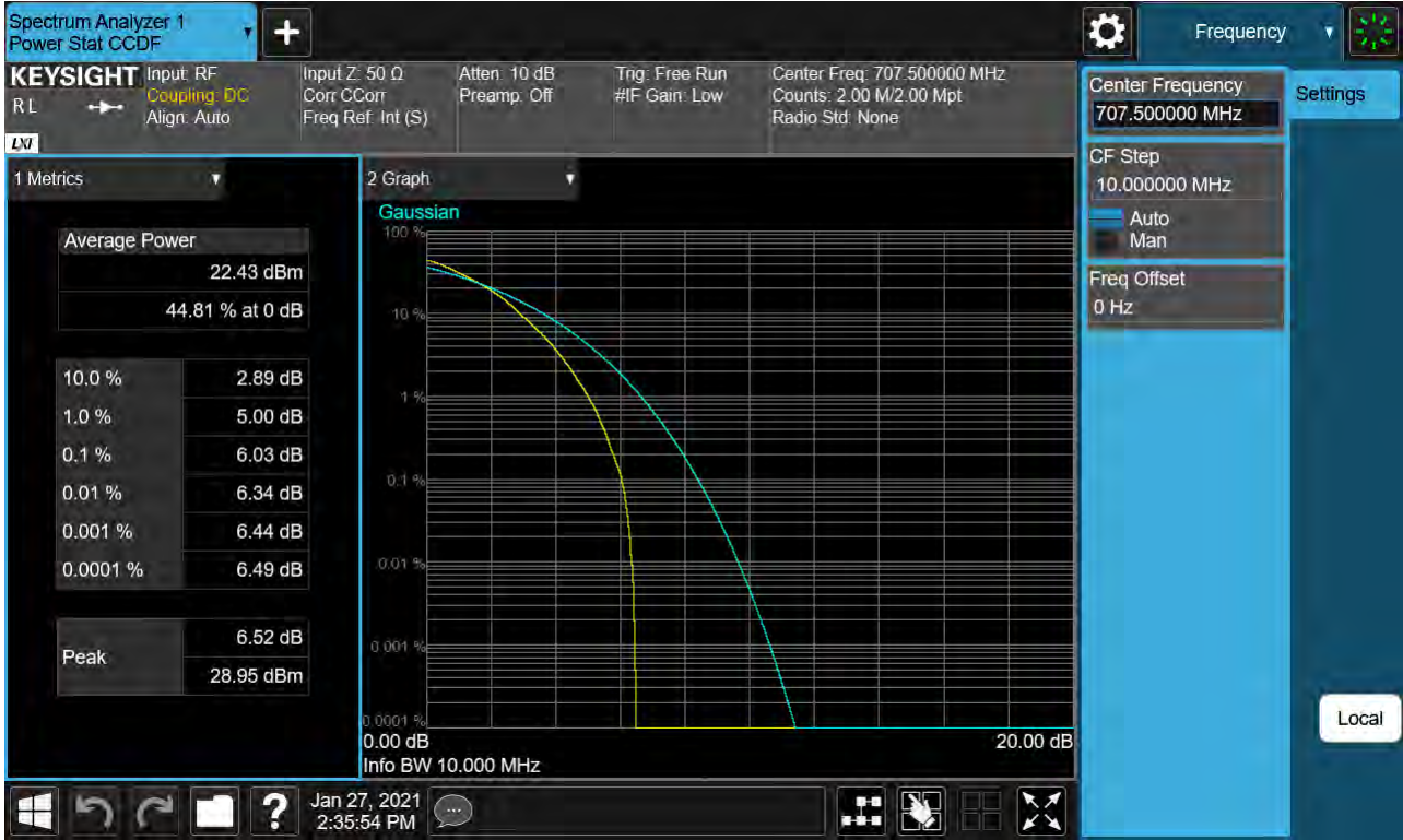
Sub6 n12. PAR Plot (10M BW Ch.141500 64QAM_RB52_0)
