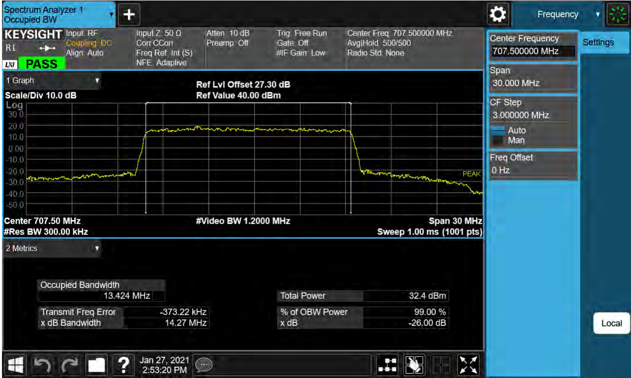
Sub6 n12. Occupied Bandwidth Plot (15M BW Ch.141500 BPSK_RB79_0)
