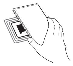
Ensure that the device's screen is turned on and unlocked. Otherwise, the device will not read NFC tags or receive data.
