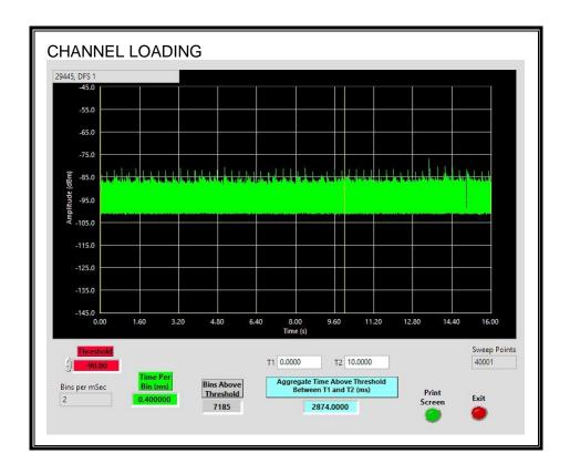
The level of traffic loading on the channel by the EUT is 28.74%
