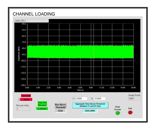
The level of traffic loading on the channel by the EUT is 18.26%
