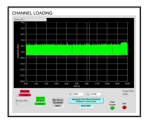
The level of traffic loading on the channel by the EUT is 40.2%
