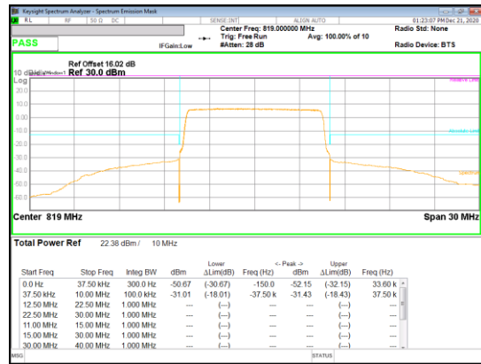
16QAM Mid channel FRB
