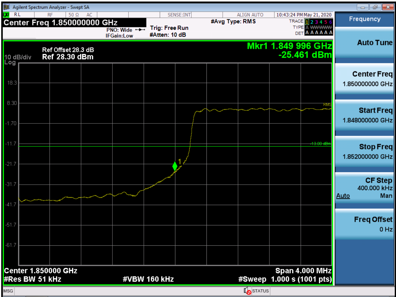
Sub6 n2. Lower Band Edge Plot (5M BW Ch.370500 BPSK_RB25_Offset 0) -2
