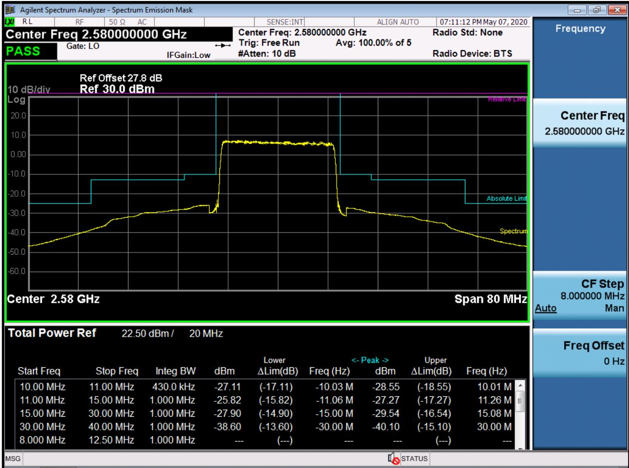
BAND 38. Mid Channel Edge Plot (20 MHz Ch.38000 QPSK RB 100)
