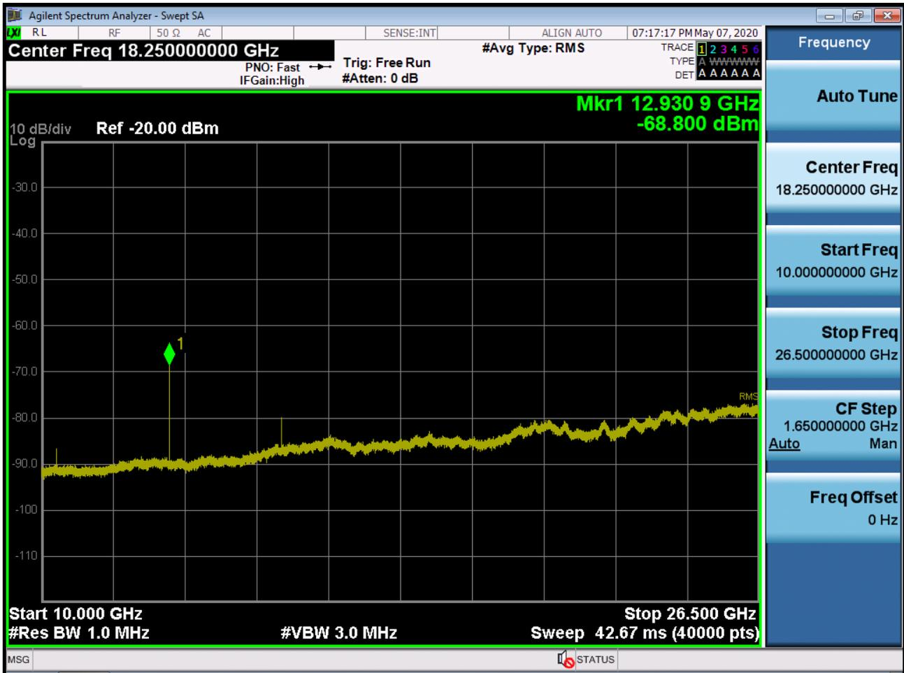
BAND 38. Conducted Spurious Plot 1 (20 MHz Ch.38150 QPSK RB 1, Offset 0)
