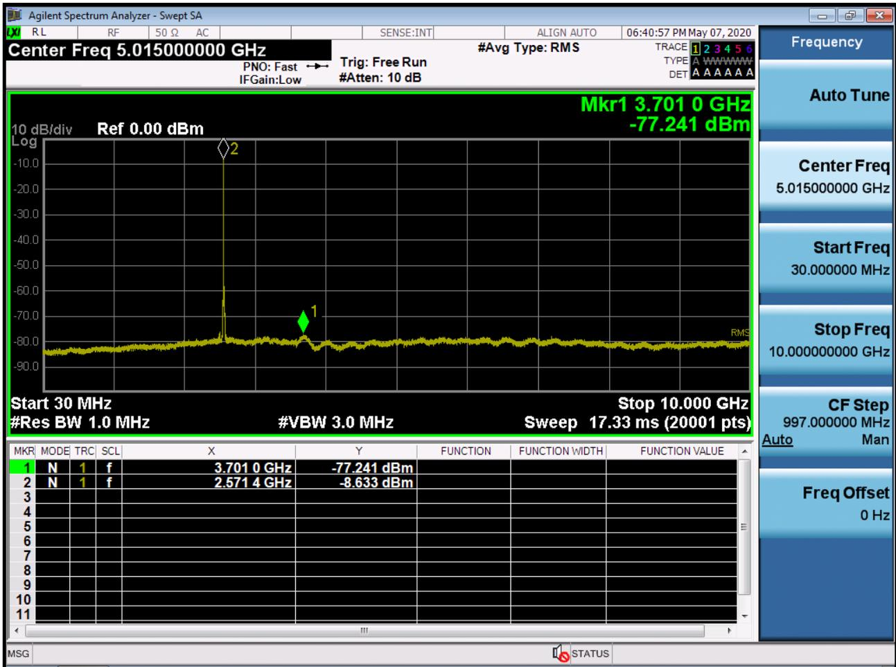
BAND 38. Conducted Spurious Plot 2 (10 MHz Ch. 37800 QPSK RB 1, Offset 0)
