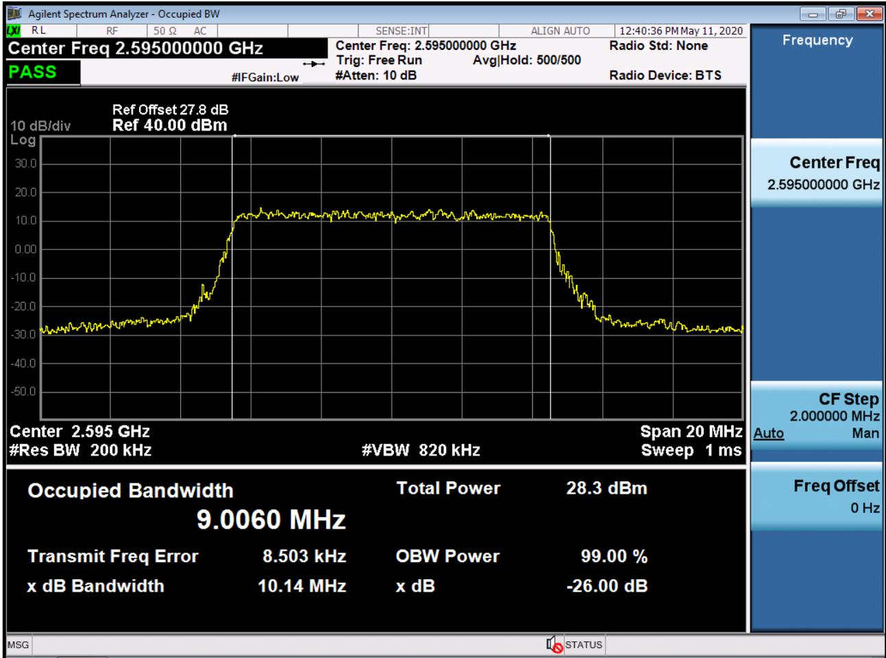
BAND 38. Occupied Bandwidth Plot (15 MHz Ch.38000 QPSK RB 75)
