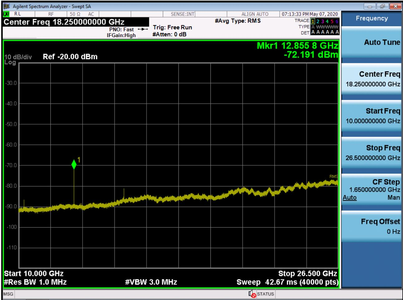
BAND 38. Conducted Spurious Plot 1 (20 MHz Ch.38000 QPSK RB 1, Offset 0)
