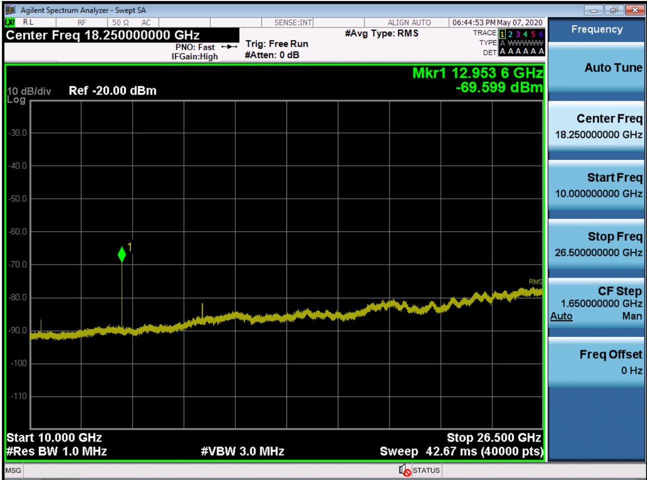
BAND 38. Conducted Spurious Plot 1 (10 MHz Ch. 38200 QPSK RB 1, Offset 0)
