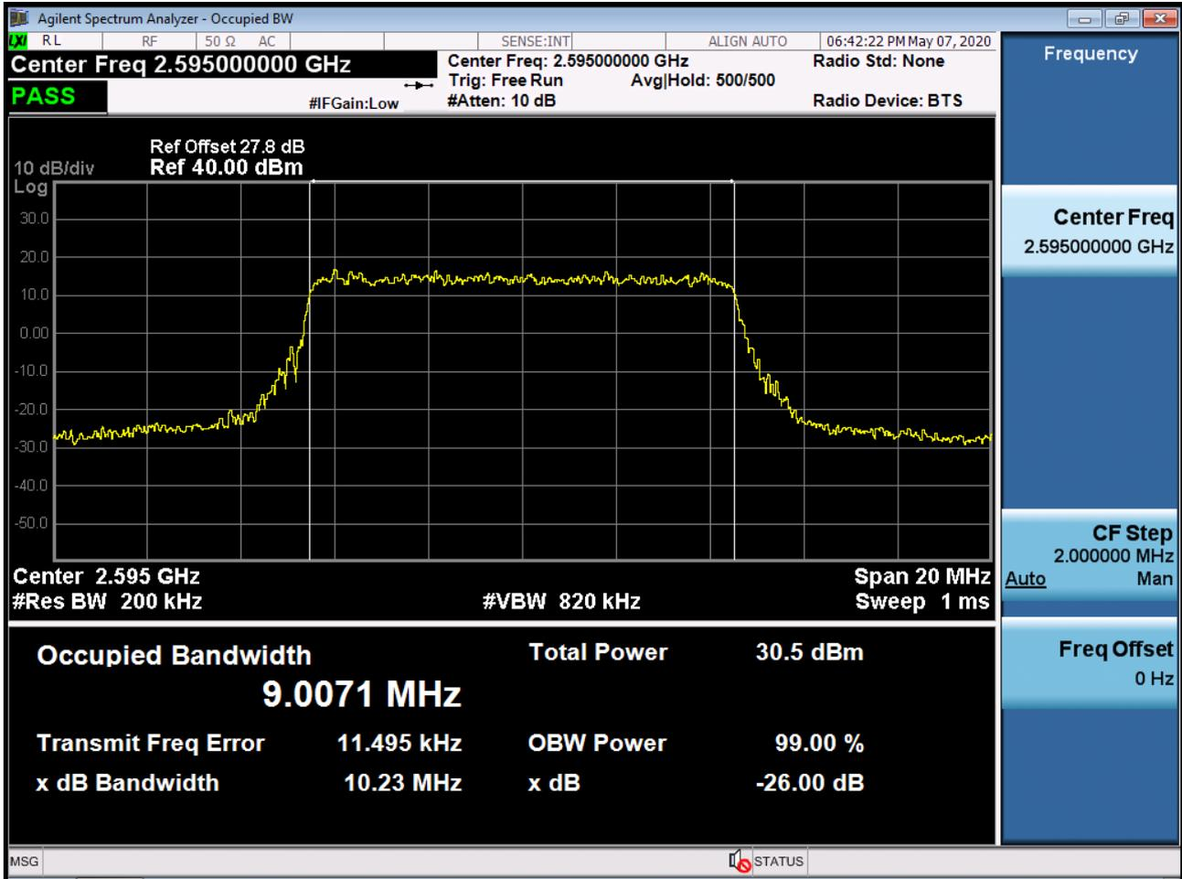
BAND 38. Occupied Bandwidth Plot (10 MHz Ch.38000 16-QAM RB 50)
