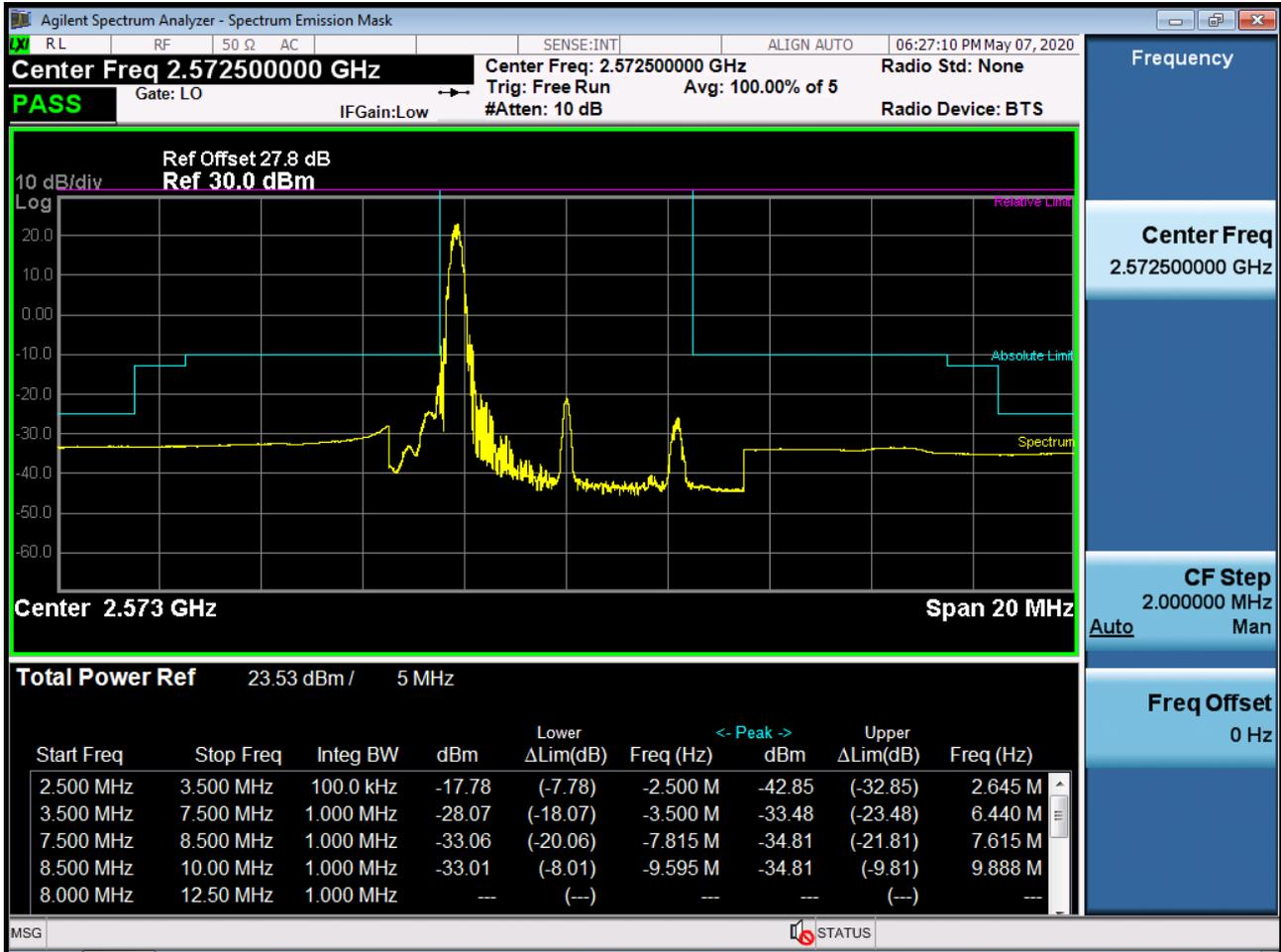
BAND 38. Low Channel Edge Plot (5 MHz Ch.37775 QPSK RB 25, Offset 0)
