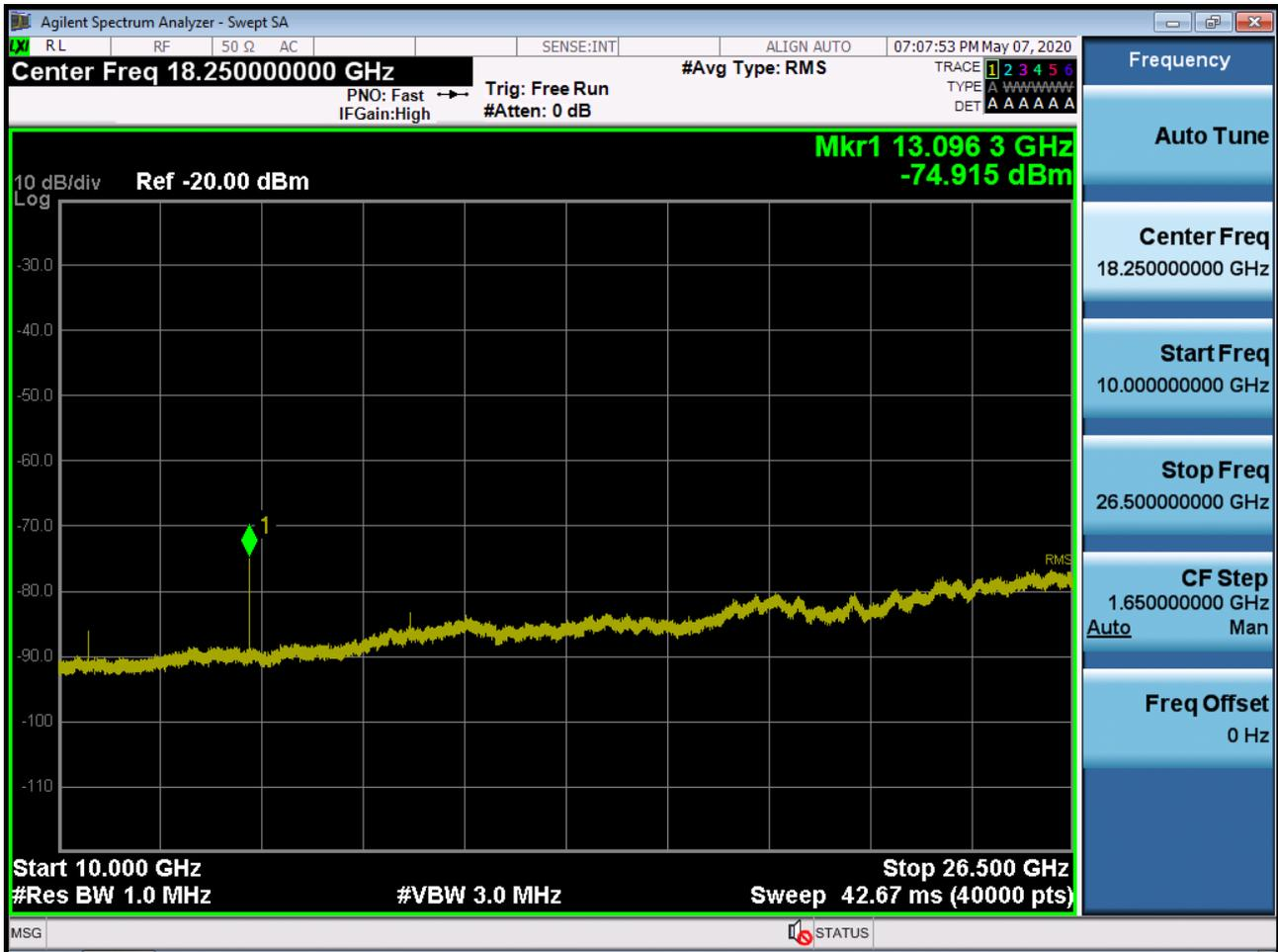
BAND 38. Conducted Spurious Plot 1 (20 MHz Ch.37850 QPSK RB 1, Offset 0)
