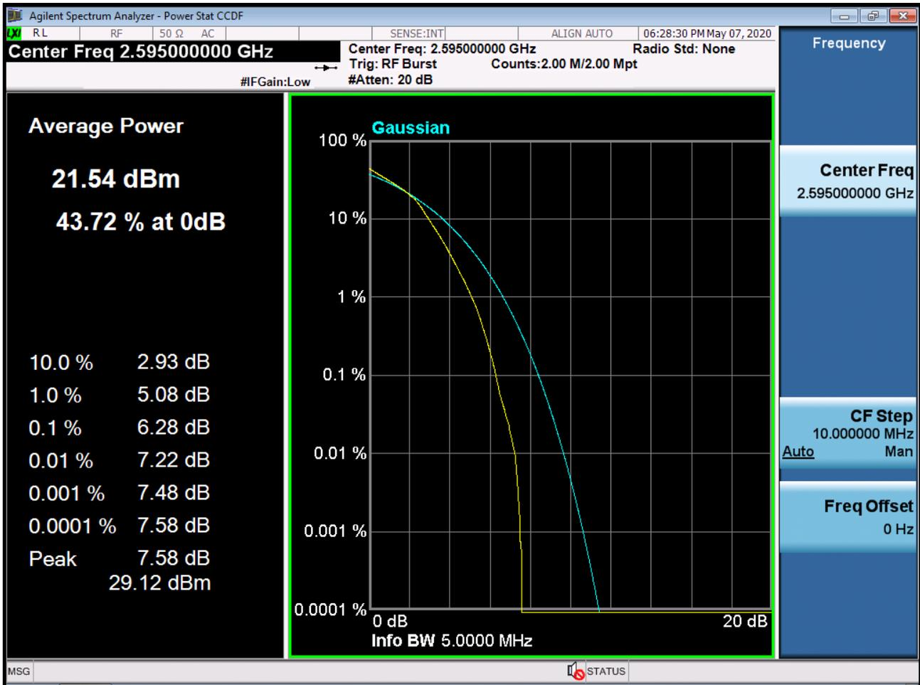
BAND 38. PAR Plot (5M BW\_Ch.38000\_64QAM\_RB25\_0)
