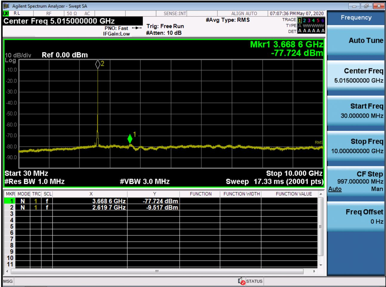
BAND 38. Conducted Spurious Plot 2 (15 MHz Ch. 38175 QPSK RB 1, Offset 0)
