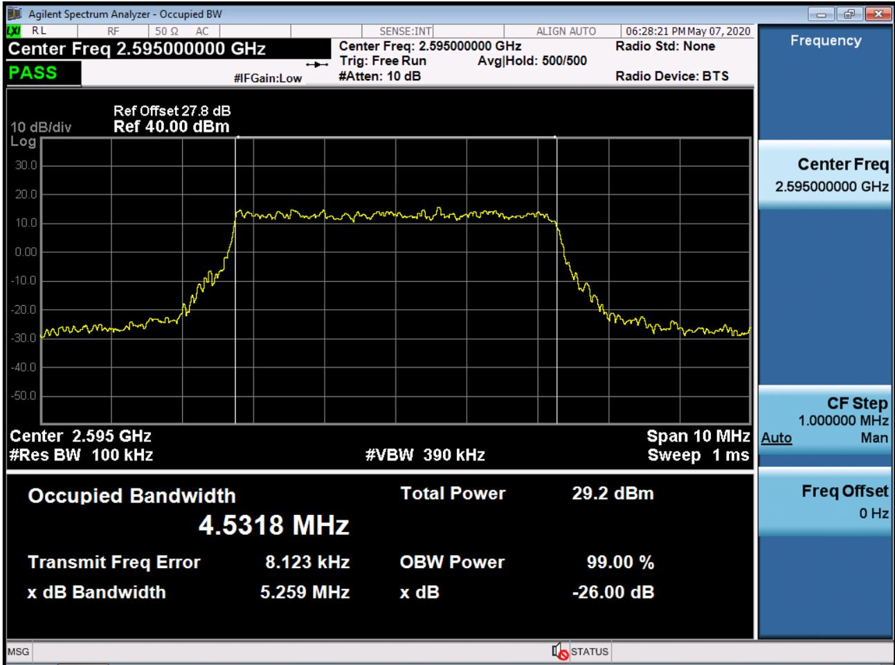
BAND 38. Occupied Bandwidth Plot (5 MHz Ch.38000 64-QAM RB 25)
