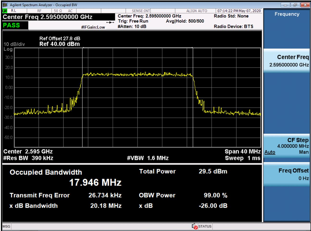
BAND 38. Occupied Bandwidth Plot (20 MHz Ch.38000 64-QAM RB 100)
