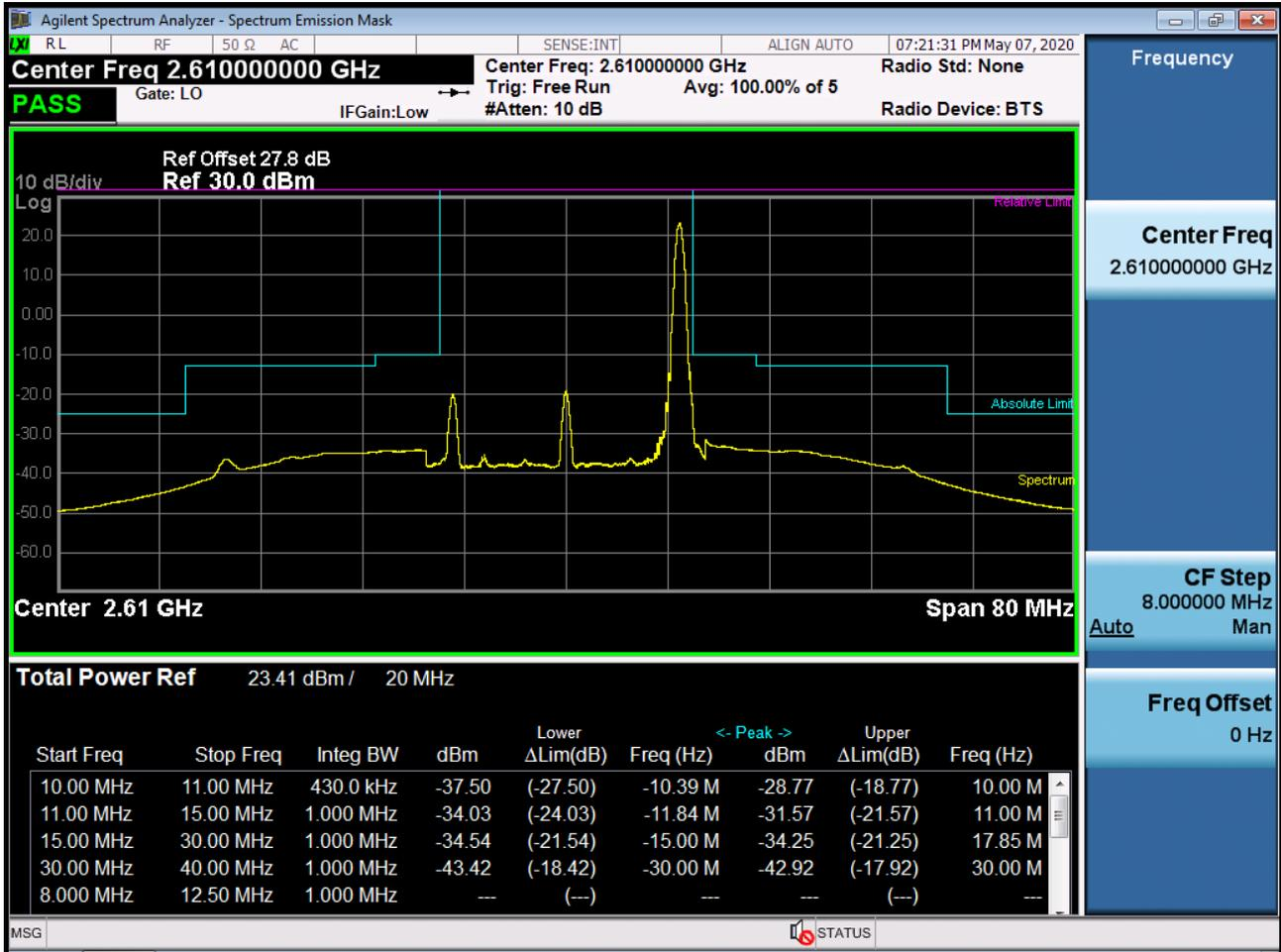
BAND 38. High Channel Edge Plot (20 MHz Ch.38150 QPSK\_RB100\_Offset 0)
