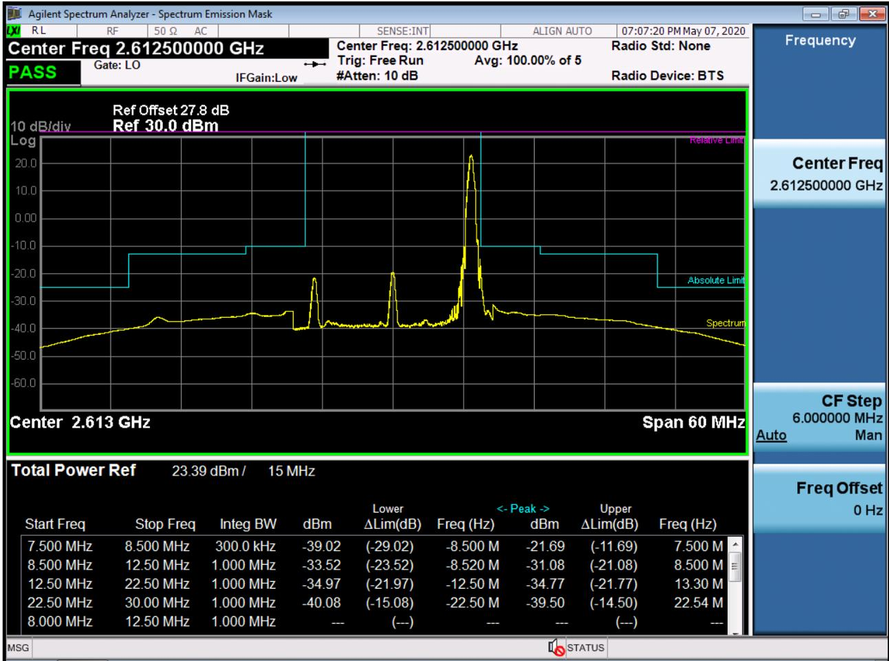
BAND 38. High Channel Edge Plot (15 MHz Ch.38175 QPSK\_RB75\_Offset 0)
