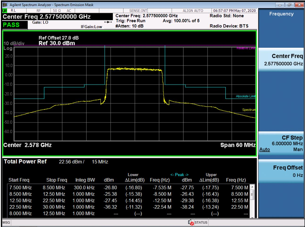
BAND 38. Mid Channel Edge Plot (15 MHz Ch.38000 QPSK RB 75)
