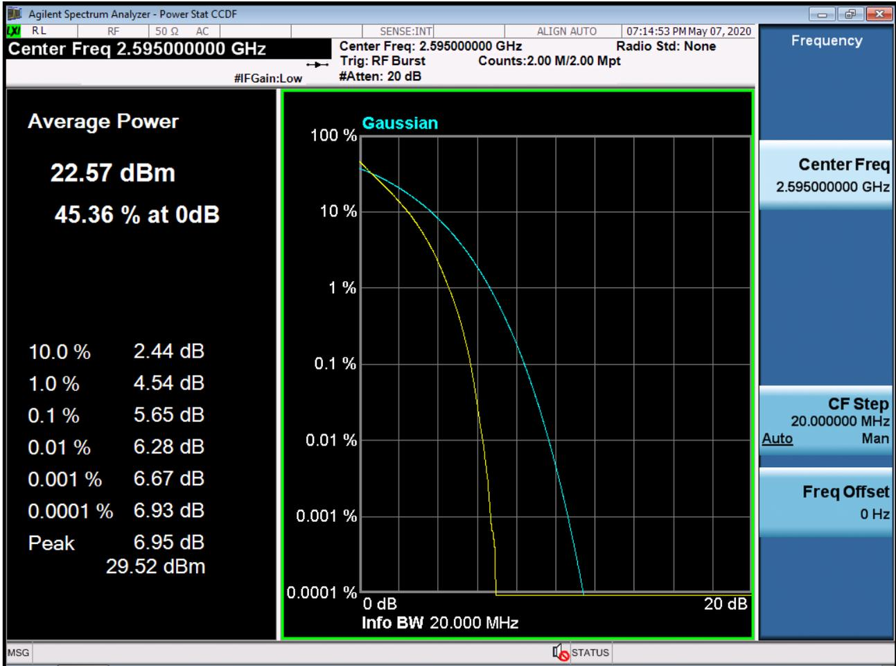
BAND 38. PAR Plot (20M BW\_Ch.38000\_16QAM\_RB100\_0)
