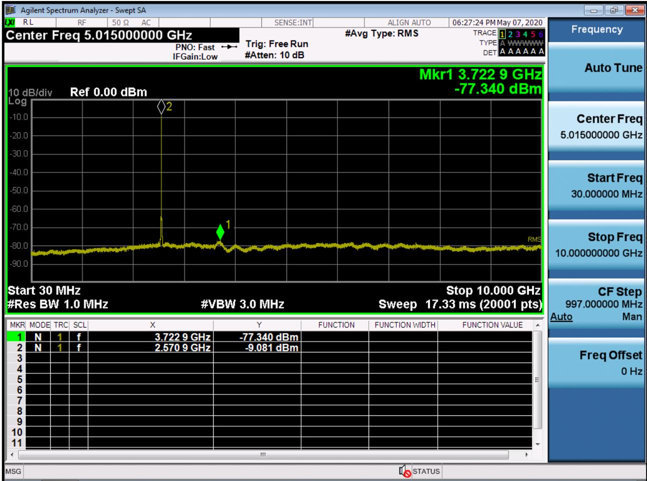
BAND 38. Conducted Spurious Plot 2 (5 MHz Ch. 37775 QPSK RB 1, Offset 0)
