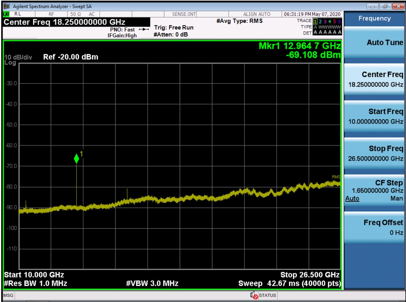
BAND 38. Conducted Spurious Plot 1 (5 MHz Ch.38225 QPSK RB 1, Offset 0)
