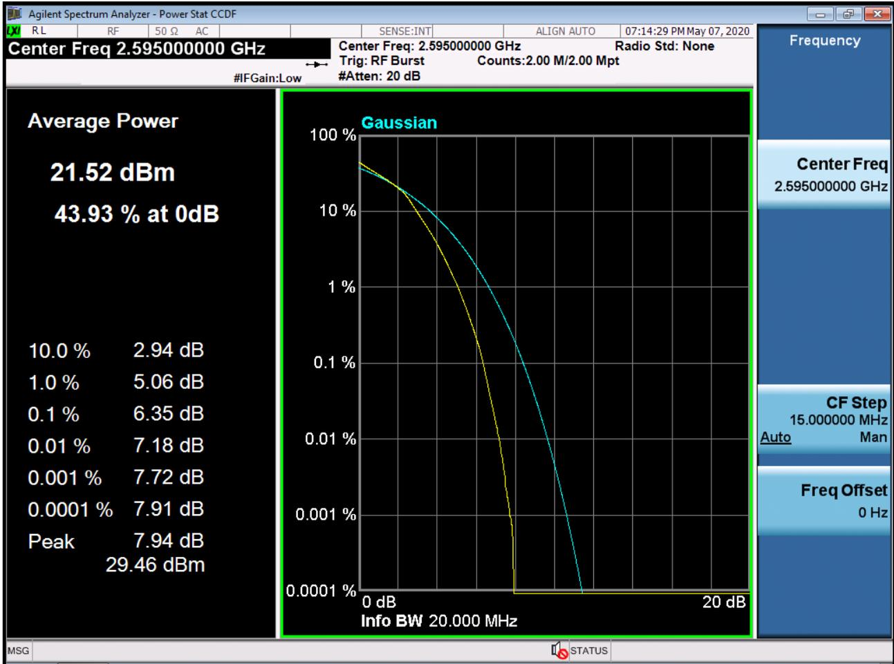
BAND 38. PAR Plot (20M BW\_Ch.38000\_64QAM\_RB100\_0)
