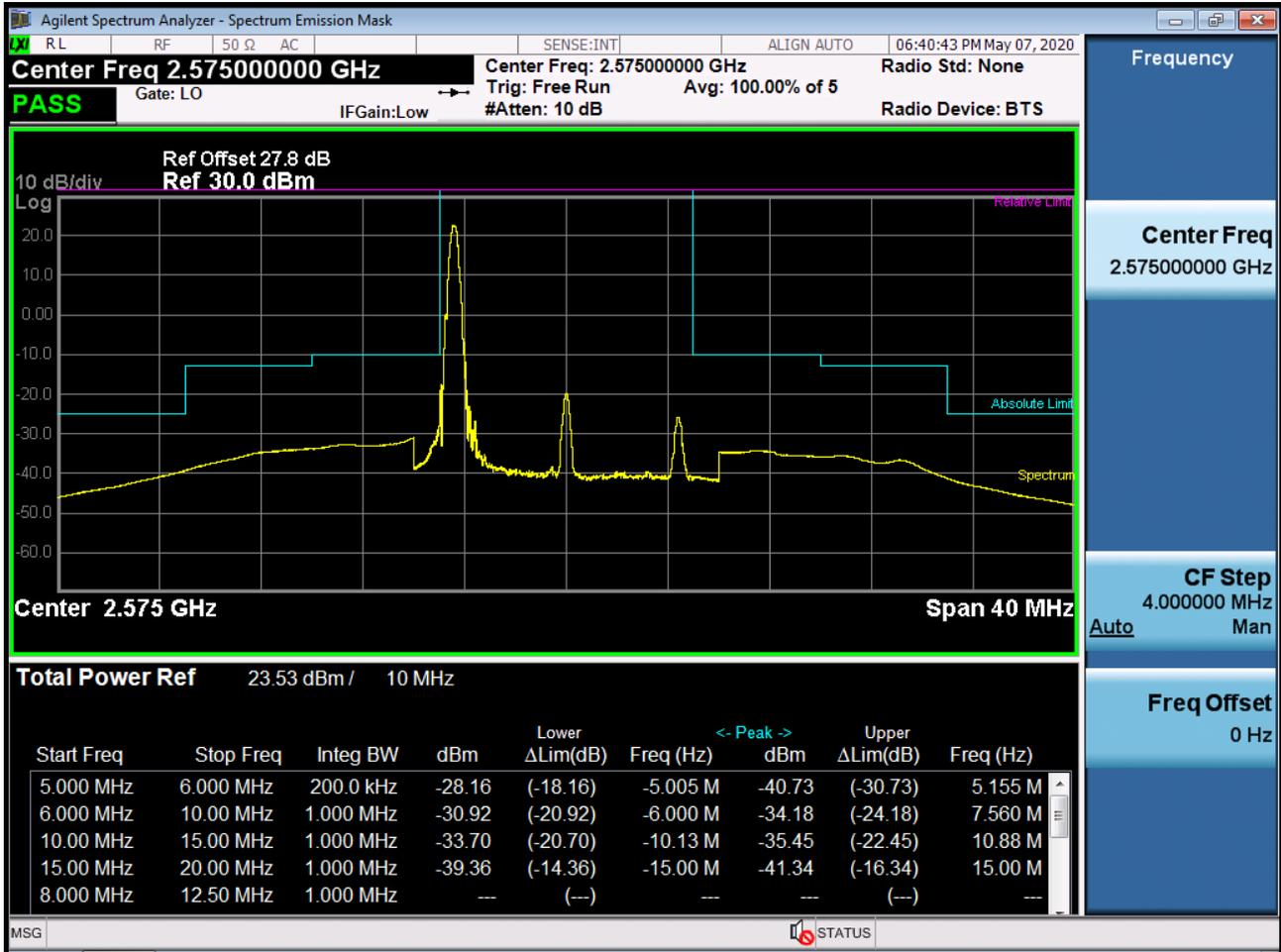
BAND 38. Low Channel Edge Plot (10 MHz Ch.37800 QPSK RB 25, Offset 0)
