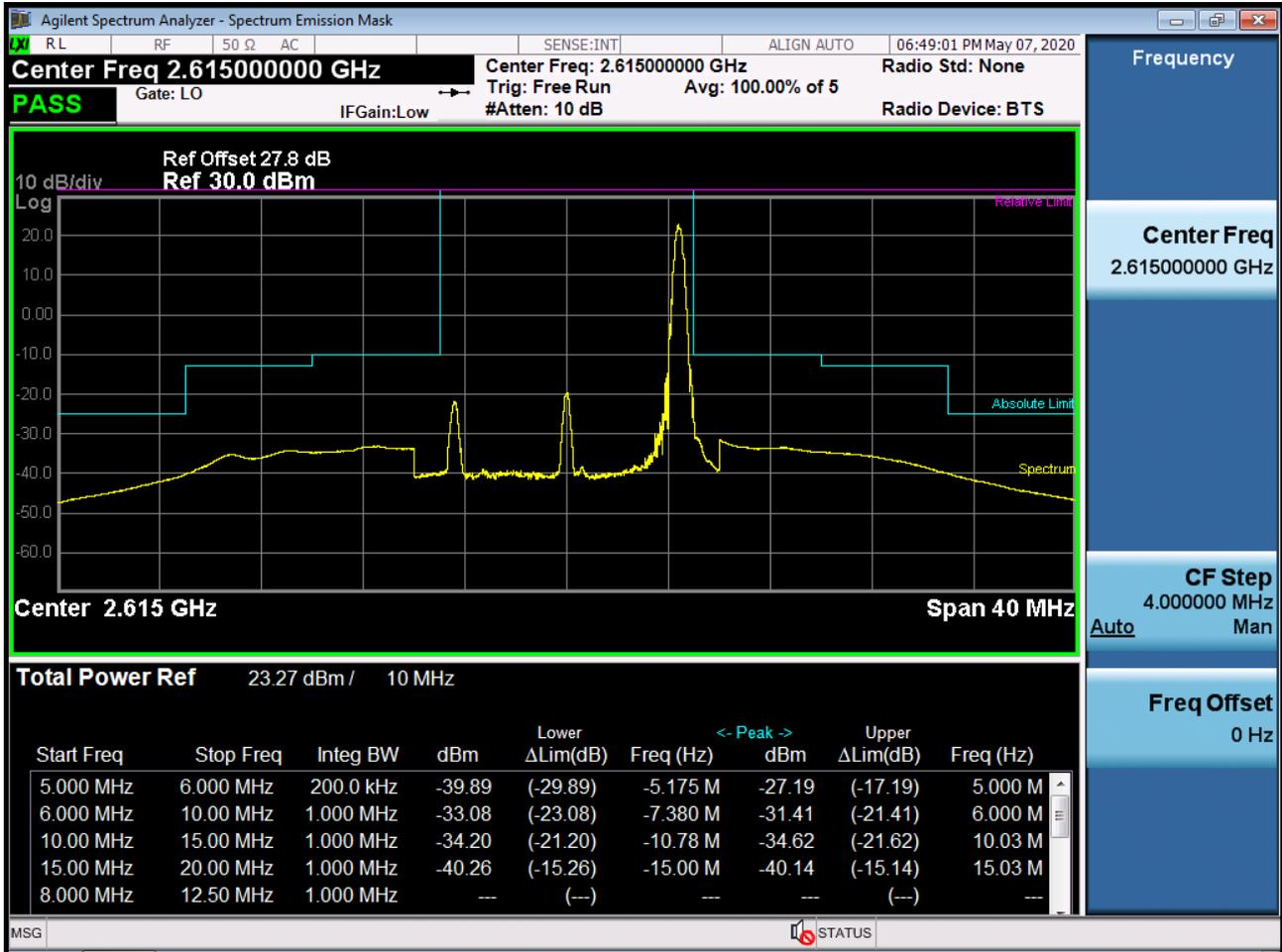
BAND 38. High Channel Edge Plot (10 MHz Ch.38200 QPSK\_RB50\_Offset 0)
