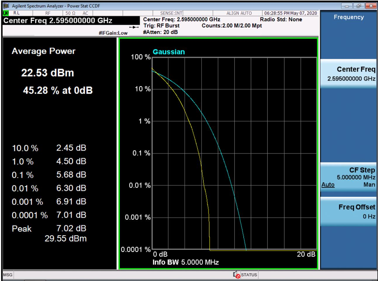
BAND 38. PAR Plot (5M BW\_Ch.38000\_16QAM\_RB25\_0)
