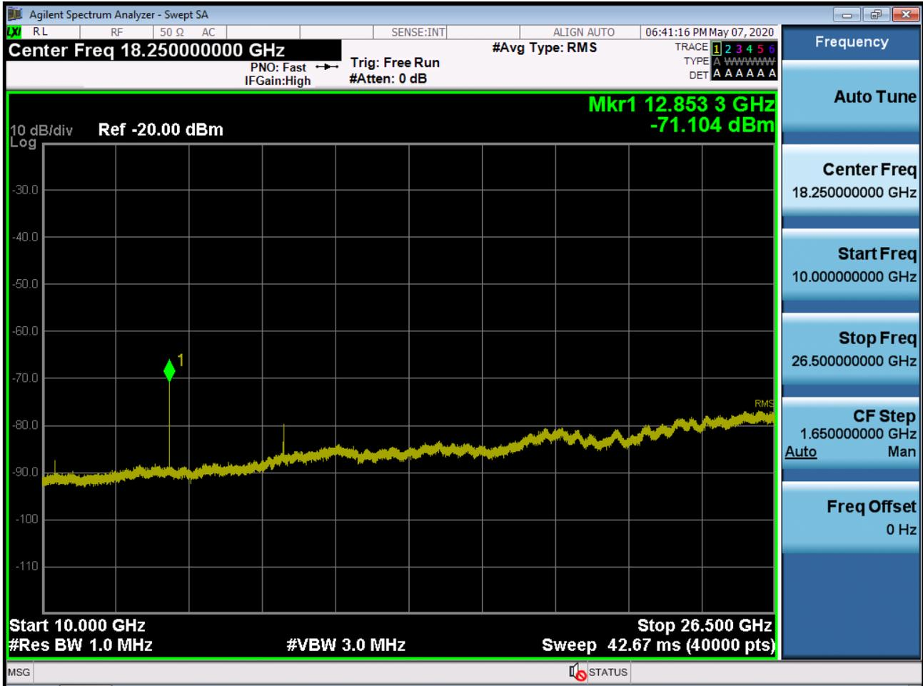
BAND 38. Conducted Spurious Plot 1 (10 MHz Ch.38000 QPSK RB 1, Offset 0)
