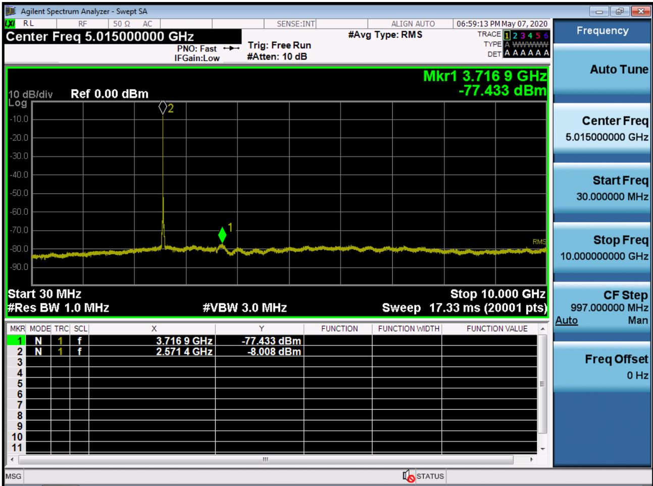
BAND 38. Conducted Spurious Plot 2 (15 MHz Ch. 37825 QPSK RB 1, Offset 0)
