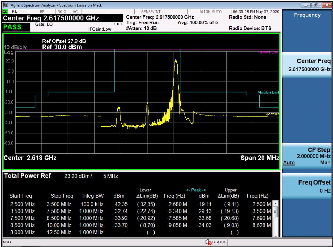
BAND 38. High Channel Edge Plot (5 MHz Ch.38225 QPSK\_RB25\_Offset 0)
