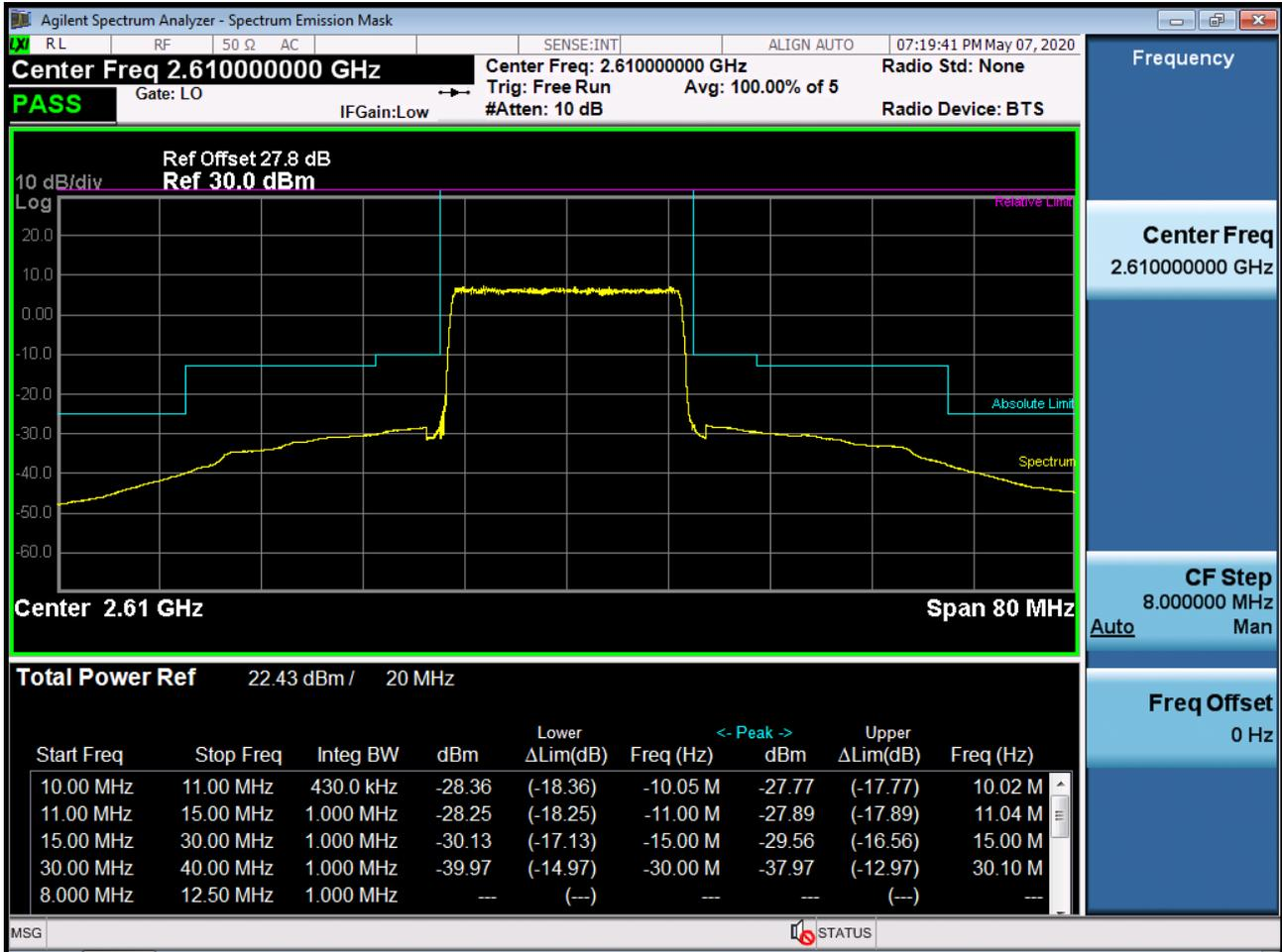
BAND 38. Conducted Spurious Plot 1 (5 MHz Ch.3775 QPSK RB 1, Offset 0)
