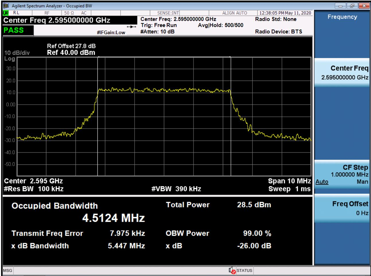
BAND 38. Occupied Bandwidth Plot (10 MHz Ch.38000 QPSK RB 50)
