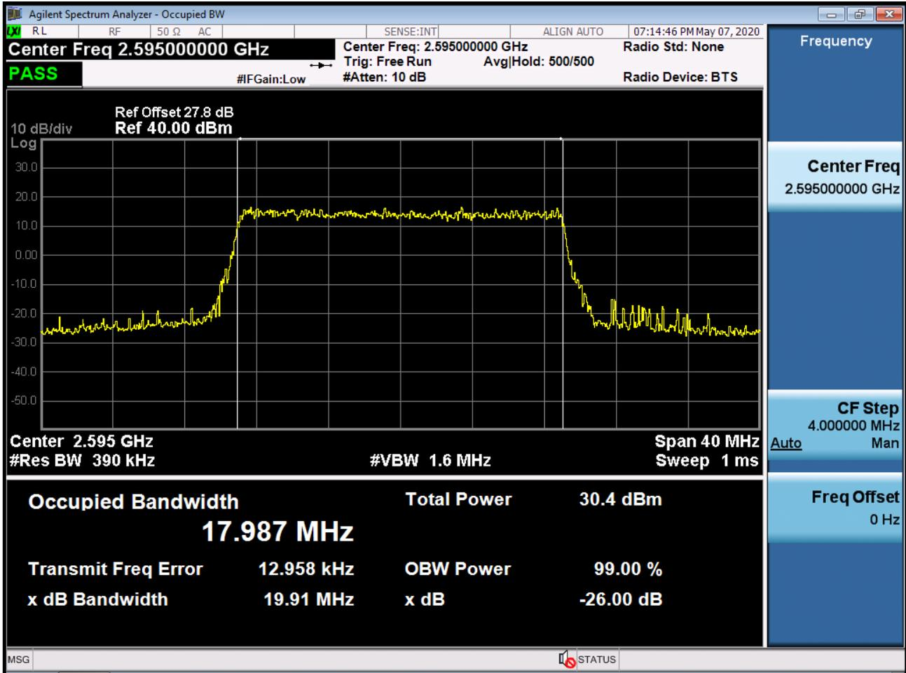
BAND 38. Occupied Bandwidth Plot (20 MHz Ch.38000 16-QAM RB 100)
