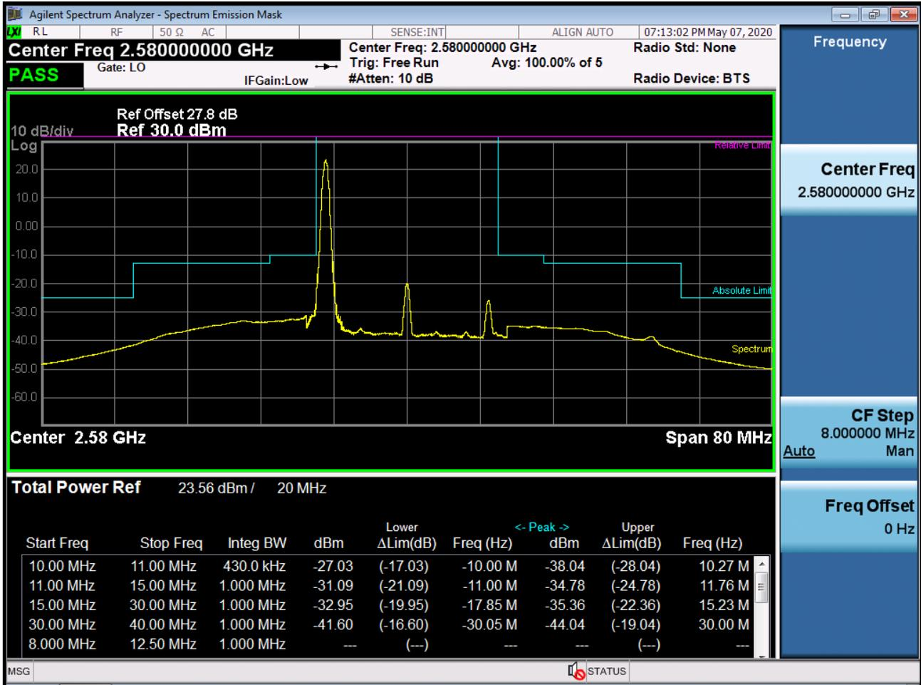
BAND 38. Low Channel Edge Plot (20 MHz Ch.37850 QPSK RB 25, Offset 0)
