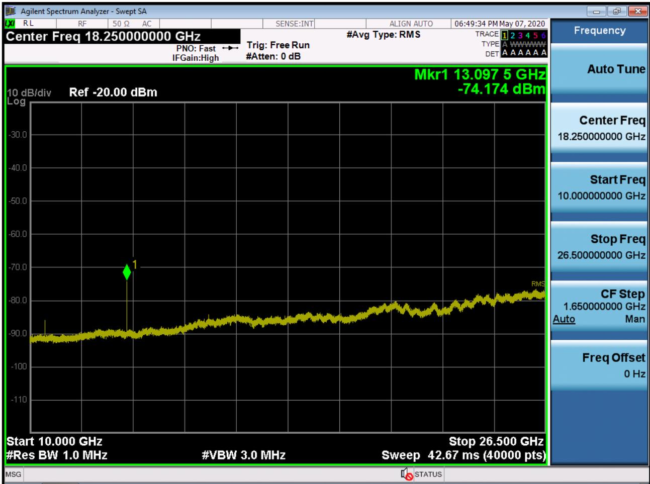
BAND 38. Conducted Spurious Plot 1 (15 MHz Ch.37825 QPSK RB 1, Offset 0)
