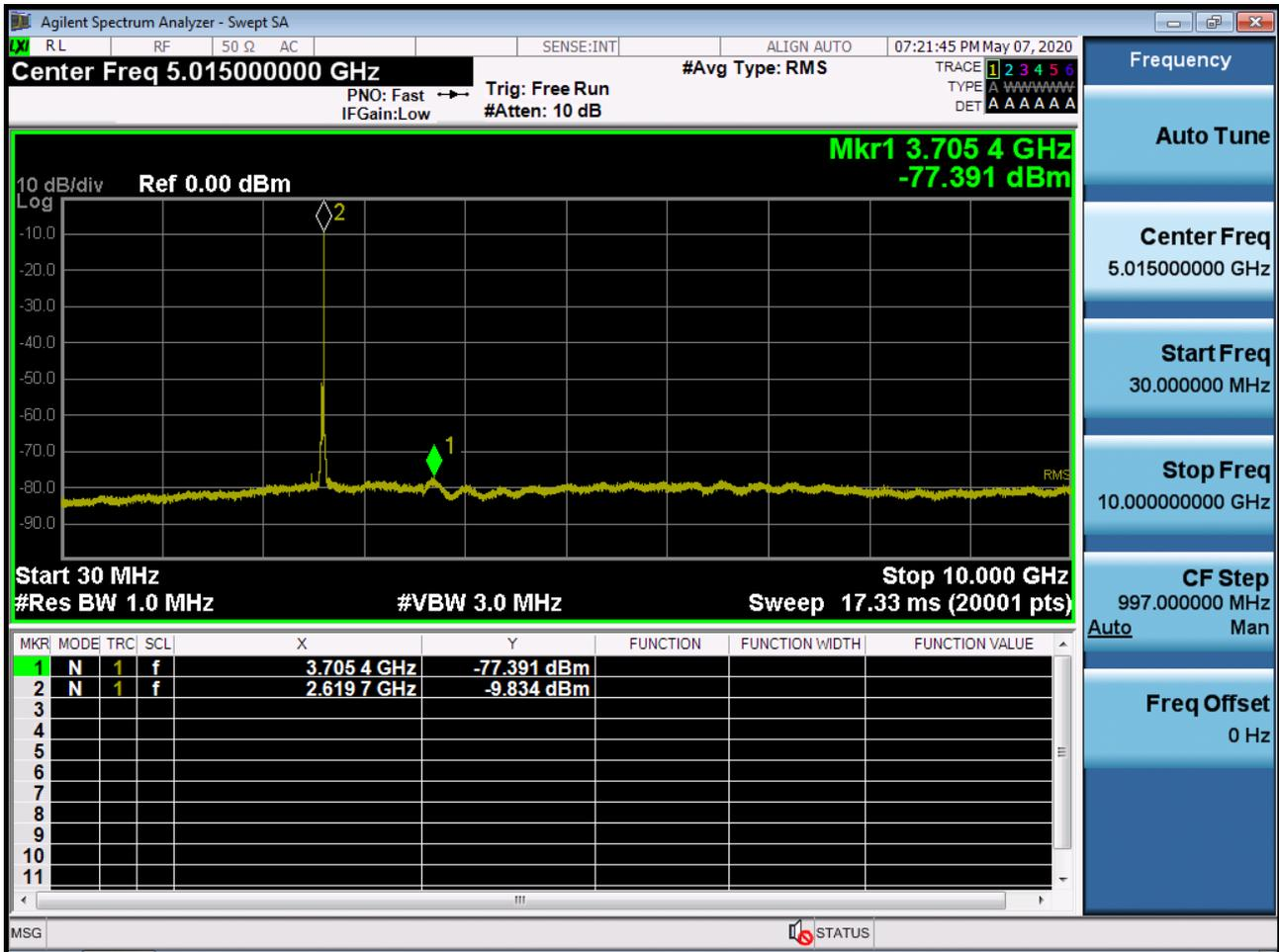
BAND 38. Conducted Spurious Plot 2 (20 MHz Ch. 38150 QPSK RB 1, Offset 0)
