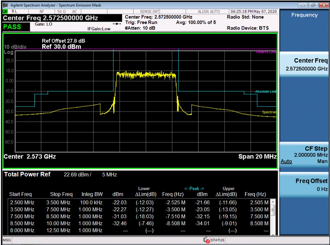
BAND 38. Mid Channel Edge Plot (5 MHz Ch.38000 QPSK RB 25)
