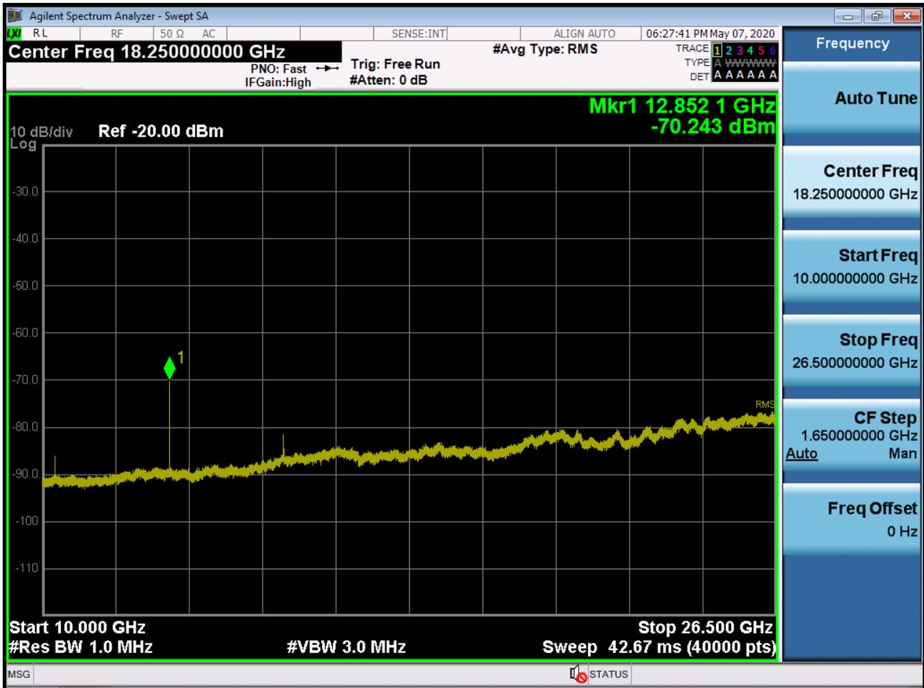
BAND 38. Conducted Spurious Plot 1 (5 MHz Ch.38000 QPSK RB 1, Offset 0)
