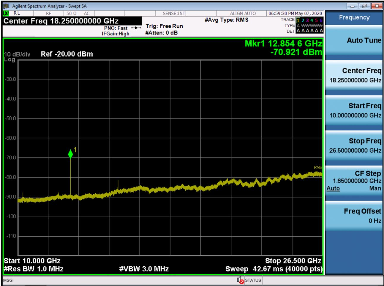
BAND 38. Conducted Spurious Plot 1 (15 MHz Ch.38000 QPSK RB 1, Offset 0)
