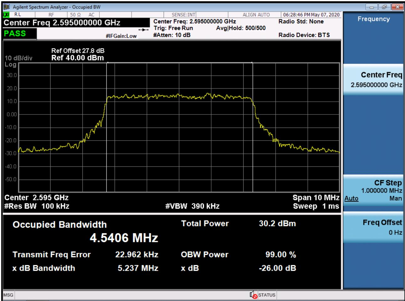
BAND 38. Occupied Bandwidth Plot (5 MHz Ch.38000 16-QAM RB 25)
