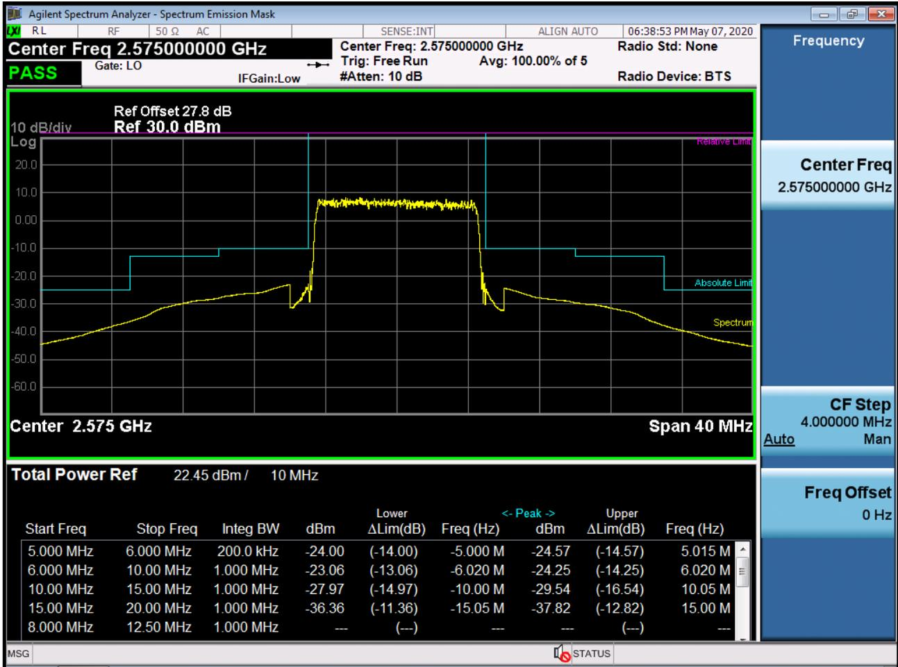
BAND 38. Mid Channel Edge Plot (10 MHz Ch.38000 QPSK RB 50)
