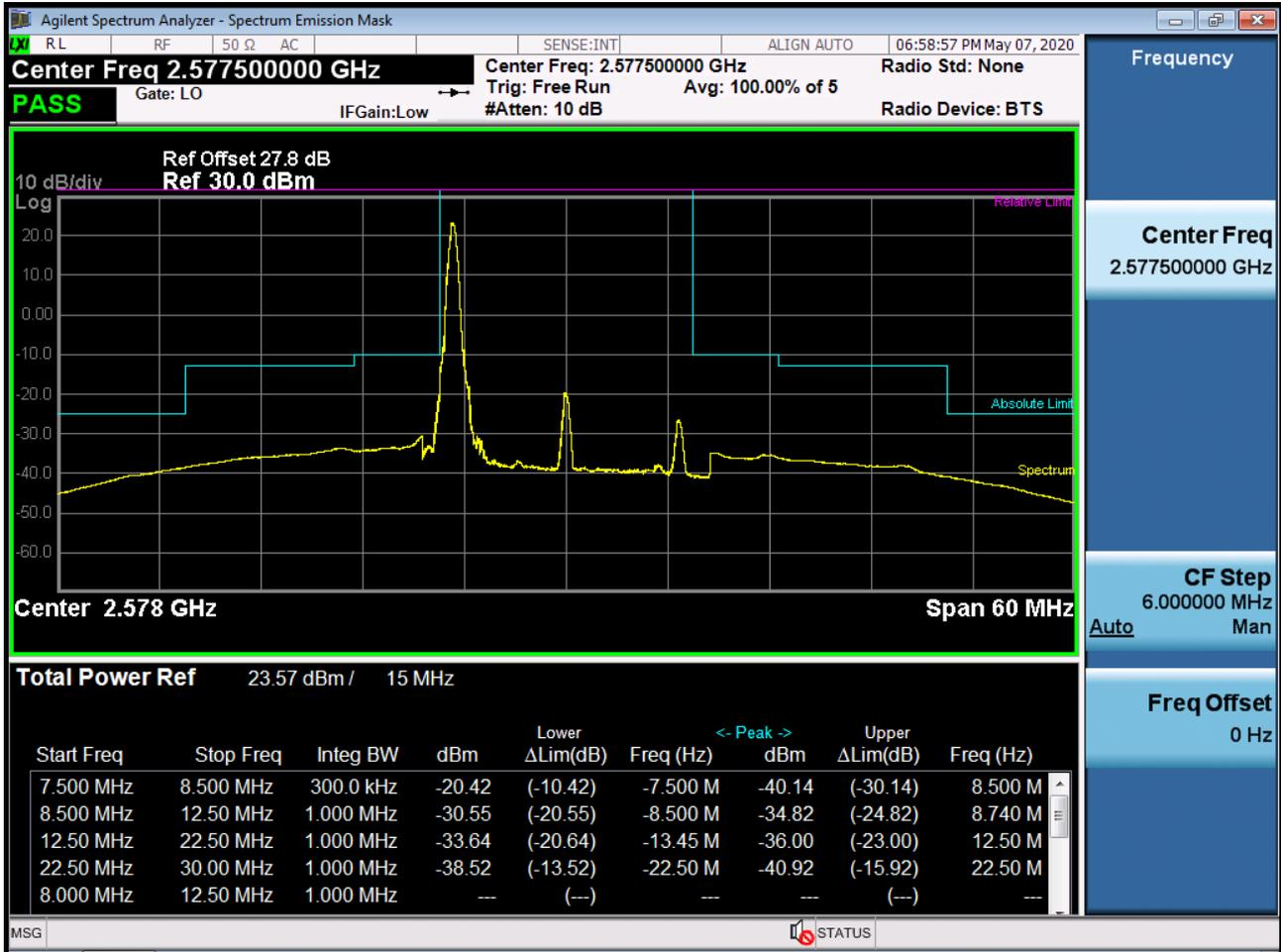
BAND 38. Low Channel Edge Plot (15 MHz Ch.37825 QPSK RB 75, Offset 0)
