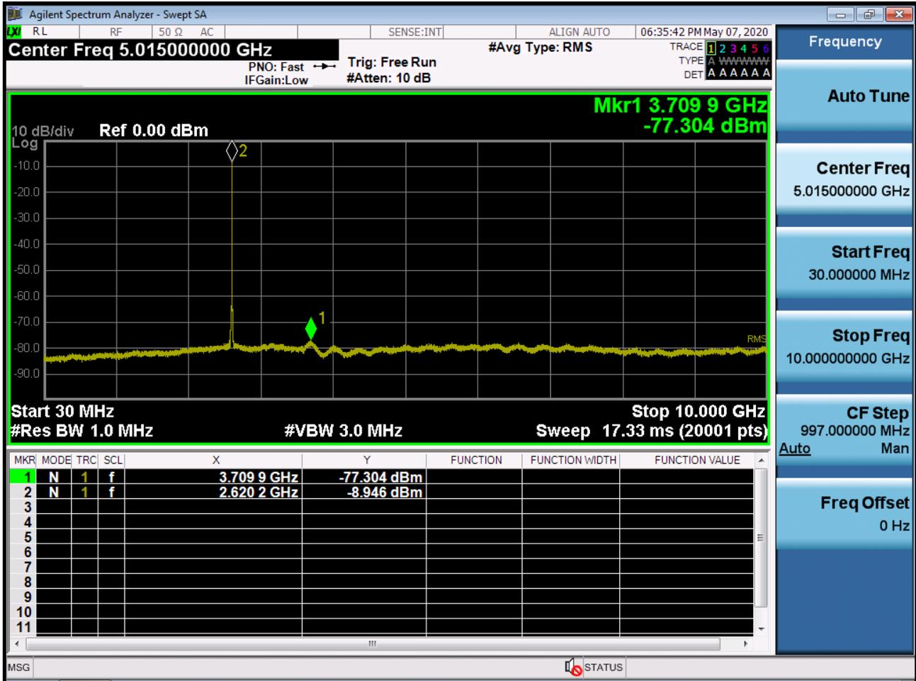
BAND 38. Conducted Spurious Plot 2 (5 MHz Ch. 38225 QPSK RB 1, Offset 0)
