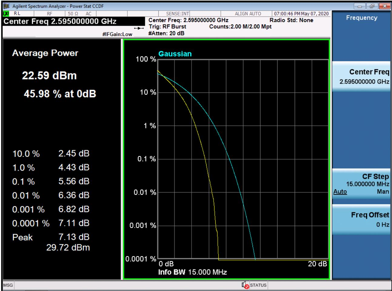
BAND 38. PAR Plot (15M BW\_Ch.38000\_16QAM\_RB75\_0)
