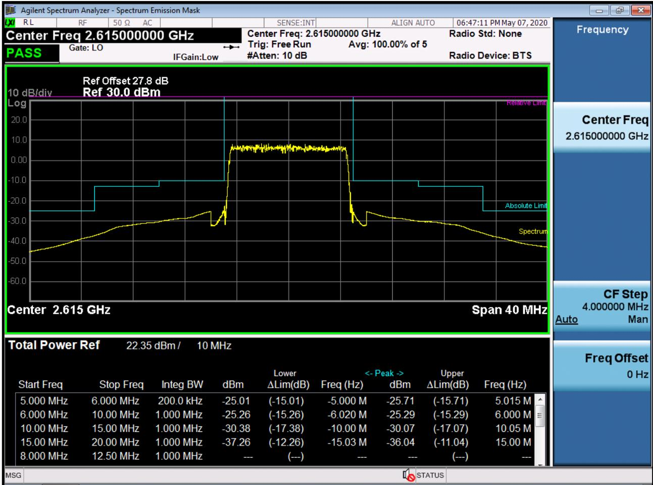
BAND 38. Low Channel Edge Plot (15 MHz Ch.37825 QPSK RB 1, Offset 0)
