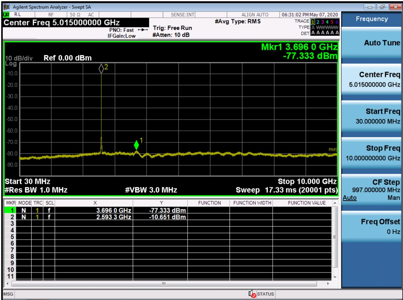
BAND 38. Conducted Spurious Plot 2 (5 MHz Ch. 38000 QPSK RB 1, Offset 0)
