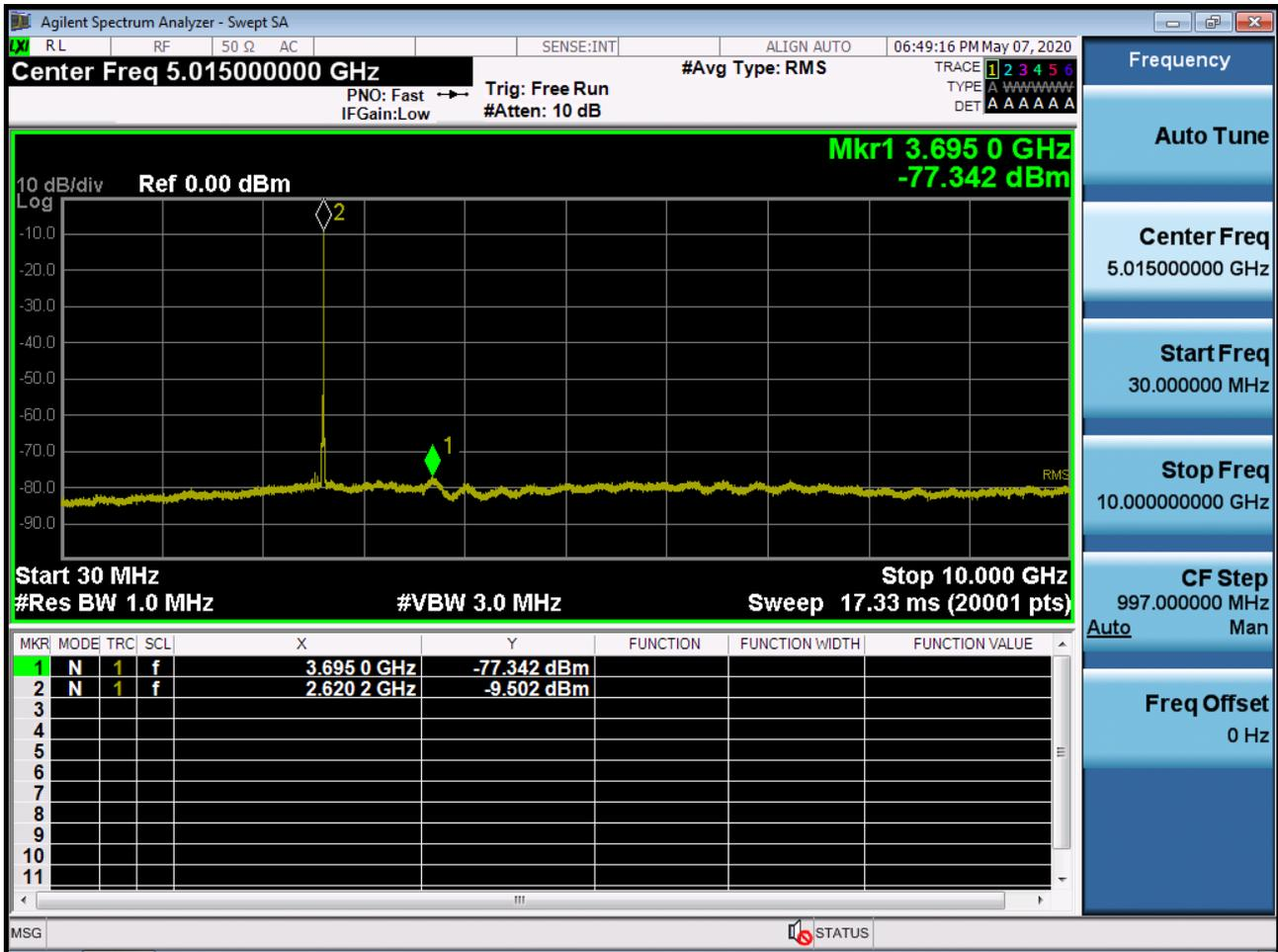
BAND 38. Conducted Spurious Plot 2 (10 MHz Ch. 38200 QPSK RB 1, Offset 0)
