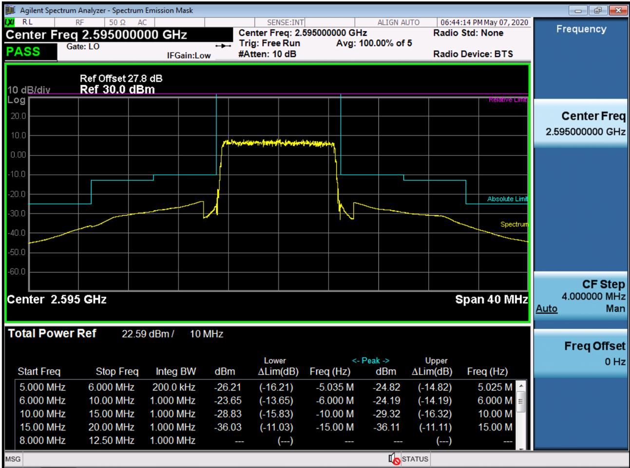
BAND 38. High Channel Edge Plot (10 MHz Ch.38200 QPSK RB 1, Offset 0)
