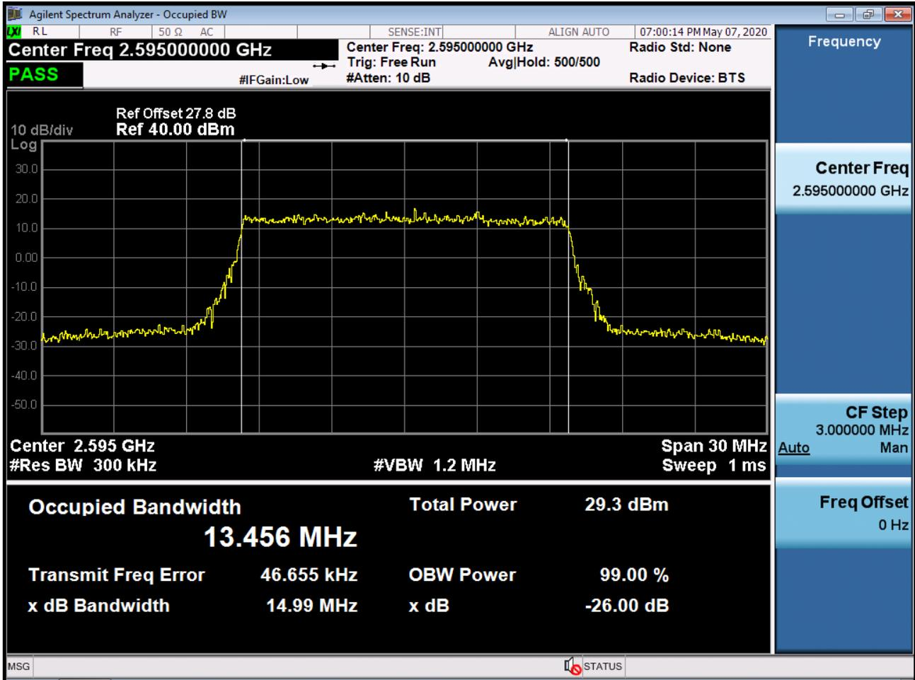
BAND 38. Occupied Bandwidth Plot (15 MHz Ch.38000 64-QAM RB 75)
