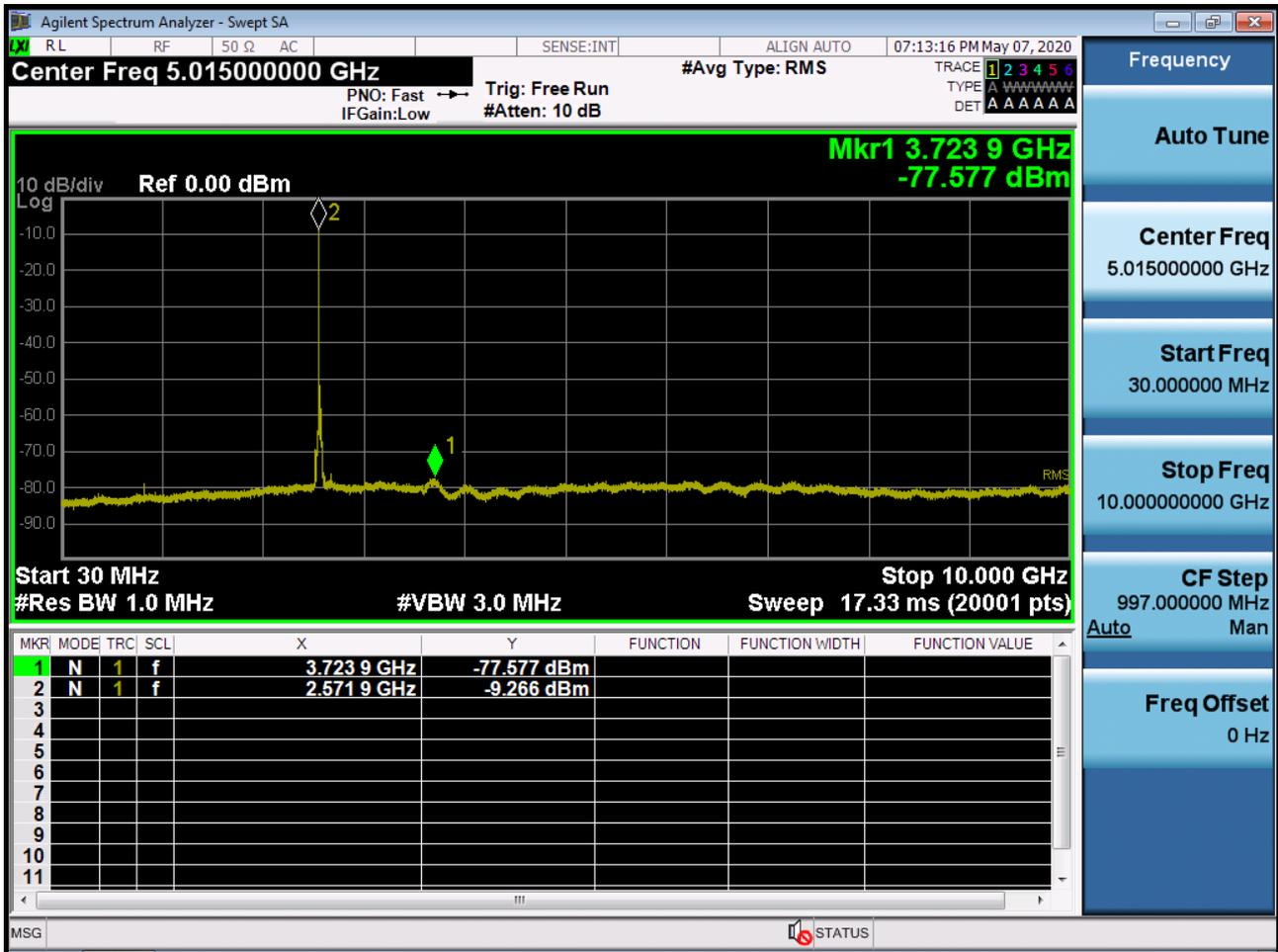
BAND 38. Conducted Spurious Plot 2 (20 MHz Ch. 37850 QPSK RB 1, Offset 0)
