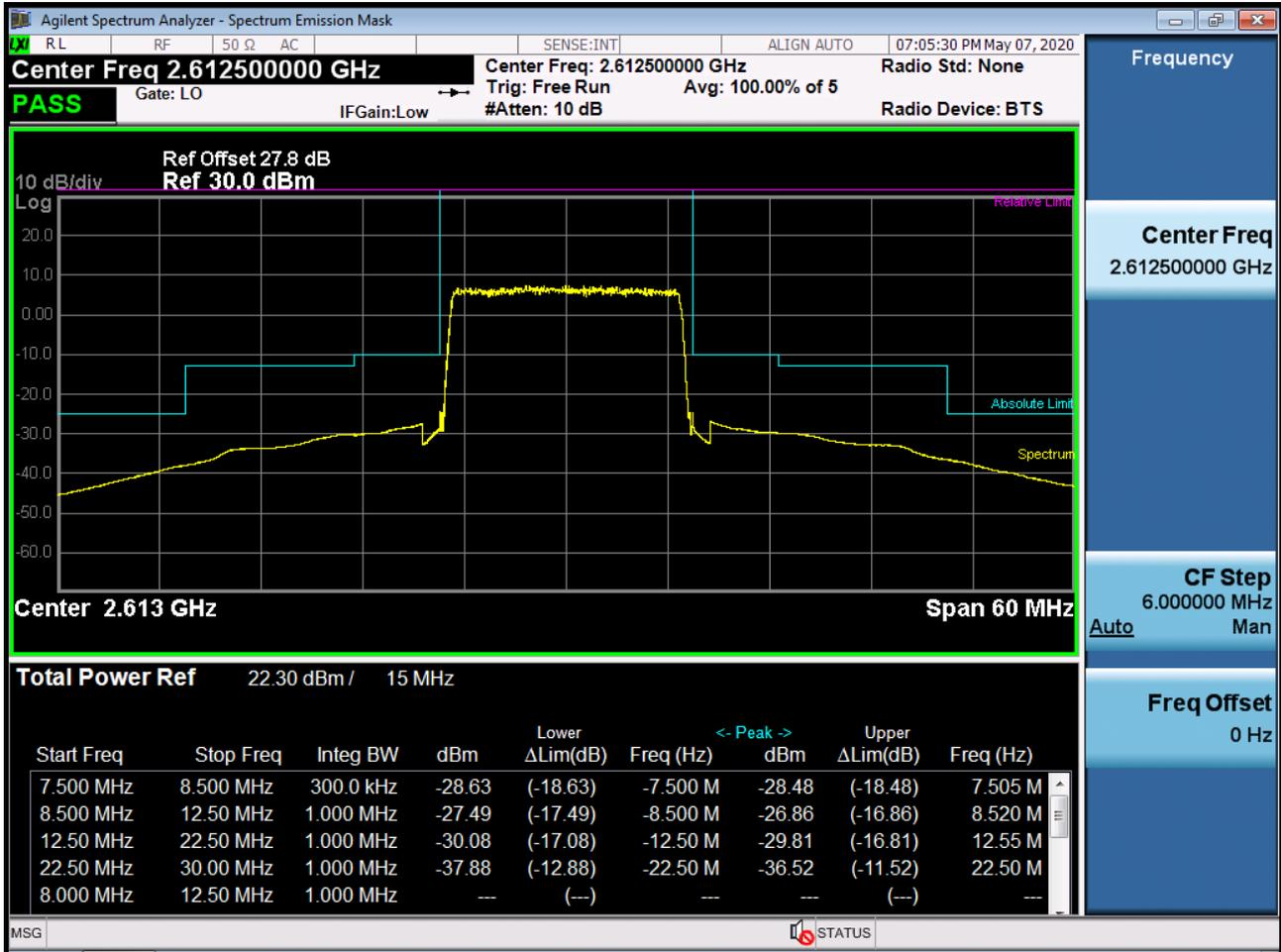
BAND 38. Low Channel Edge Plot (20 MHz Ch.37850 QPSK RB 1, Offset 0)
