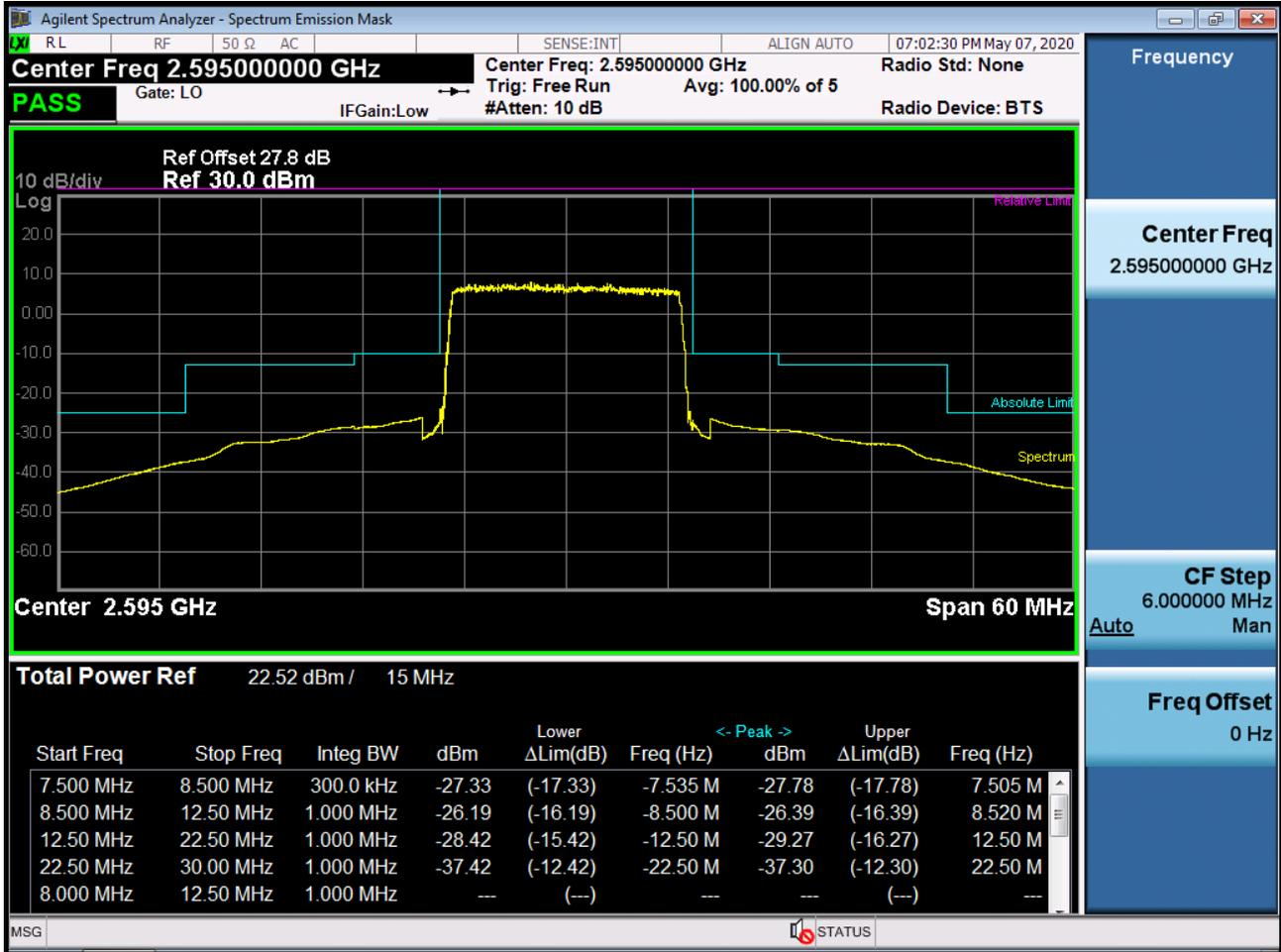
BAND 38. High Channel Edge Plot (15 MHz Ch.38175 QPSK RB 1, Offset 0)
