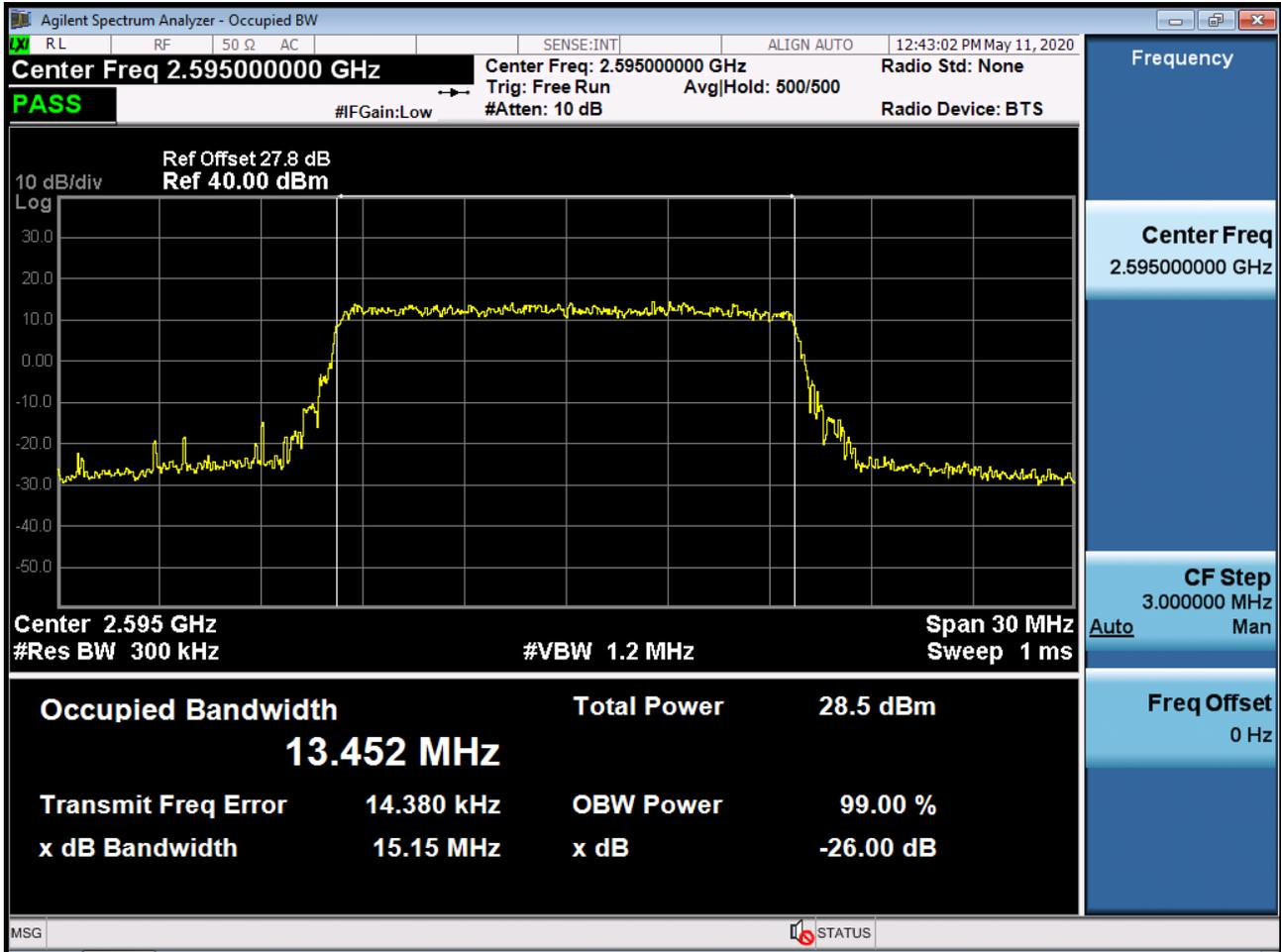
BAND 38. Occupied Bandwidth Plot (20 MHz Ch.38000 QPSK RB 100)
