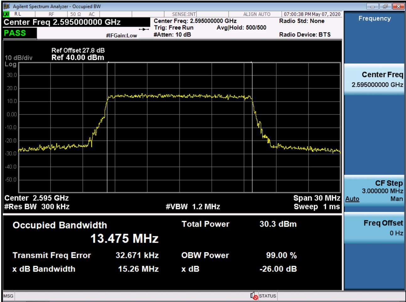
BAND 38. Occupied Bandwidth Plot (15 MHz Ch.38000 16-QAM RB 75)
