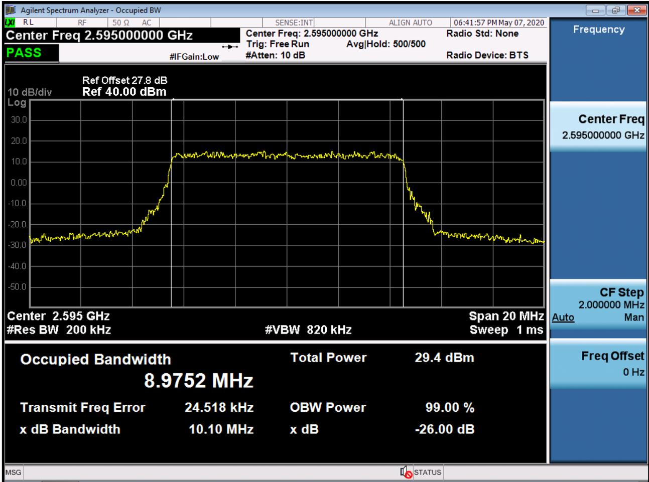
BAND 38. Occupied Bandwidth Plot (10 MHz Ch.38000 64-QAM RB 50)
