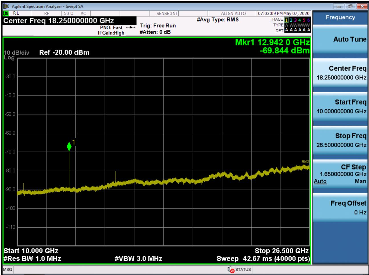
BAND 38. Conducted Spurious Plot 1 (15 MHz Ch.38175 QPSK RB 1, Offset 0)
