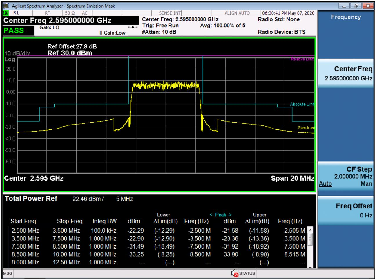
BAND 38. High Channel Edge Plot (5 MHz Ch.38225 QPSK RB 1, Offset 0)
