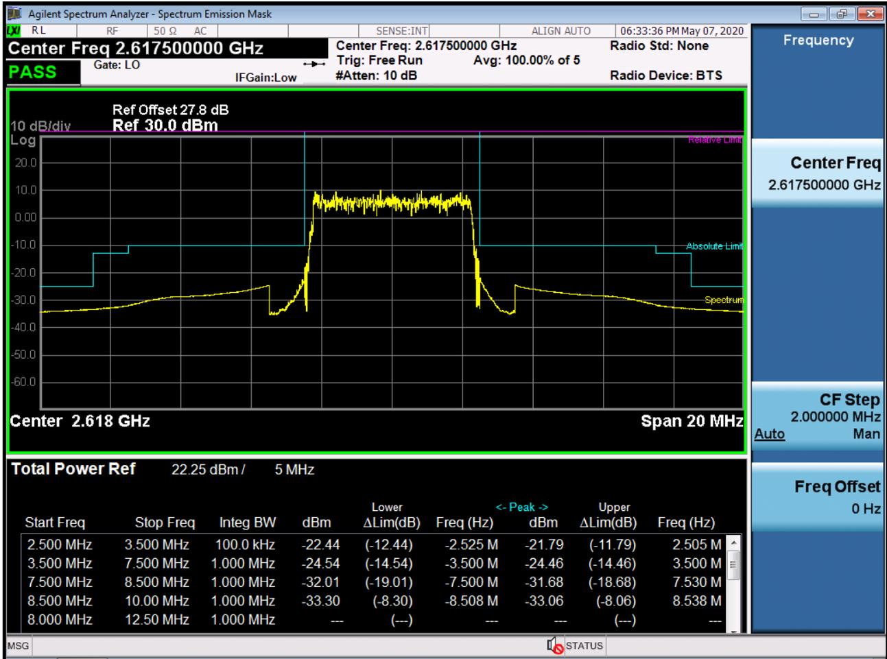
BAND 38. Low Channel Edge Plot (10 MHz Ch.37800 QPSK RB 1, Offset 0)
