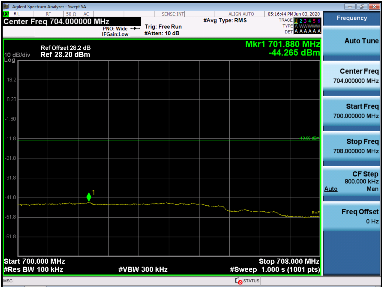
Sub6 n71. Upper Extended Band Edge Plot (20M BW Ch.137600 BPSK_RB50_0)
