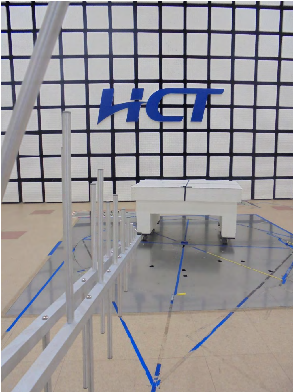
NFC Radiated Test Setup Photo for 30 MHz ~ 1 GHz : Without Tag
