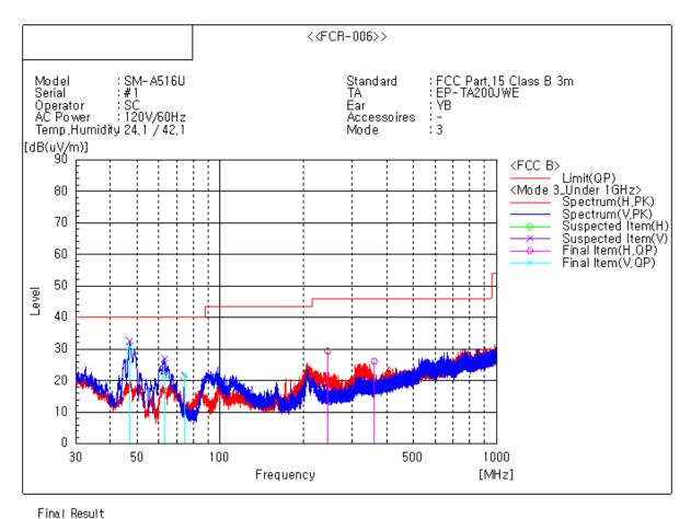
Note1) Receiving antenna polarization : Horizontal, Vertical
