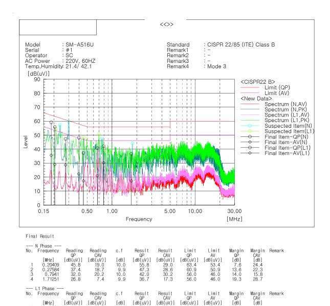
48.9 38.1 27.3 30.7 59.0 48.1 37.3 40.7 5.2 9.8 19.5 15.3 18.6 25.6 29.5 25.1 Note 1) Two graphs measured for both Live(L1) and Neutral(N) of the LISN are combined into one graph Note 2) Level (QP and/or CAV) = Meter Reading (QP and/or CAV) + Corr. (LISN Insertion Loss + Cable Loss) Margin (QP and/or CAV) = Limit – Level (QP and/or CAV) QP = Quasi-Peak, CAV = CISPR-Average, Corr. = Correction Factor.
