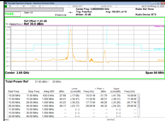
16QAM High channel 1RB_Offset Low
