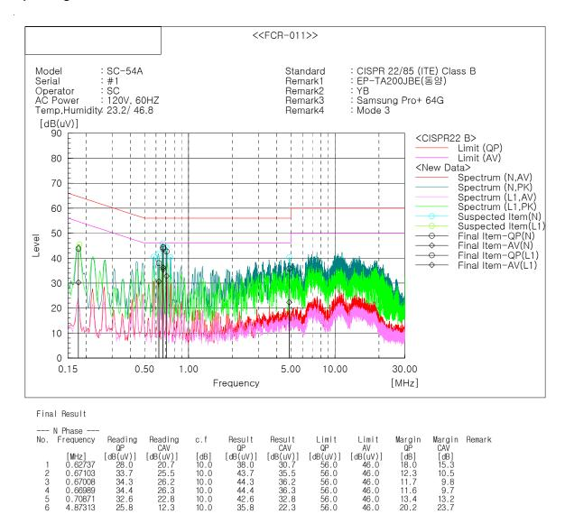
Note 1) Two graphs measured for both Live(L1) and Neutral(N) of the LISN are combined into one graph Note 2) Level (QP and/or CAV) = Meter Reading (QP and/or CAV) + Corr. (LISN Insertion Loss + Cable Loss) Margin (QP and/or CAV) = Limit – Level (QP and/or CAV) QP = Quasi-Peak, CAV = CISPR-Average, Corr. = Correction Factor.
