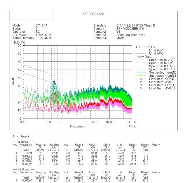
Note 1) Two graphs measured for both Live(L1) and Neutral(N) of the LISN are combined into one graph Note 2) Level (QP and/or CAV) = Meter Reading (QP and/or CAV) + Corr. (LISN Insertion Loss + Cable Loss) Margin (QP and/or CAV) = Limit – Level (QP and/or CAV) QP = Quasi-Peak, CAV = CISPR-Average, Corr. = Correction Factor.
