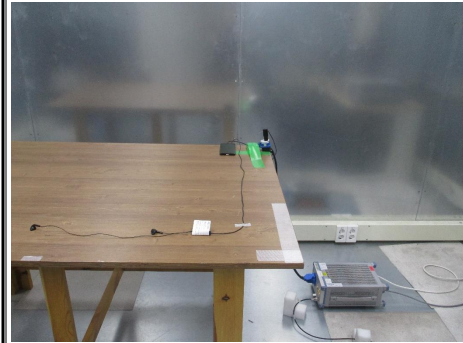
AC LINE CONDUCTED FRONT TEST PHOTO
