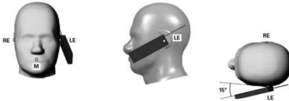
Figure 8.5. Tilt 15° position of the wireless device
