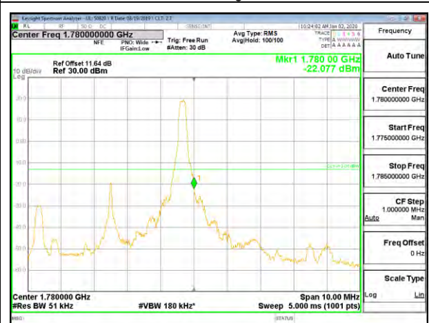
LTE B66 5MHz 16QAM High Channel RB1-24
