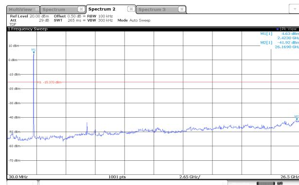
**Conducted band-edge / 2 437 MHz****Conducted spurious / 2 437 MHz**
