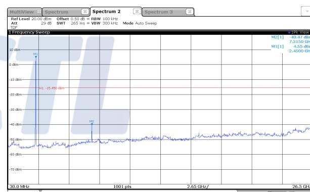
**Conducted band-edge / 2 462 MHz****Conducted spurious / 2 462 MHz**
