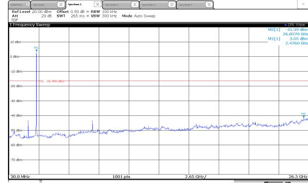
**Conducted band-edge / 2 472 MHz****Conducted spurious / 2 472 MHz**
