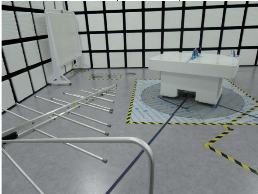
RADIATED FRONT PHOTO (BELOW 1 GHz)
