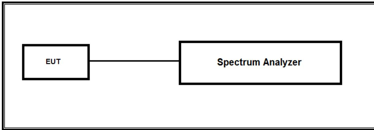
**SETUP DIAGRAM FOR TESTS (RADIATED TEST SETUP)**
