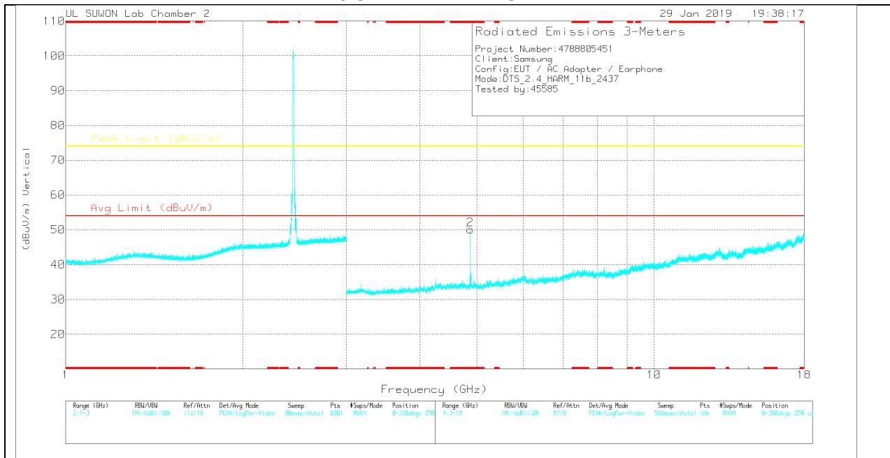
Note: Emission was scanned up to 26GHz; No emissions were detected above the noise floor which was at least 20dB below the specification limit.
