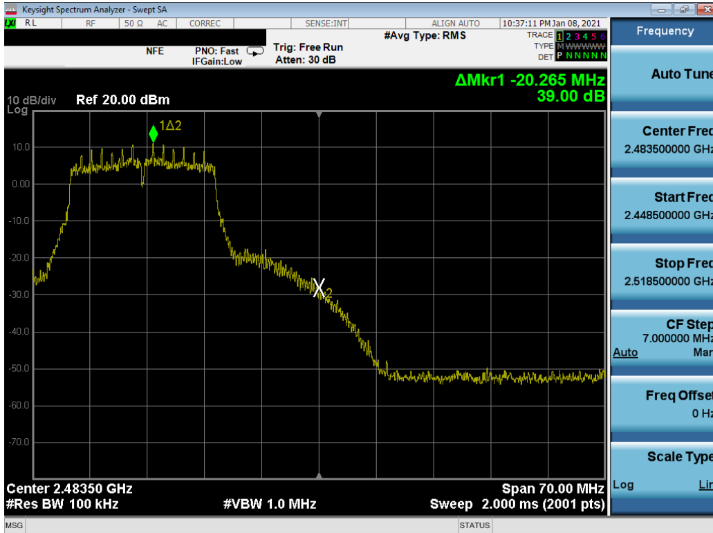
Plot 7-31. Band Edge Plot (802.11n (2.4GHz) – Ch. 11)
