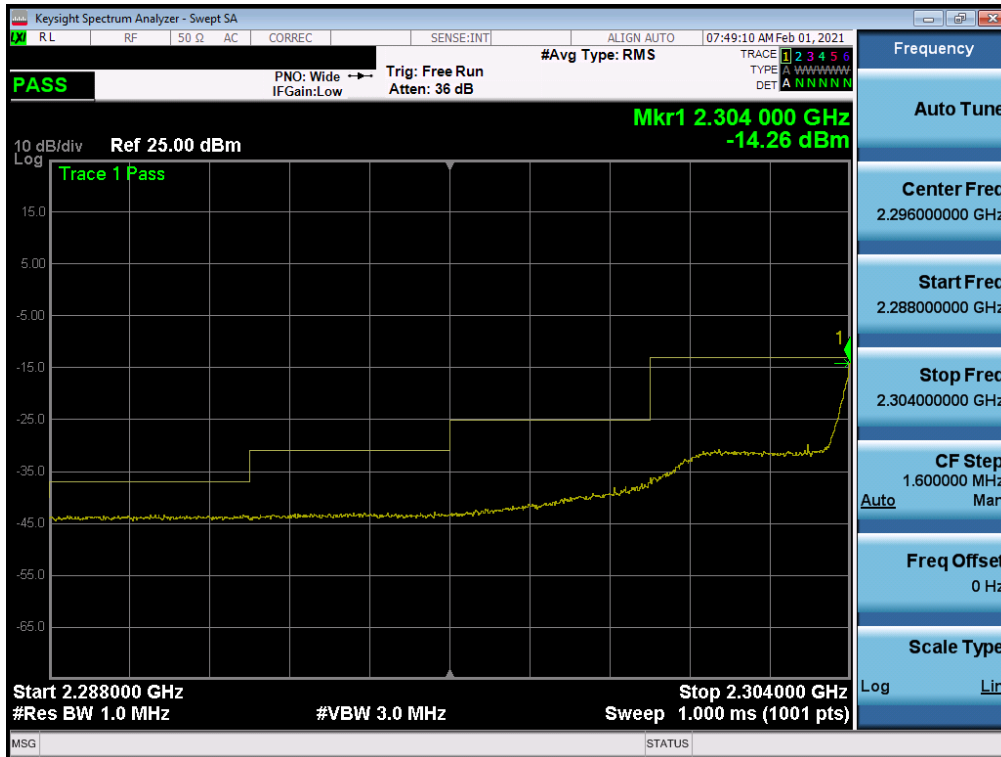
Plot 7-114. Extended Lower Band Edge Plot (LTE Band 30 - 5MHz QPSK – Full RB)
