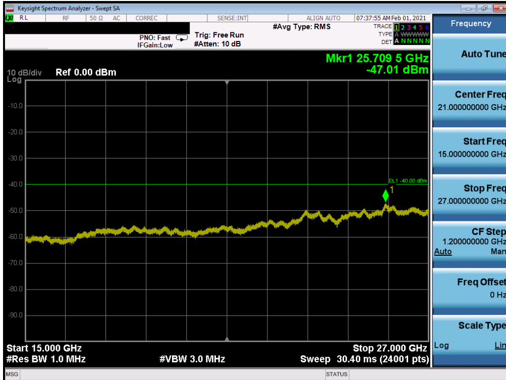
Plot 7-63. Conducted Spurious Plot (LTE Band 30 - 10MHz QPSK - RB Size 1, RB Offset 0)
