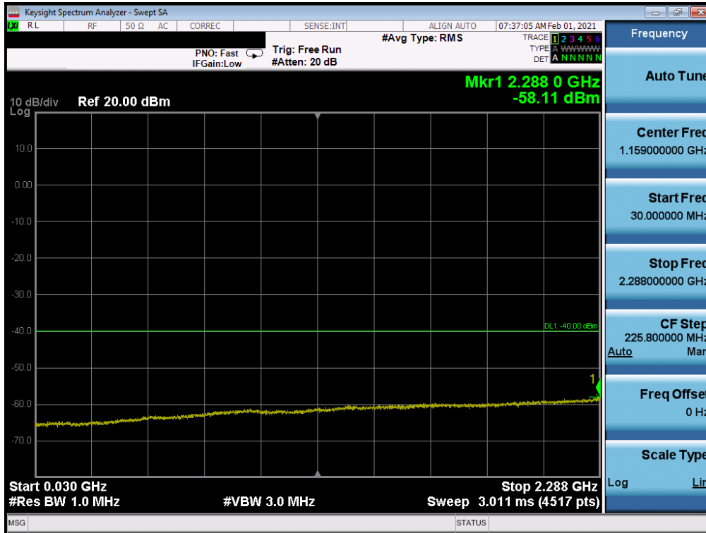
Plot 7-61. Conducted Spurious Plot (LTE Band 30 - 10MHz QPSK - RB Size 1, RB Offset 0)
