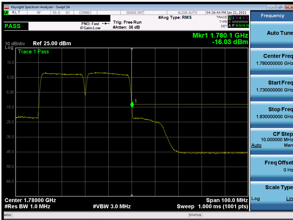
Plot 7-284. Upper Band Edge Plot (Band 66 QPSK – PCC:20 MHz SCC:20 MHz – Full RB)
