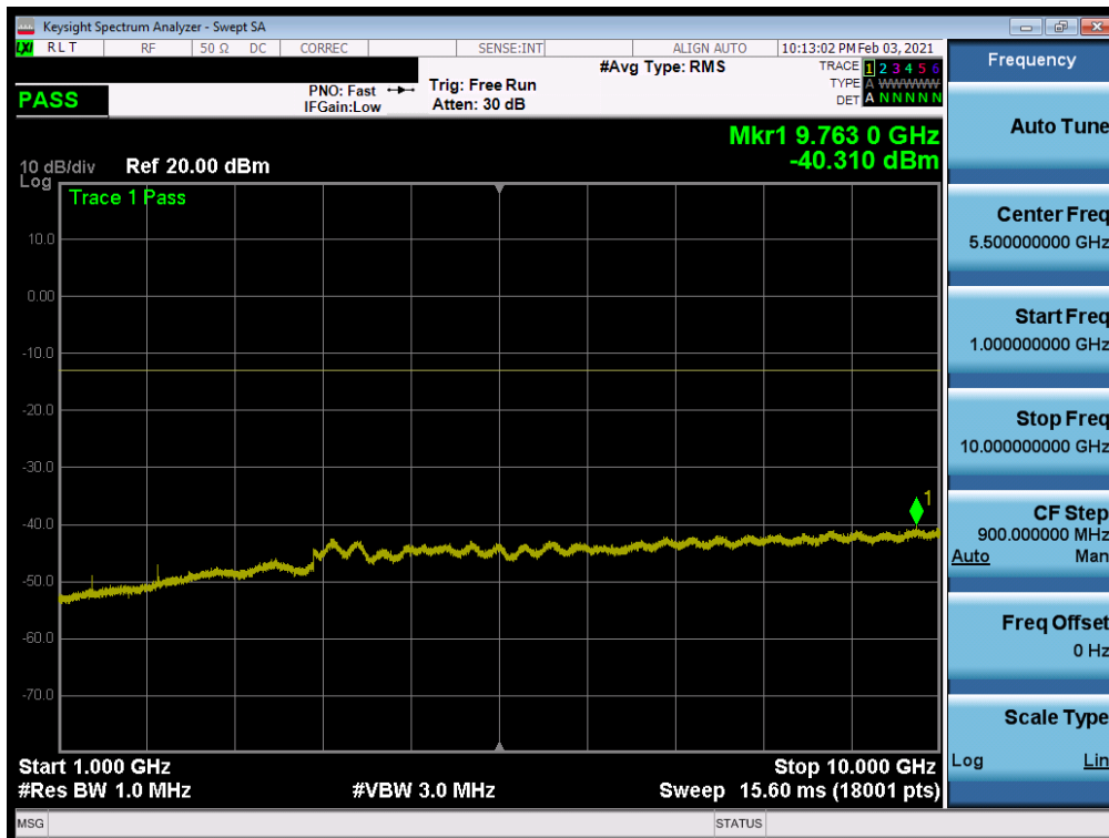
Plot 7-107. Conducted Spurious Plot (LTE Band 71 - 20MHz QPSK - RB Size 1, RB Offset 0 - Mid Channel)
