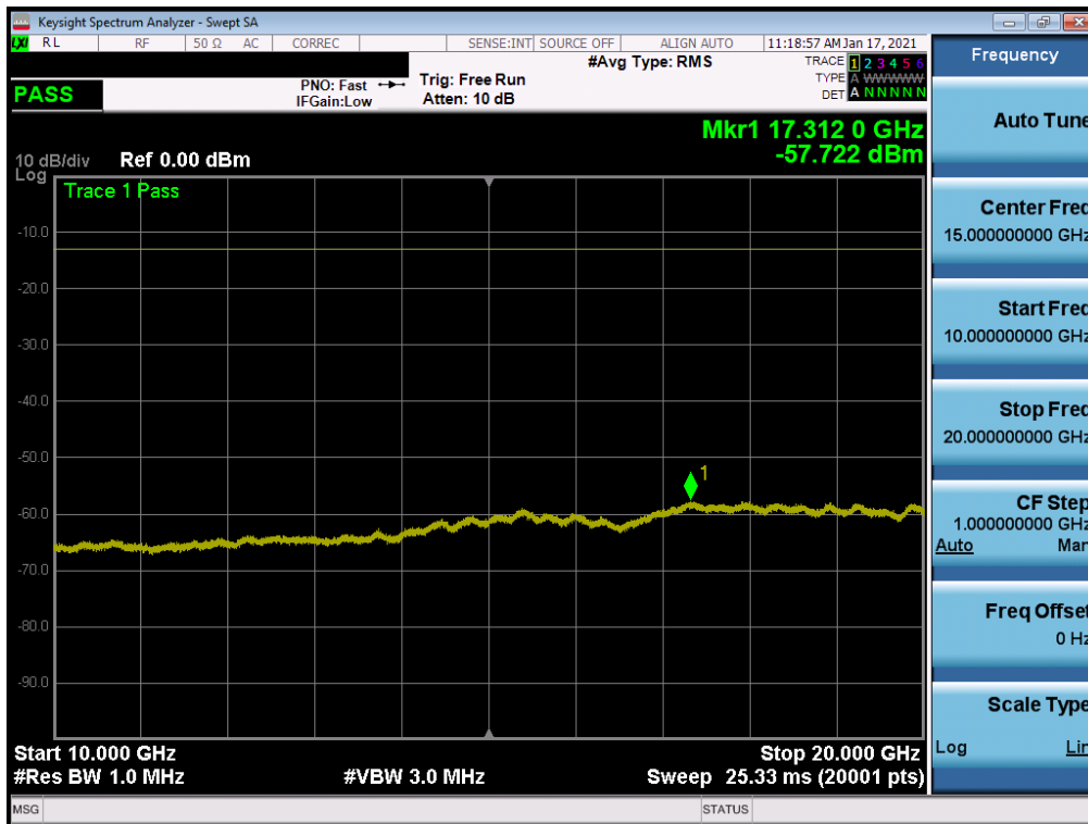
Plot 7-143. Conducted Spurious Plot (NR Band n66 - 20.0MHz - RB Size 1, RB Offset 0 - Mid Channel)
