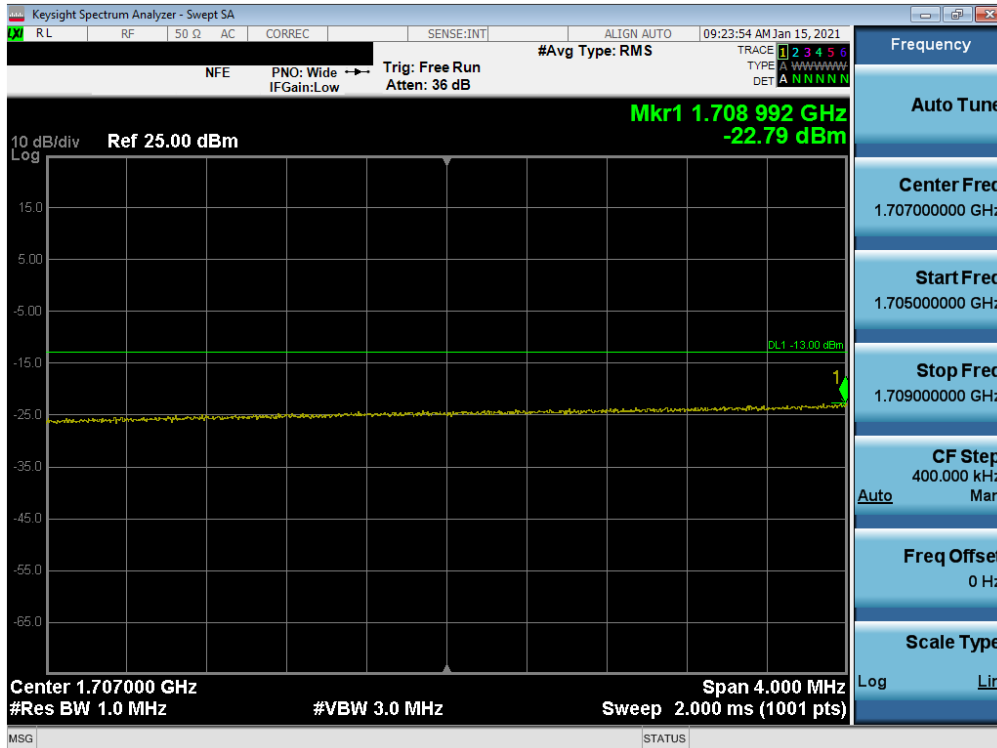
Plot 7-190. Lower Extended Band Edge Plot (LTE Band 66/4 - 15MHz QPSK – Full RB)
