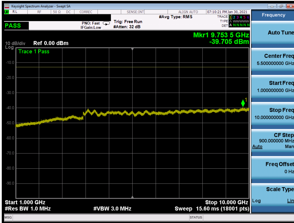
Plot 7-113. Conducted Spurious Plot (NR Band n71 - 20.0MHz - RB Size 1, RB Offset 0 - Low Channel)
