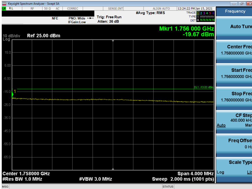
Plot 7-192. Upper Extended Band Edge Plot (LTE Band 4 - 15MHz QPSK – Full RB)
