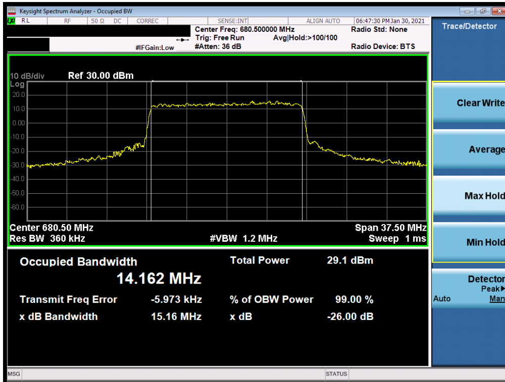
Plot 7-38. Occupied Bandwidth Plot (NR Band n71 - 15MHz CP-OFDM 16-QAM - Full RB)
