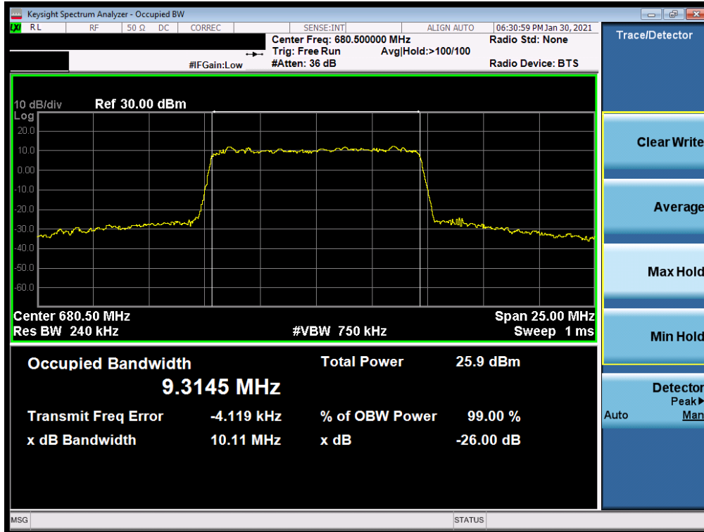
Plot 7-45. Occupied Bandwidth Plot (NR Band n71 - 10MHz CP-OFDM 256-QAM - Full RB)
