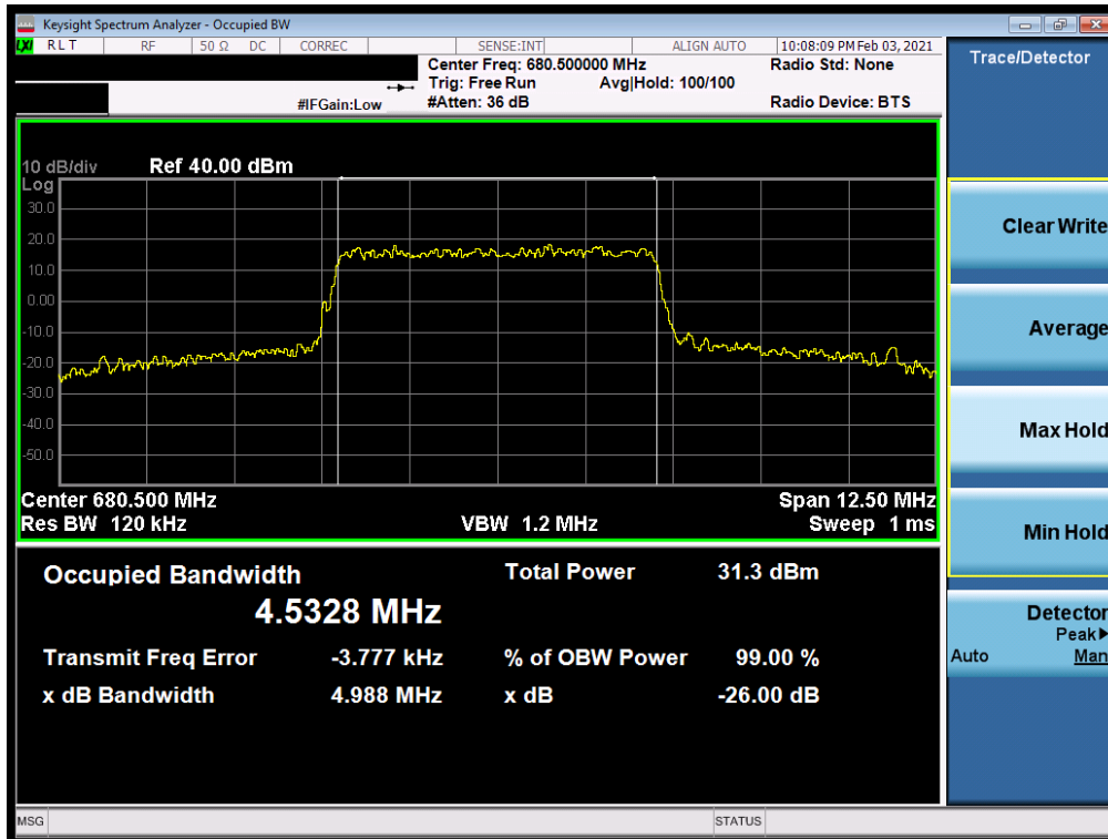
Plot 7-28. Occupied Bandwidth Plot (LTE Band 71 - 5MHz QPSK - Full RB)
