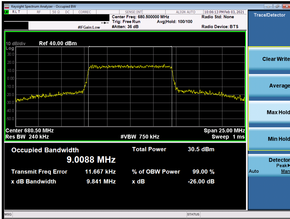
Plot 7-26. Occupied Bandwidth Plot (LTE Band 71 - 10MHz 16-QAM - Full RB)
