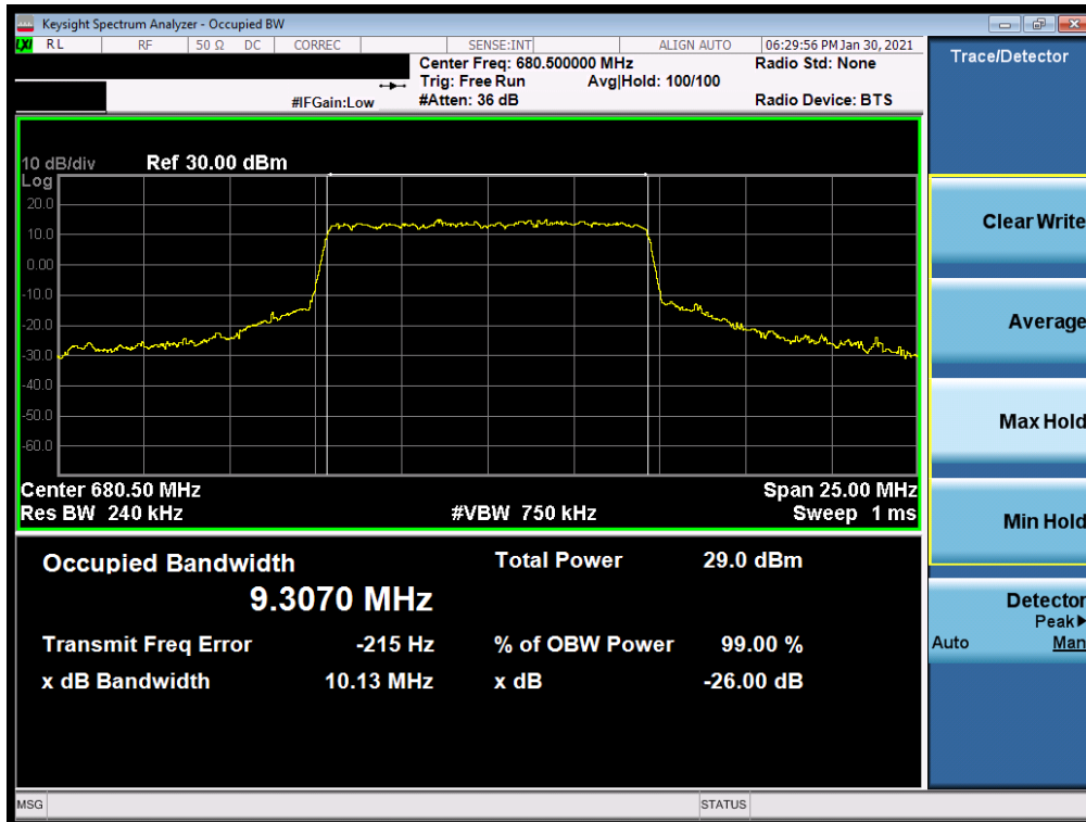
Plot 7-42. Occupied Bandwidth Plot (NR Band n71 - 10MHz CP-OFDM QPSK - Full RB)
