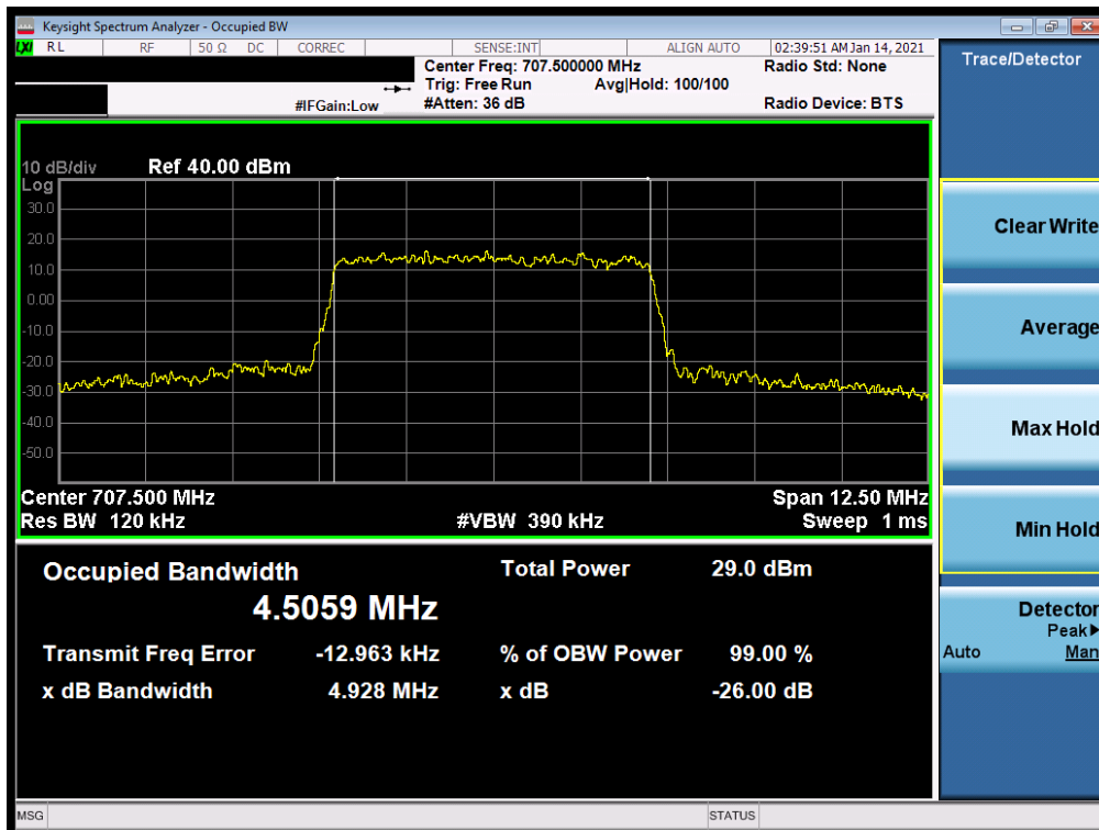
Plot 7-4. Occupied Bandwidth Plot (LTE Band 12 - 5MHz QPSK - Full RB)
