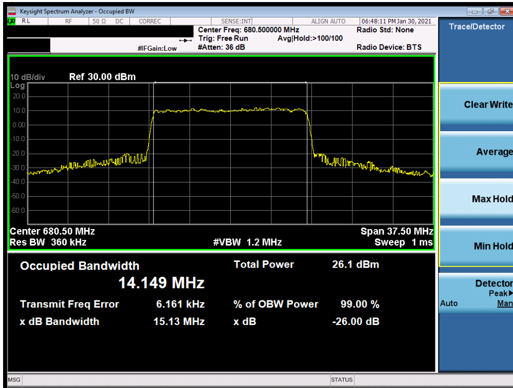
Plot 7-40. Occupied Bandwidth Plot (NR Band n71 - 15MHz CP-OFDM 256-QAM - Full RB)
