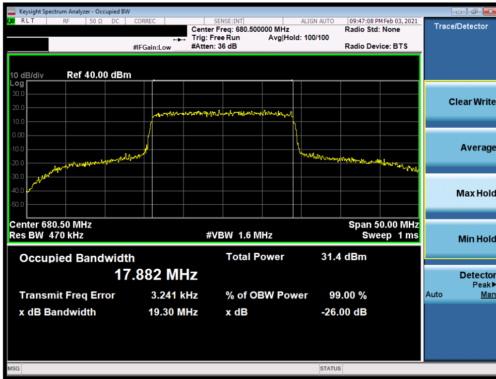
Plot 7-19. Occupied Bandwidth Plot (LTE Band 71 - 20MHz QPSK - Full RB)
