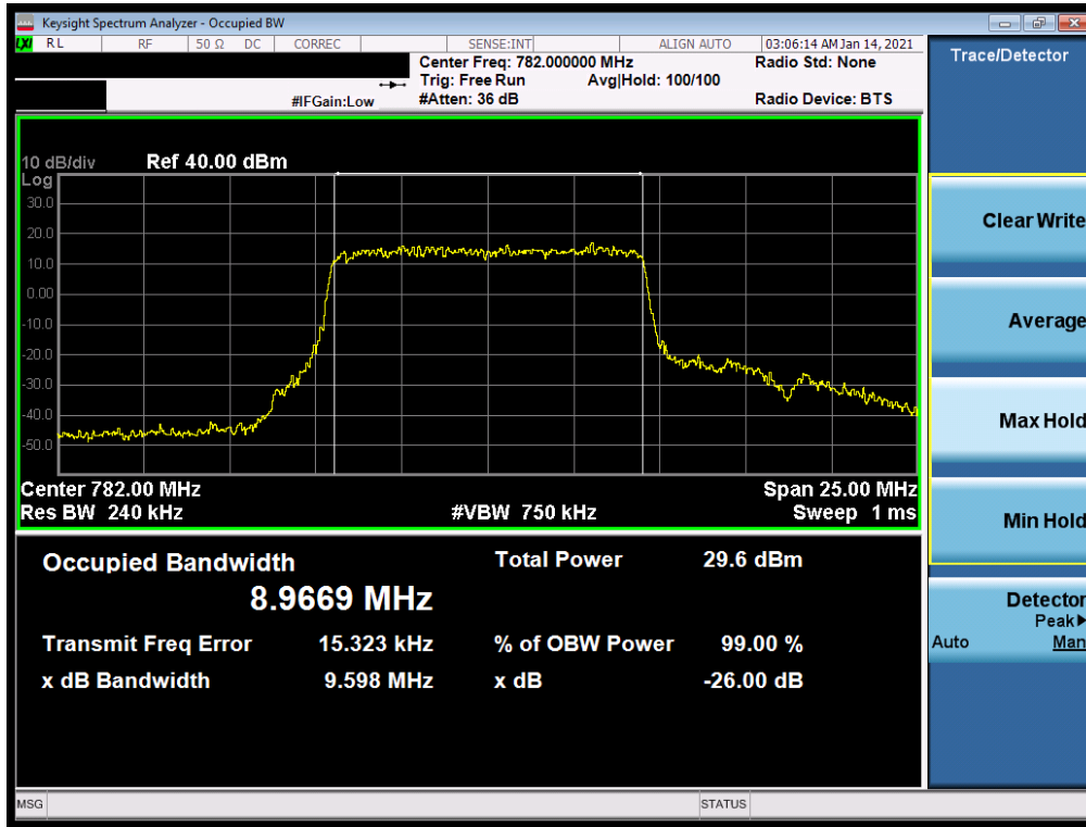
Plot 7-13. Occupied Bandwidth Plot (LTE Band 13 - 10MHz QPSK - Full RB)
