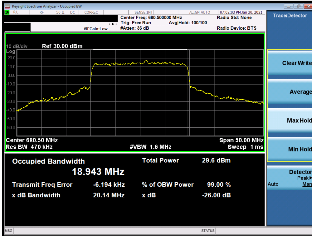
Plot 7-33. Occupied Bandwidth Plot (NR Band n71 - 20MHz CP-OFDM 16-QAM - Full RB)
