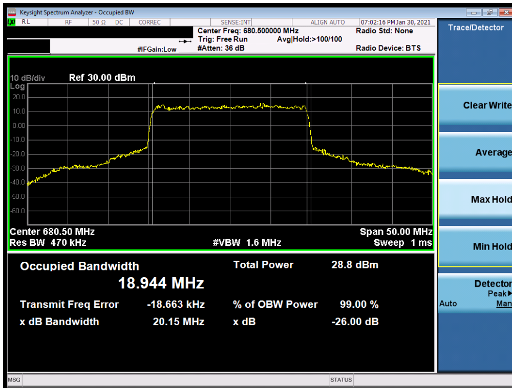
Plot 7-34. Occupied Bandwidth Plot (NR Band n71 - 20MHz CP-OFDM 64-QAM - Full RB)
