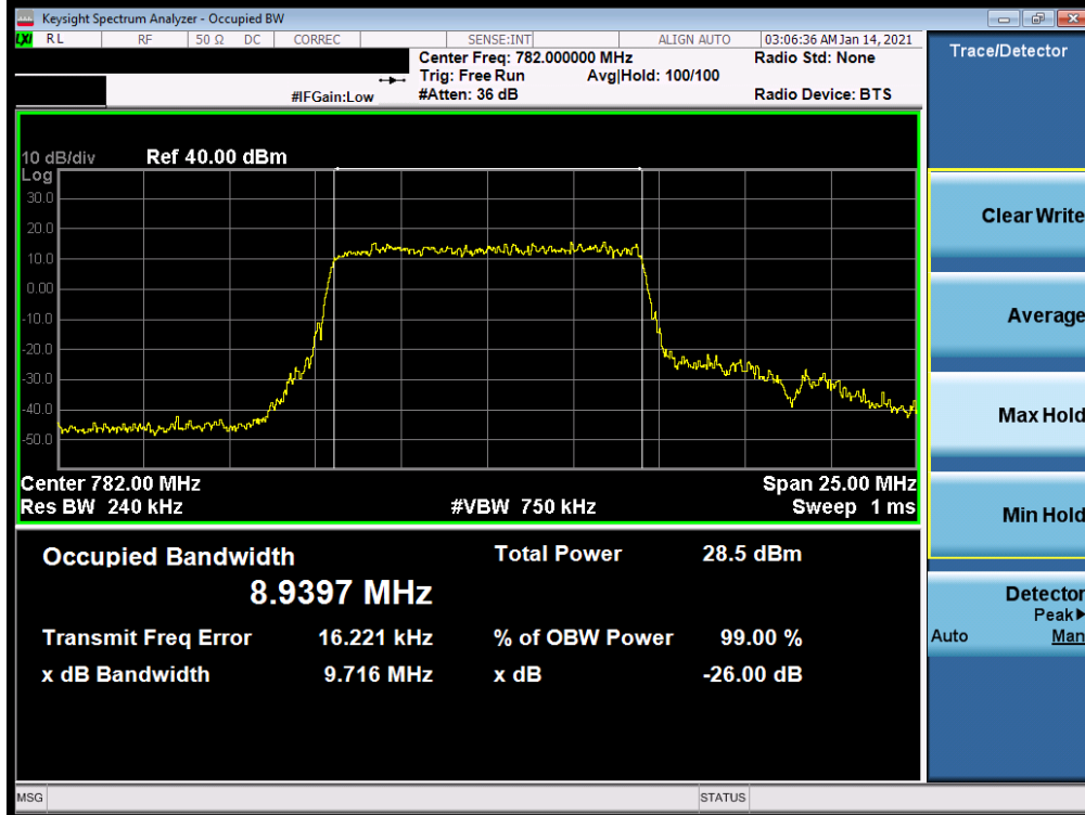
Plot 7-14. Occupied Bandwidth Plot (LTE Band 13 - 10MHz 16-QAM - Full RB)
