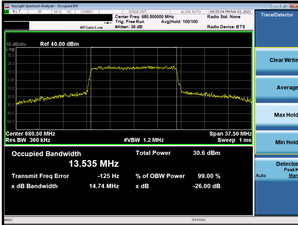
Plot 7-23. Occupied Bandwidth Plot (LTE Band 71 - 15MHz 16-QAM - Full RB)
