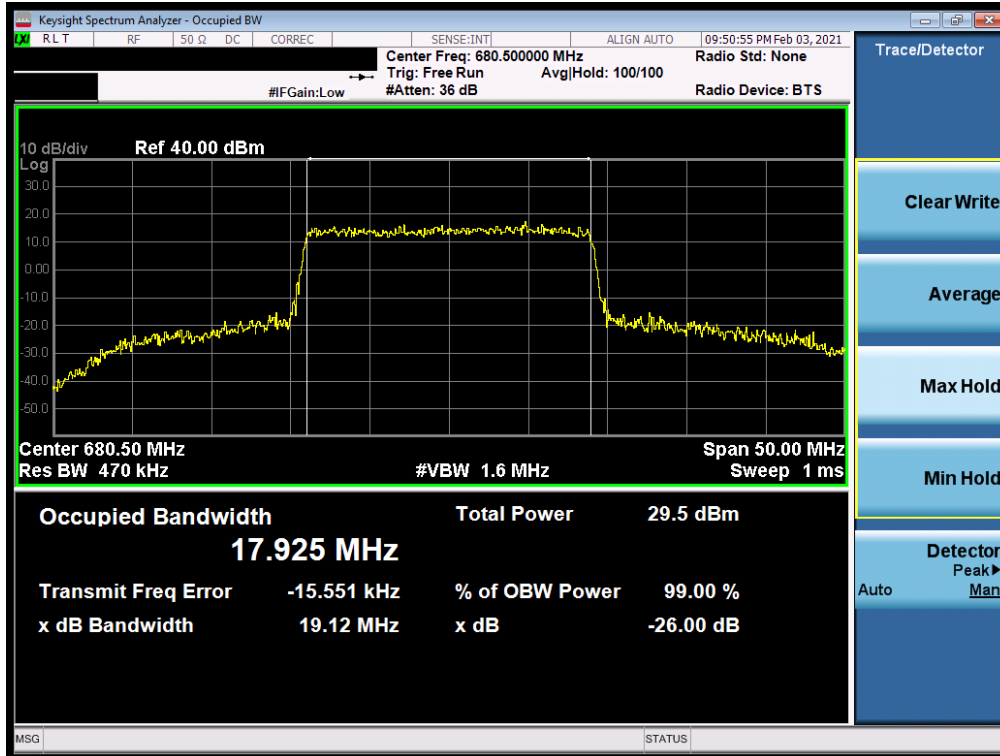
Plot 7-21. Occupied Bandwidth Plot (LTE Band 71 - 20MHz 64-QAM - Full RB)
