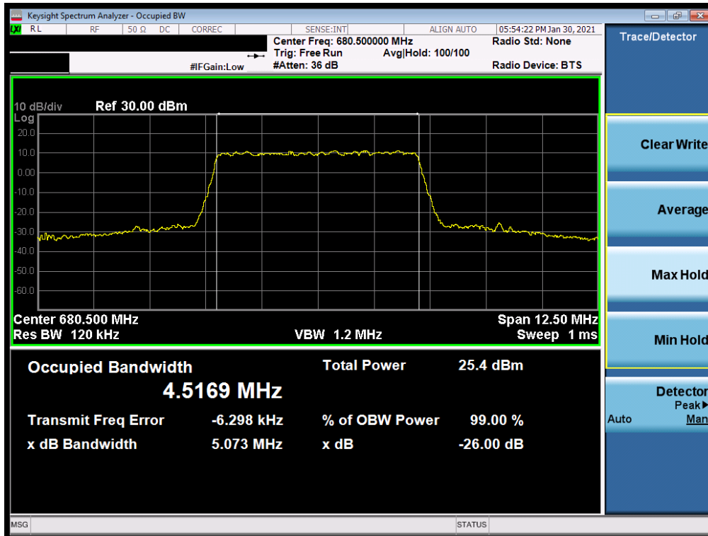
Plot 7-50. Occupied Bandwidth Plot (NR Band n71 - 5MHz CP-OFDM 256-QAM - Full RB)
