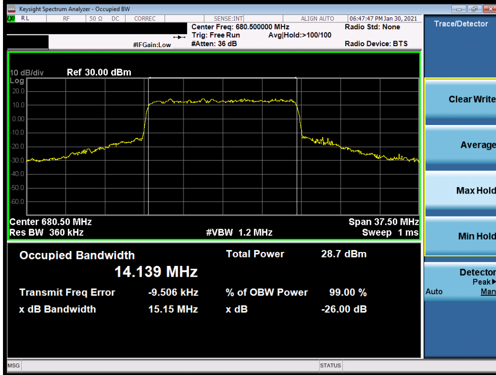
Plot 7-39. Occupied Bandwidth Plot (NR Band n71 - 15MHz CP-OFDM 64-QAM - Full RB)
