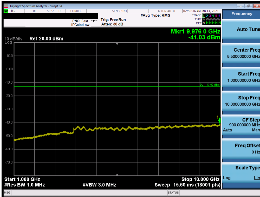
Plot 7-92. Conducted Spurious Plot (LTE Band 12 - 10MHz QPSK - RB Size 1, RB Offset 0 - Low Channel)
