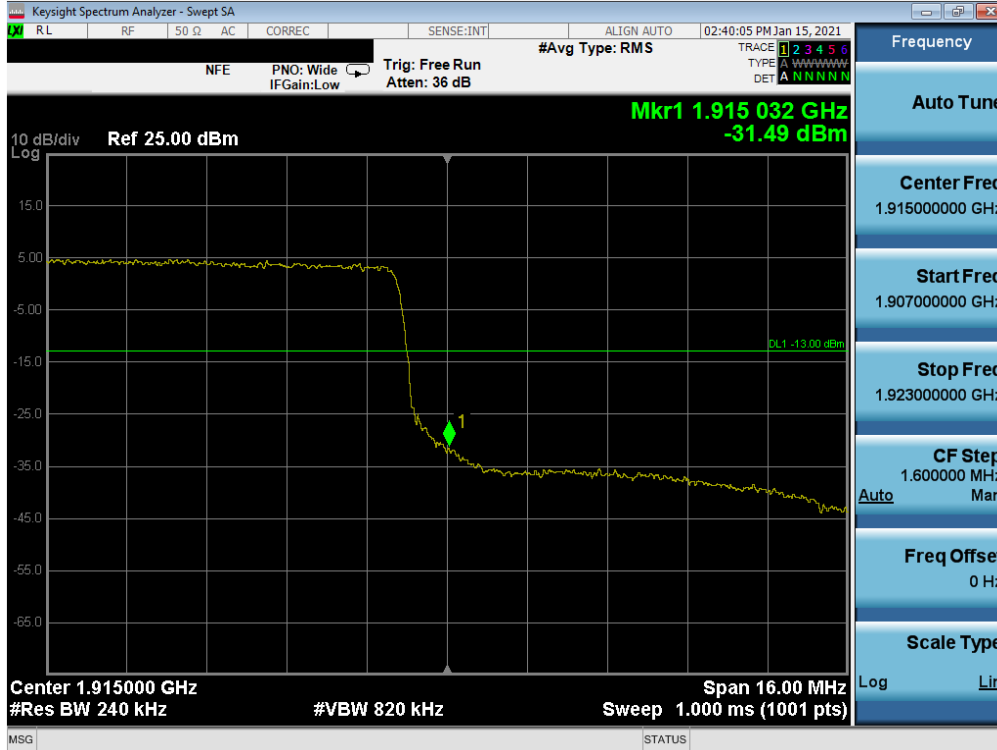
Plot 7-102. Upper Band Edge Plot (LTE Band 25 - 20MHz QPSK – Full RB Configuration)
