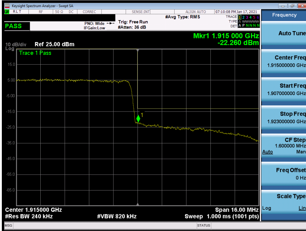
Plot 7-138. Upper Band Edge Plot (NR Band n25 - 20MHz QPSK – Full RB Configuration)
