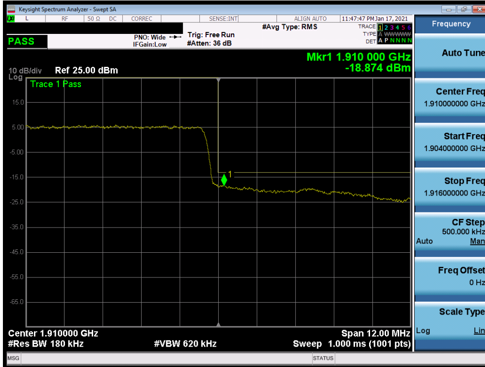
Plot 7-142. Upper Band Edge Plot (NR Band n2 - 15MHz QPSK – Full RB Configuration)
