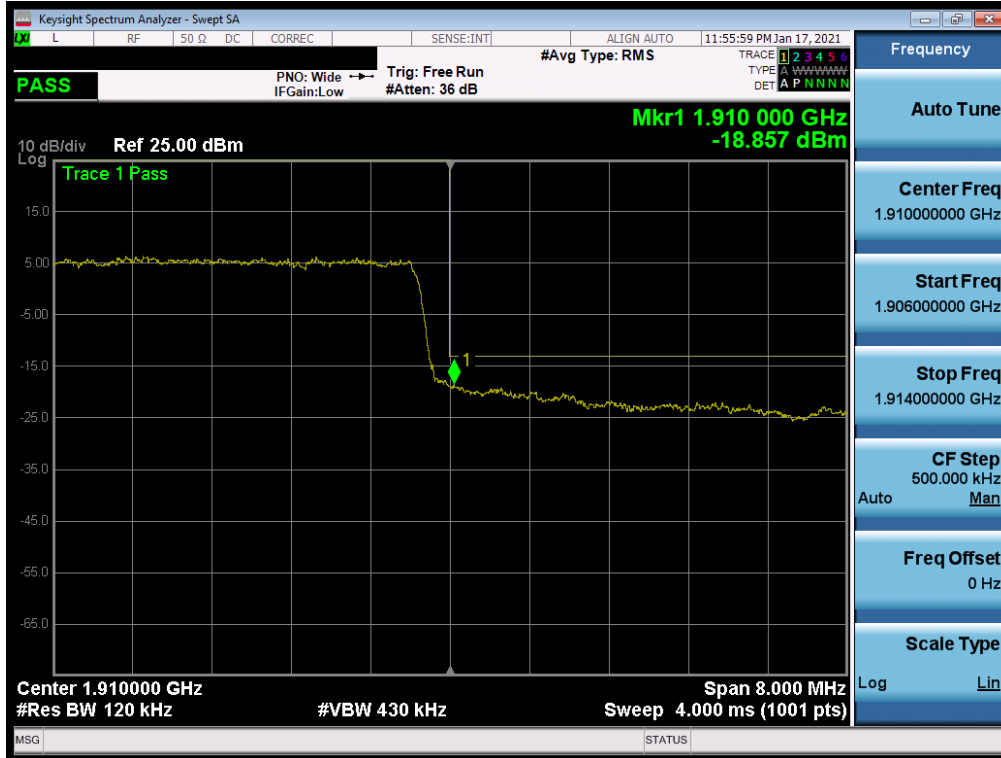
Plot 7-148. Upper Band Edge Plot (NR Band n2 - 10MHz QPSK – Full RB Configuration)
