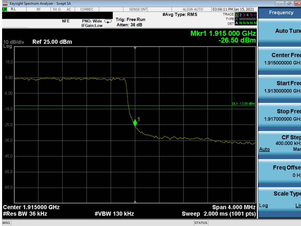
Plot 7-126. Upper Band Edge Plot (LTE Band 25 - 3MHz QPSK – Full RB Configuration)
