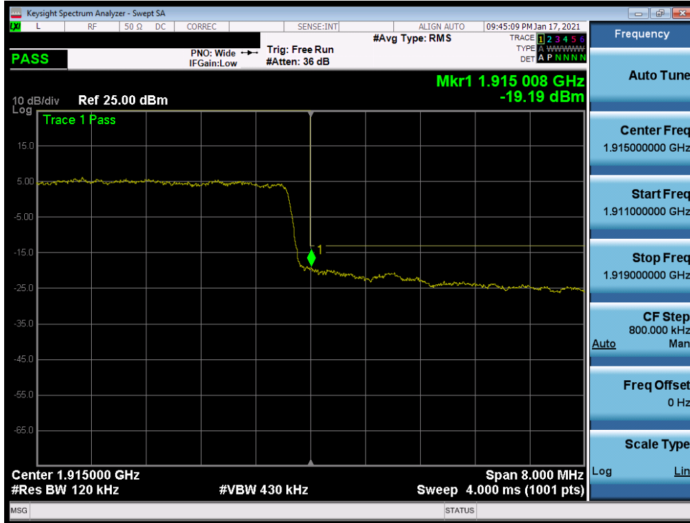
Plot 7-150. Upper Band Edge Plot (NR Band n25 - 10MHz QPSK – Full RB Configuration)
