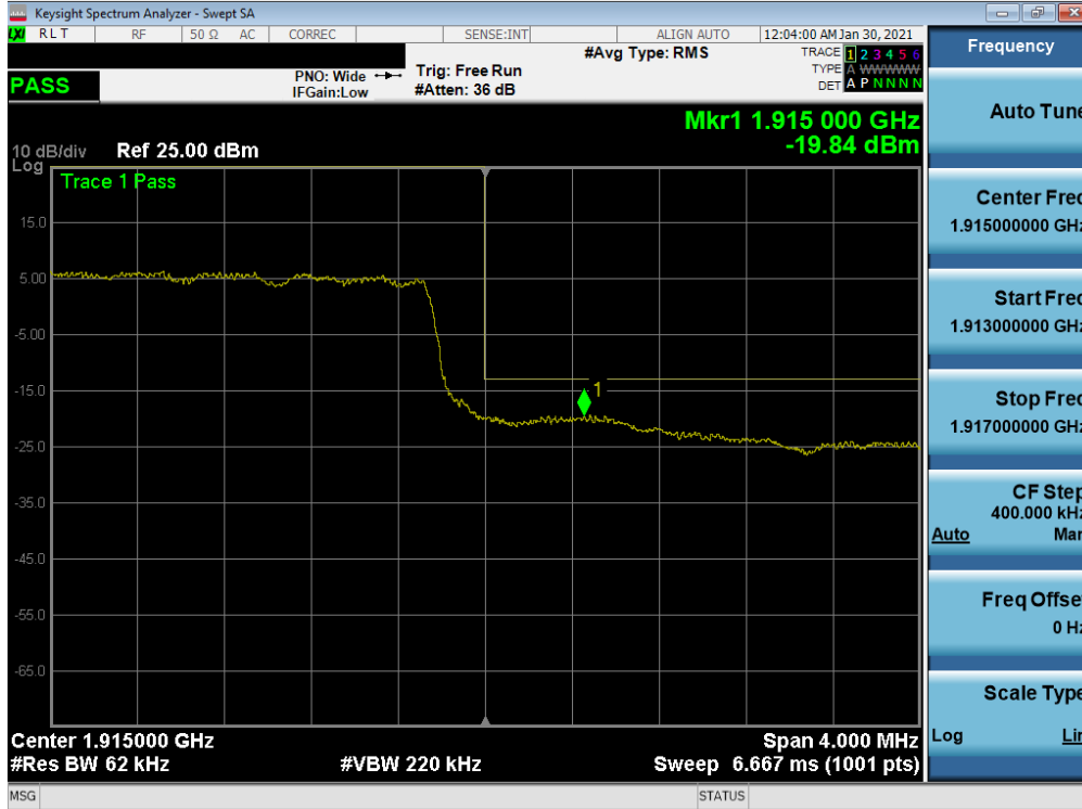
Plot 7-156. Upper Band Edge Plot (NR Band n25 – 5MHz QPSK – Full RB Configuration)
