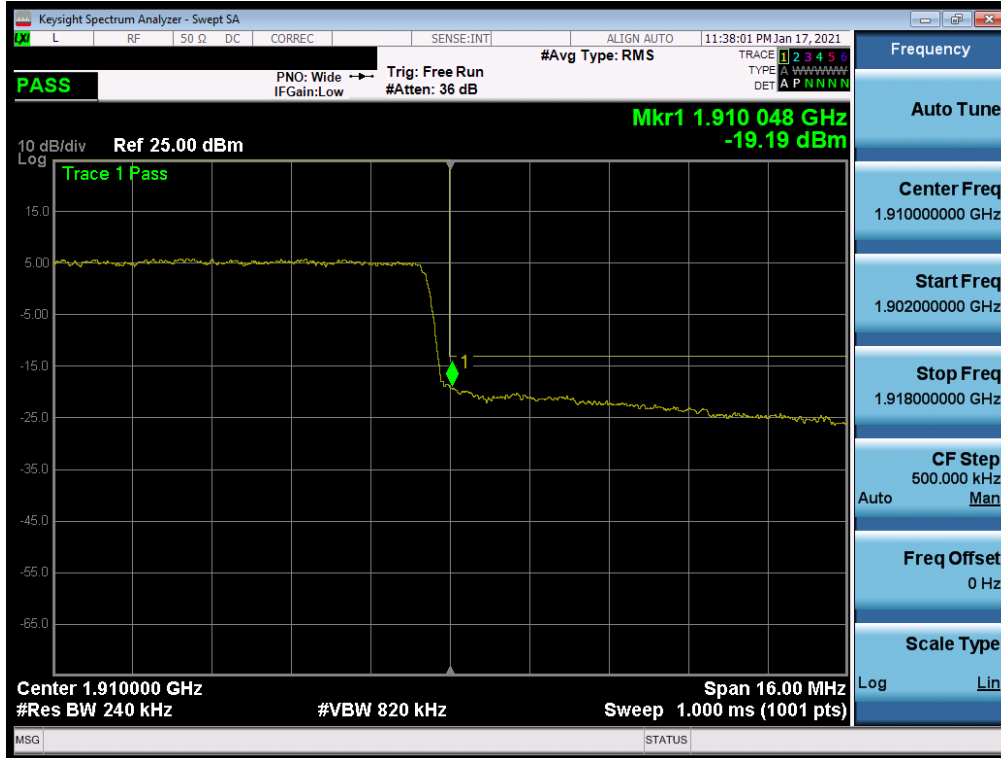
Plot 7-136. Upper Band Edge Plot (NR Band n2 - 20MHz QPSK – Full RB Configuration)
