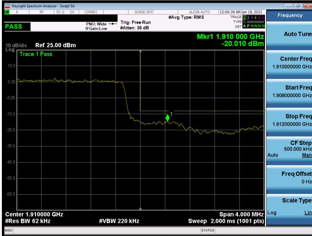
Plot 7-154. Upper Band Edge Plot (NR Band n2 – 5MHz QPSK – Full RB Configuration)
