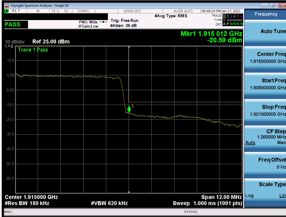
Plot 7-144. Upper Band Edge Plot (NR Band n25 - 15MHz QPSK – Full RB Configuration)
