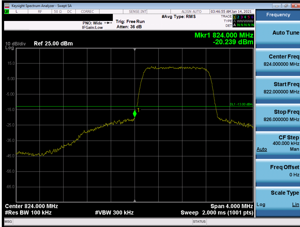
Plot 7-100. Lower Band Edge Plot (LTE Band 26/5 – 1.4MHz QPSK – Full RB Configuration)
