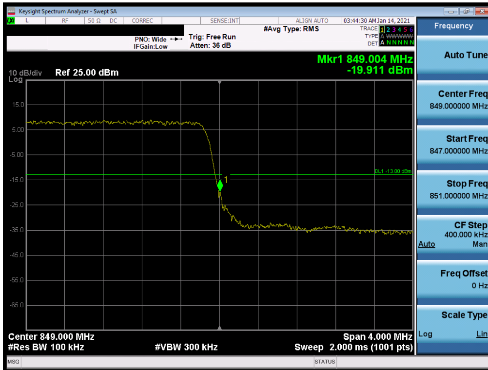
Plot 7-99. Upper Band Edge Plot (LTE Band 26/5 - 3MHz QPSK – Full RB Configuration)
