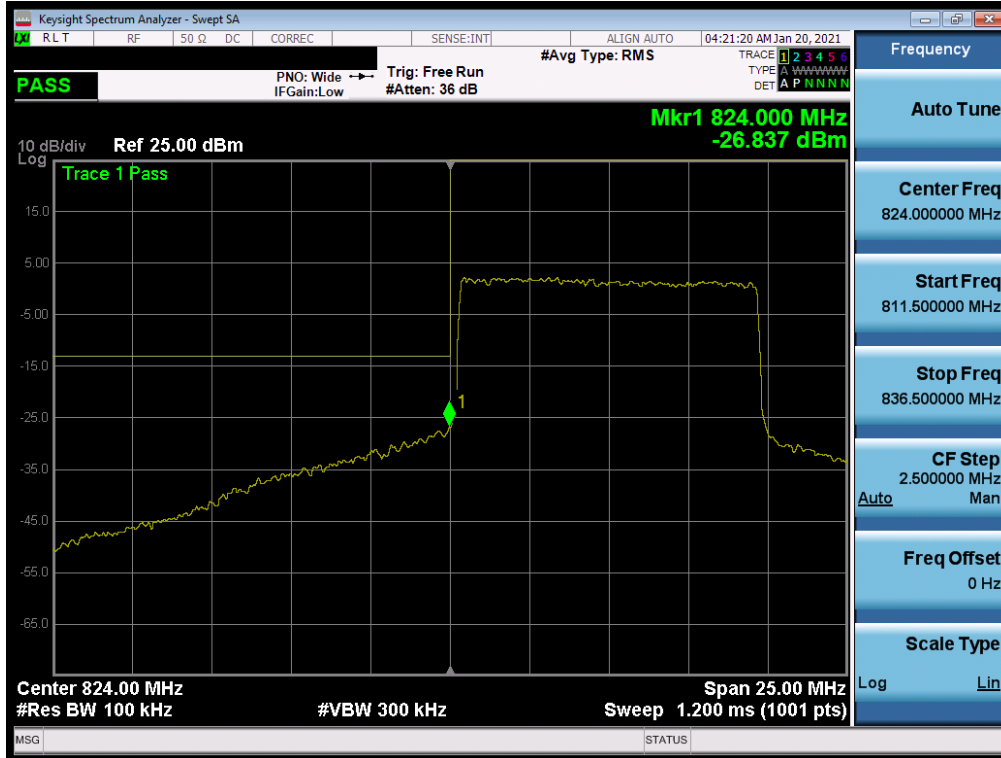
Plot 7-106. Lower Band Edge Plot (NR Band n5 – 10.0MHz - Full RB)
