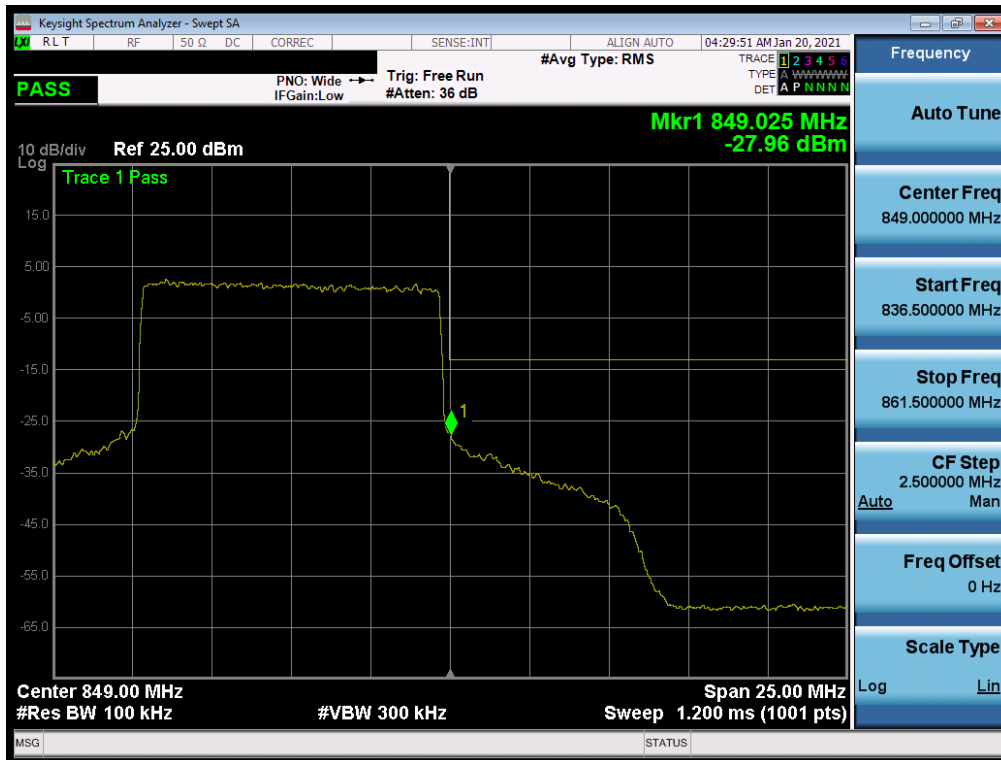
Plot 7-107. Upper Band Edge Plot (NR Band n5 – 10.0MHz - Full RB)
