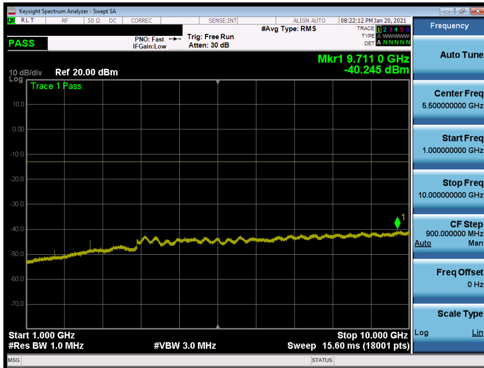
Plot 7-112. Conducted Spurious Plot (Band 5 – 10.0MHz QPSK – PCC 1/49 SCC 1/0 – Low Channel)
