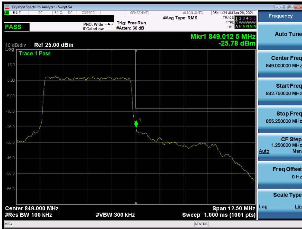
Plot 7-109. Upper Band Edge Plot (NR Band n5 – 5.0MHz - Full RB)
