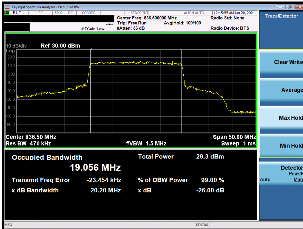
Plot 7-21. Occupied Bandwidth Plot (NR Band n5 - 20MHz QPSK - Full RB Configuration)
