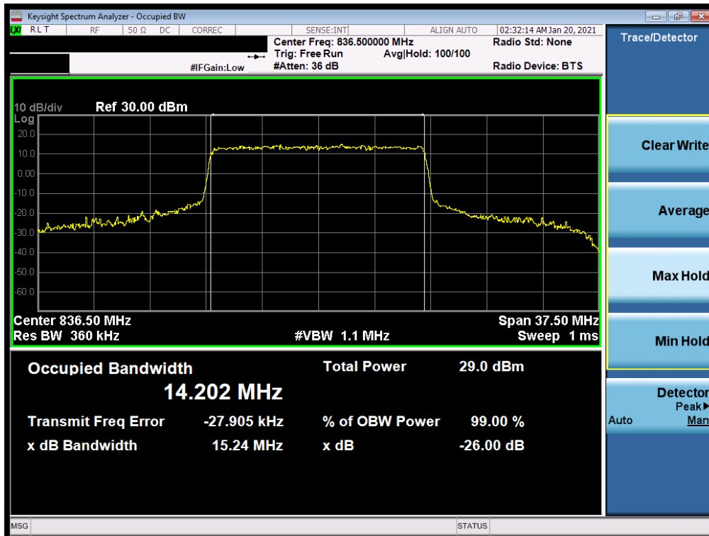
Plot 7-27. Occupied Bandwidth Plot (NR Band n5 - 15MHz 16-QAM - Full RB Configuration)
