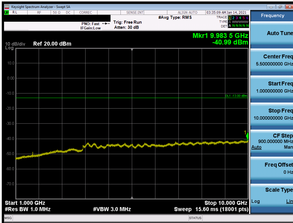
Plot 7-72. Conducted Spurious Plot (LTE Band 26/5 - 10MHz QPSK - RB Size 1, RB Offset 0 - Mid Channel)
