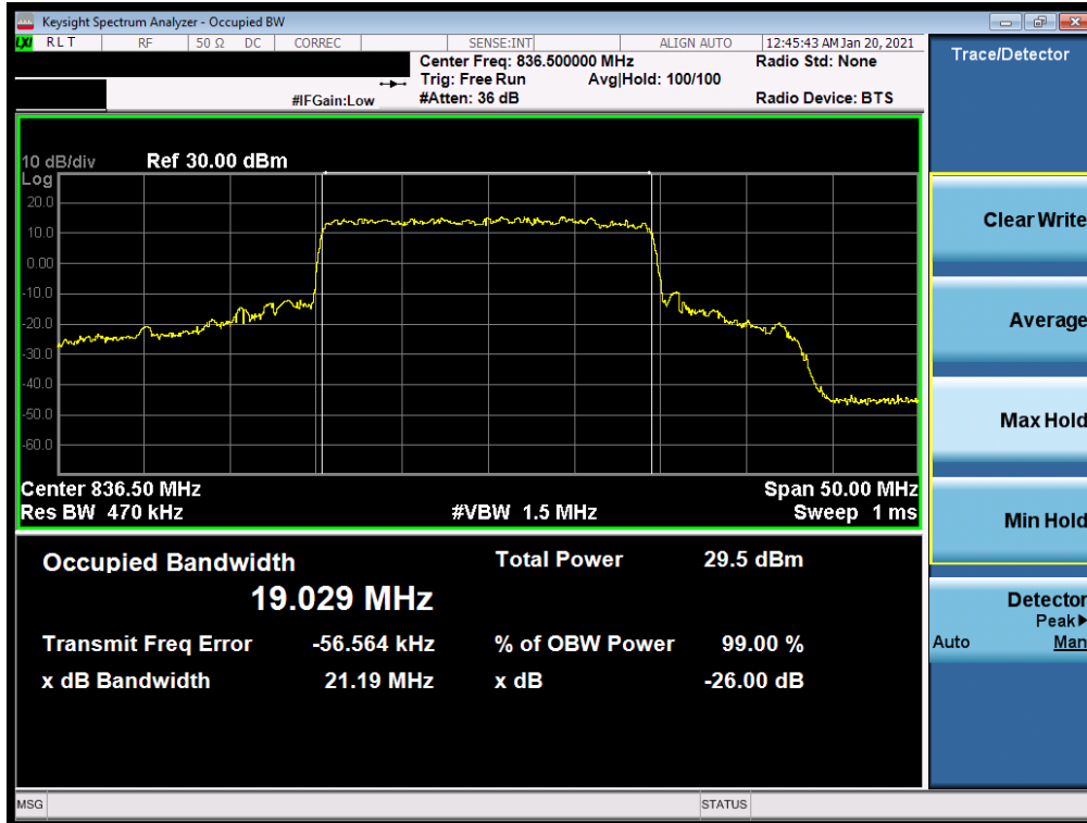
Plot 7-22. Occupied Bandwidth Plot (NR Band n5 - 20MHz 16-QAM - Full RB Configuration)
