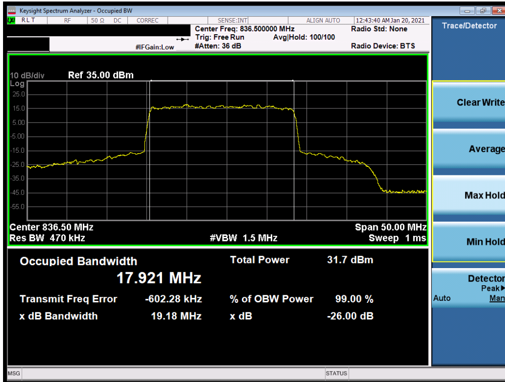
Plot 7-20. Occupied Bandwidth Plot (NR Band n5 - 20MHz \pi/2 BPSK - Full RB Configuration)
