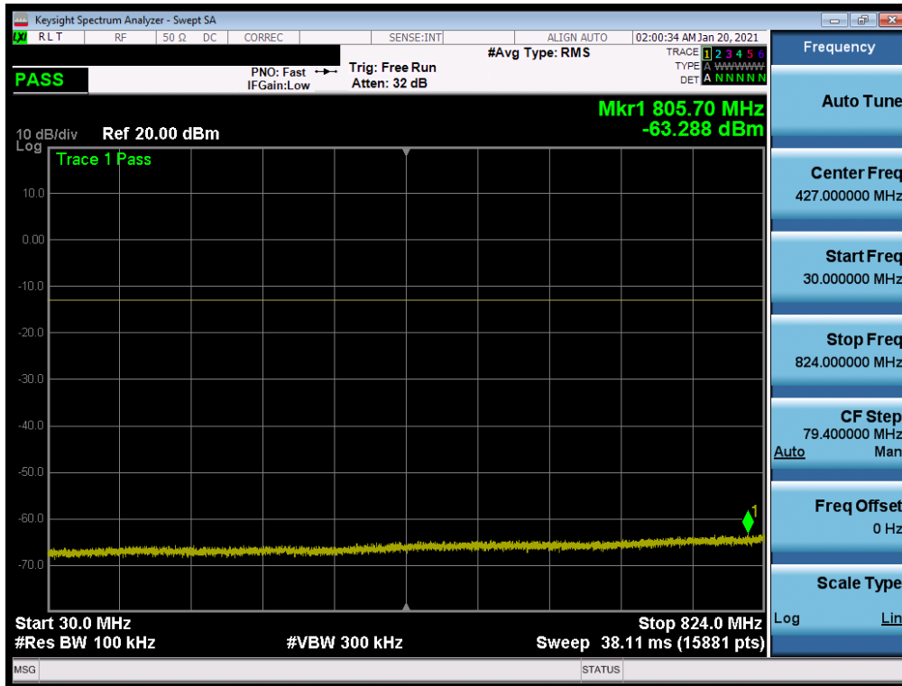
Plot 7-82. Conducted Spurious Plot (NR Band n5 - 20.0MHz - RB Size 1, RB Offset 0 - High Channel)
