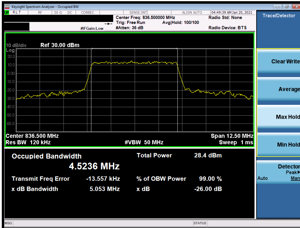
Plot 7-38. Occupied Bandwidth Plot (NR Band n5 - 5MHz 64-QAM - Full RB Configuration)
