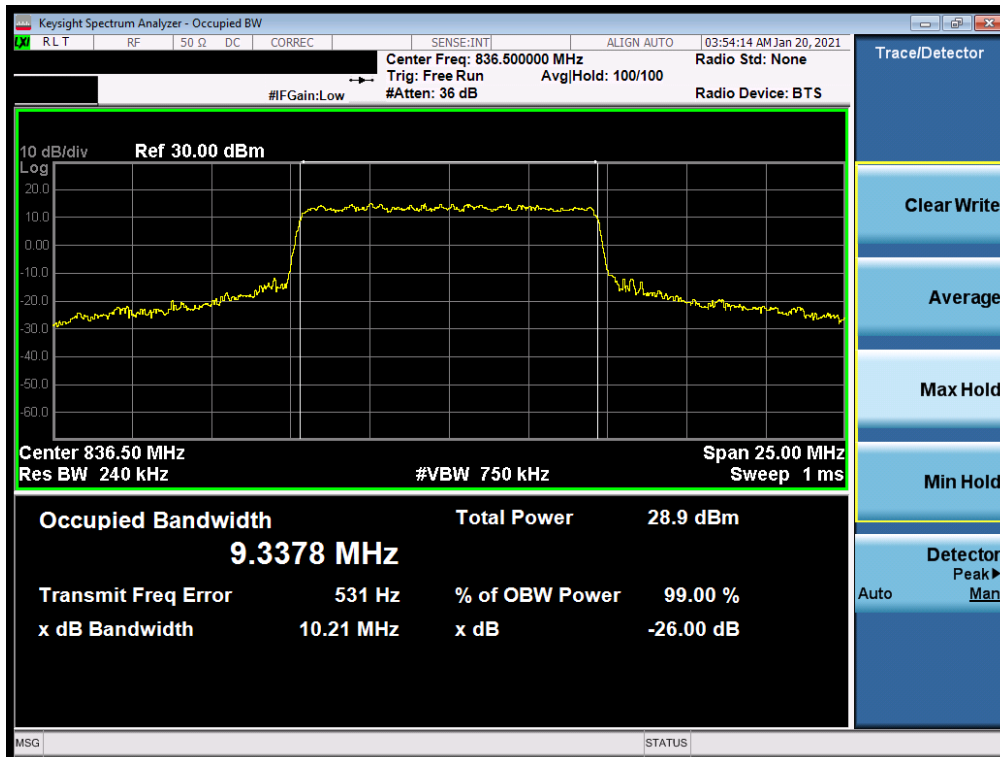
Plot 7-31. Occupied Bandwidth Plot (NR Band n5 - 10MHz QPSK - Full RB Configuration)
