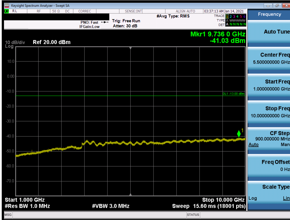
Plot 7-69. Conducted Spurious Plot (LTE Band 26/5 - 10MHz QPSK - RB Size 1, RB Offset 0 - Low Channel)
