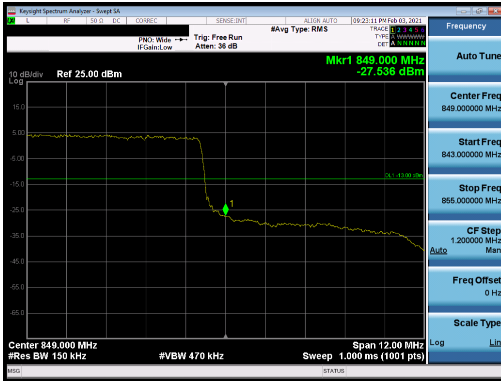
Plot 7-93. Upper Band Edge Plot (LTE Band 26 - 15MHz QPSK – Full RB Configuration)
