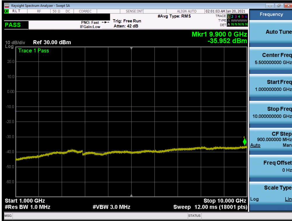
Plot 7-84. Conducted Spurious Plot (NR Band n5 - 20.0MHz - RB Size 1, RB Offset 0 - High Channel)
