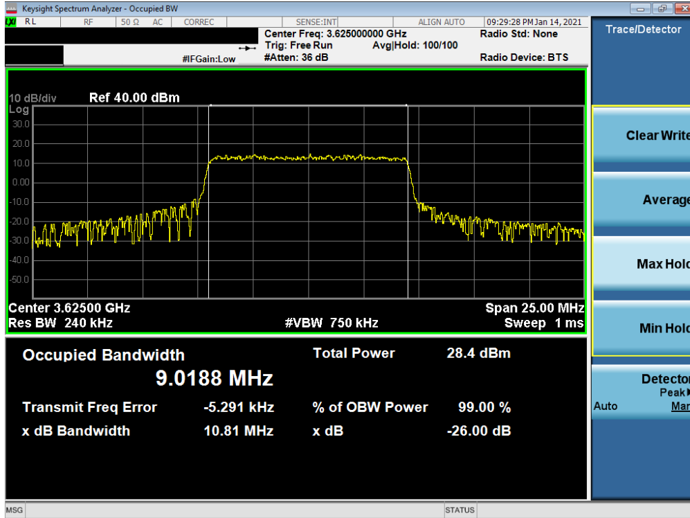
Plot 7-9. Occupied Bandwidth Plot (LTE Band 48 - 10MHz 64-QAM - Full RB Configuration)
