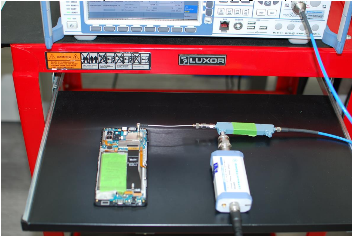
Test Setup Photo 2 – Conducted Test Setup (Figure 6-1a)
