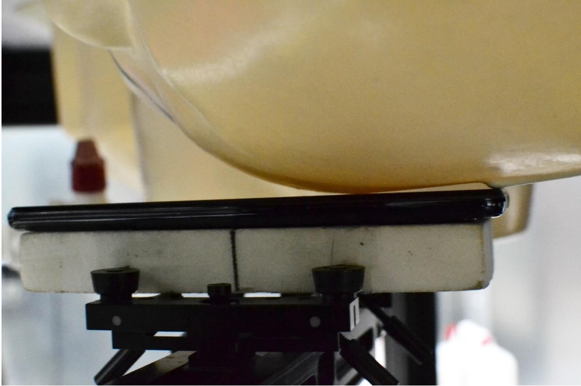
SAR Test Setup Photo 3 – Left Cheek
