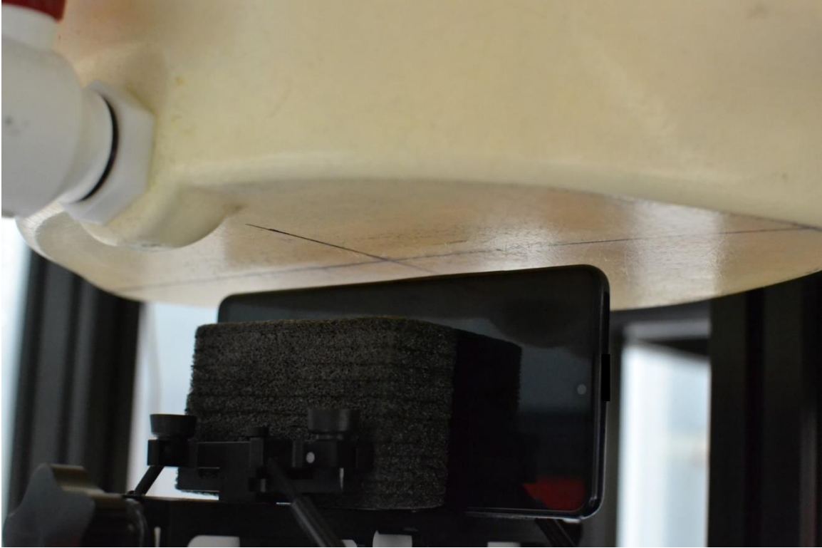
SAR Test Setup Photo 19 – Left Edge at 6mm
