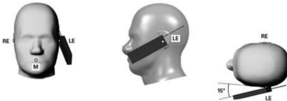
Figure 8.5. Tilt 15° position of the wireless device
