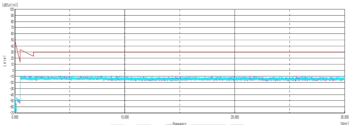
**Test results (Below 1 000 MHz) – Worst case: 802.11a / UNII-2C Middle frequency**
