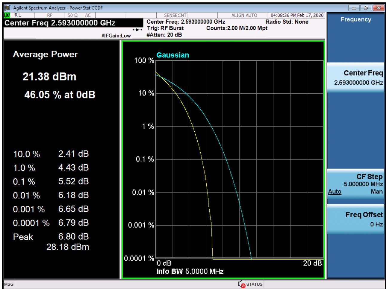
BAND 41. PAR Plot (5M BW\_Ch.40620\_16QAM\_RB25\_0)
