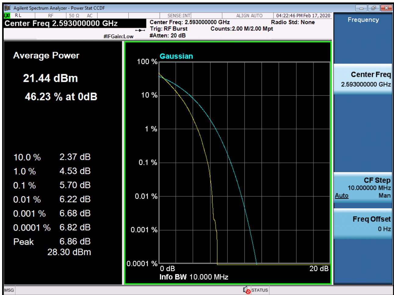
BAND 41. PAR Plot (10M BW\_Ch.40620\_16QAM\_RB50\_0)
