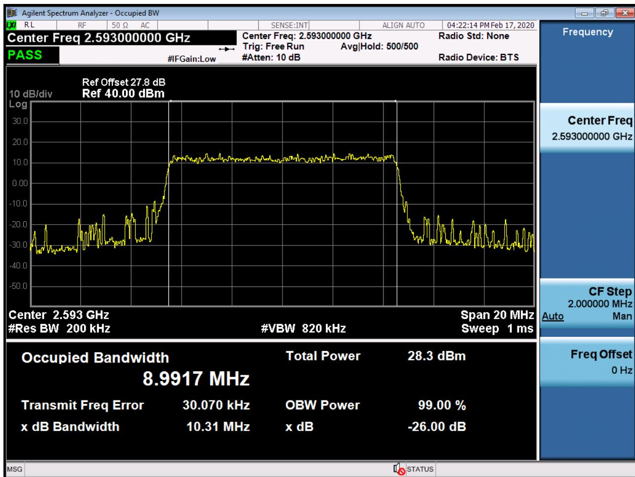
BAND 41. Occupied Bandwidth Plot (10 MHz Ch.40620 64-QAM RB 50)
