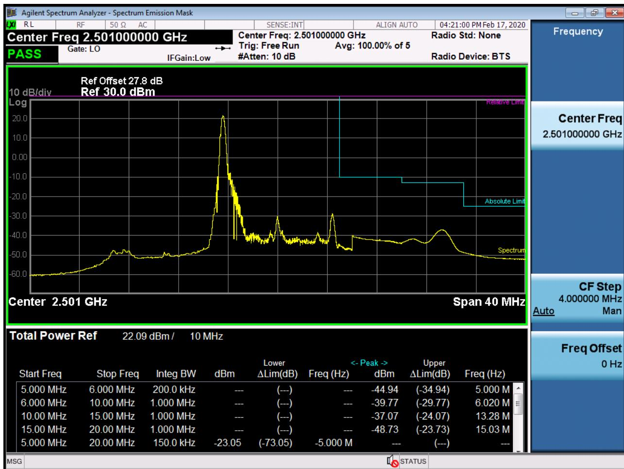
BAND 41. Low Channel Edge Plot (10 MHz Ch.39700 QPSK\_RB50\_Offset 0)-2
