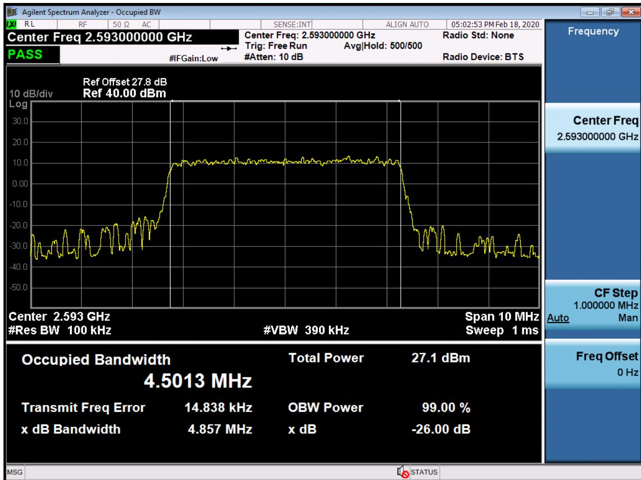
BAND 41. Occupied Bandwidth Plot (10 MHz Ch.40620 QPSK RB 50)
