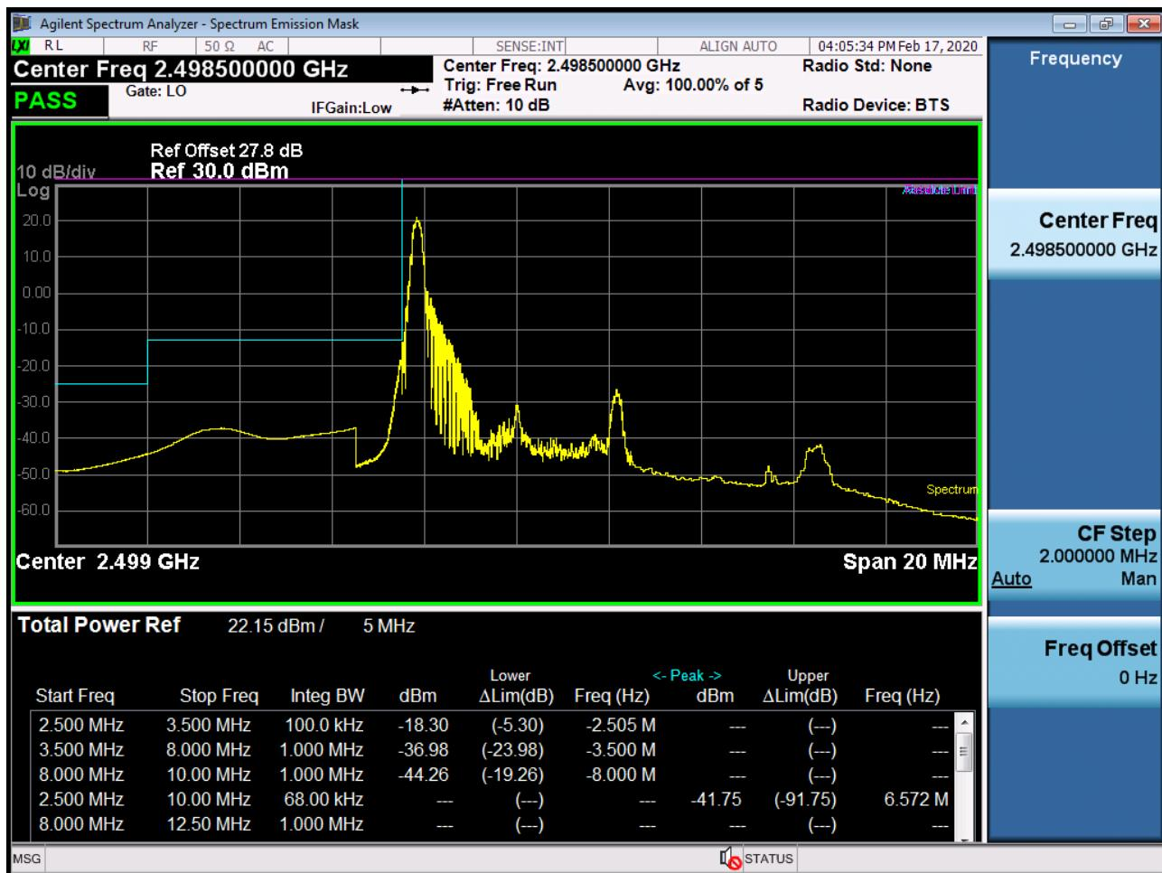
BAND 41. Low Channel Edge Plot (5 MHz Ch.39675 QPSK RB 25, Offset 0)-1
