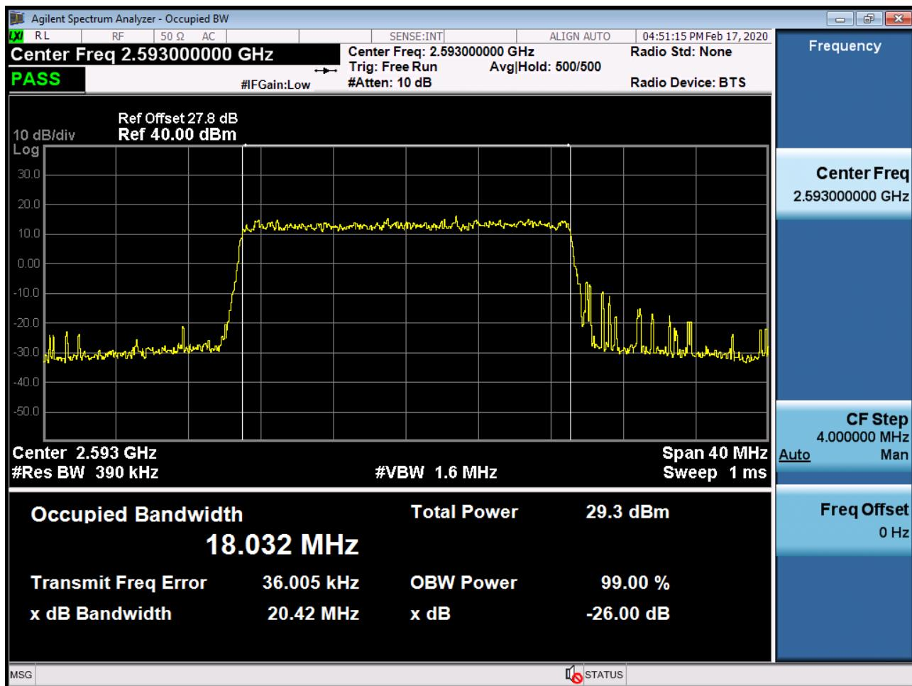
BAND 41. Occupied Bandwidth Plot (20 MHz Ch.40620 16-QAM RB 100)
