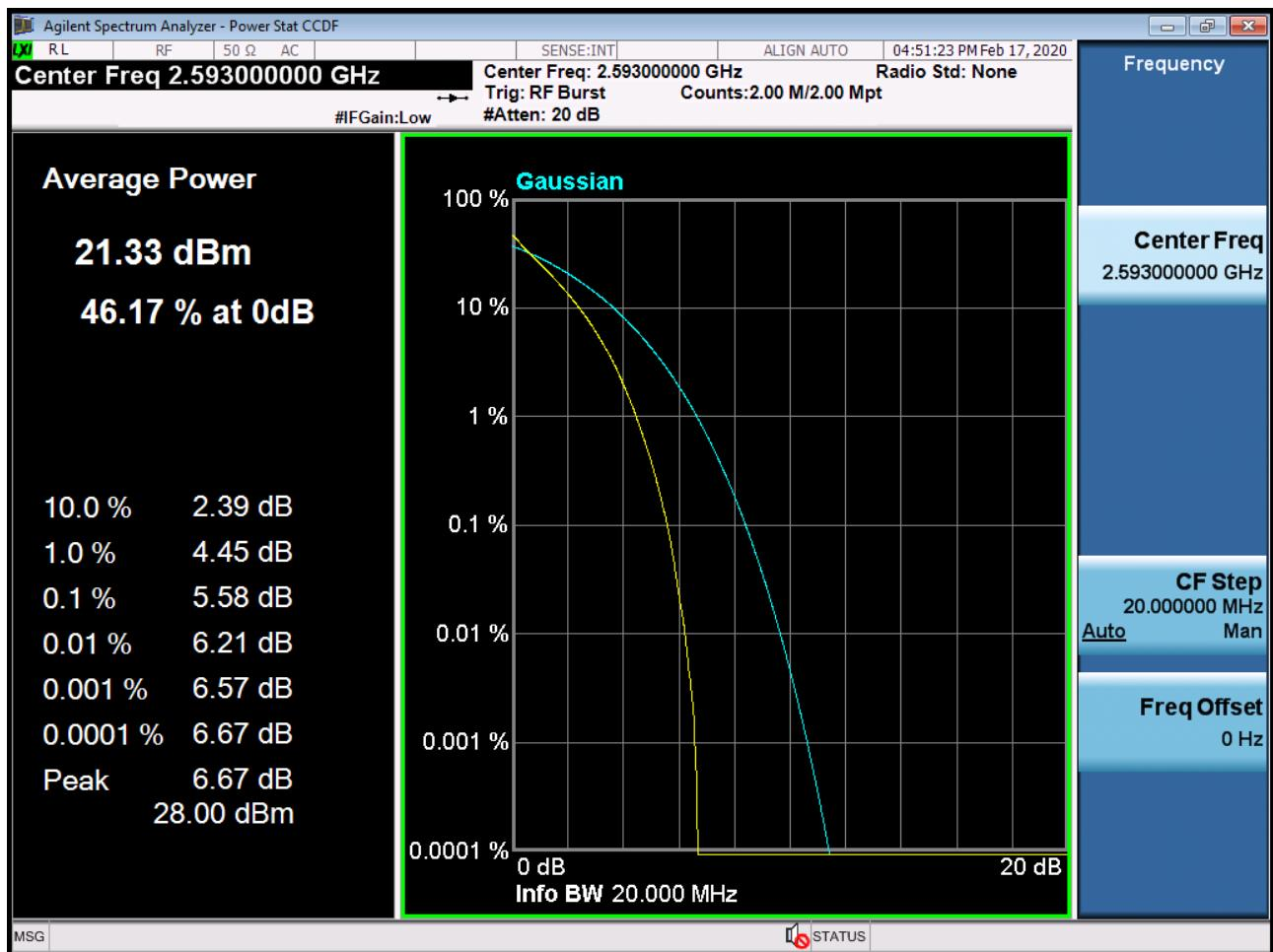
BAND 41. PAR Plot (20M BW\_Ch.40620\_16QAM\_RB100\_0)
