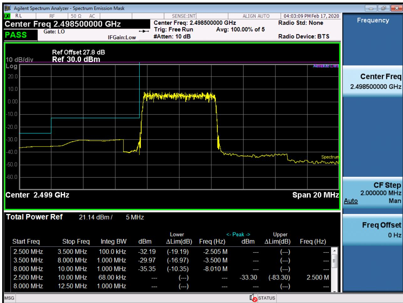
BAND 41. Low Channel Edge Plot (5 MHz Ch.39675 QPSK\_RB1\_Offset 0)-2
