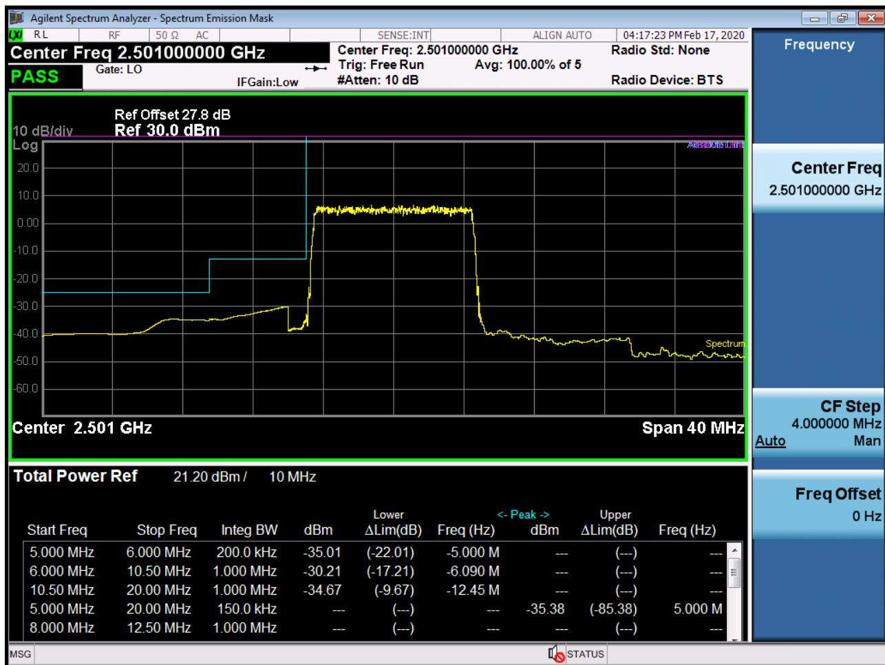
BAND 41. Low Channel Edge Plot (10 MHz Ch.39700 QPSK\_RB1\_Offset 0)-2
