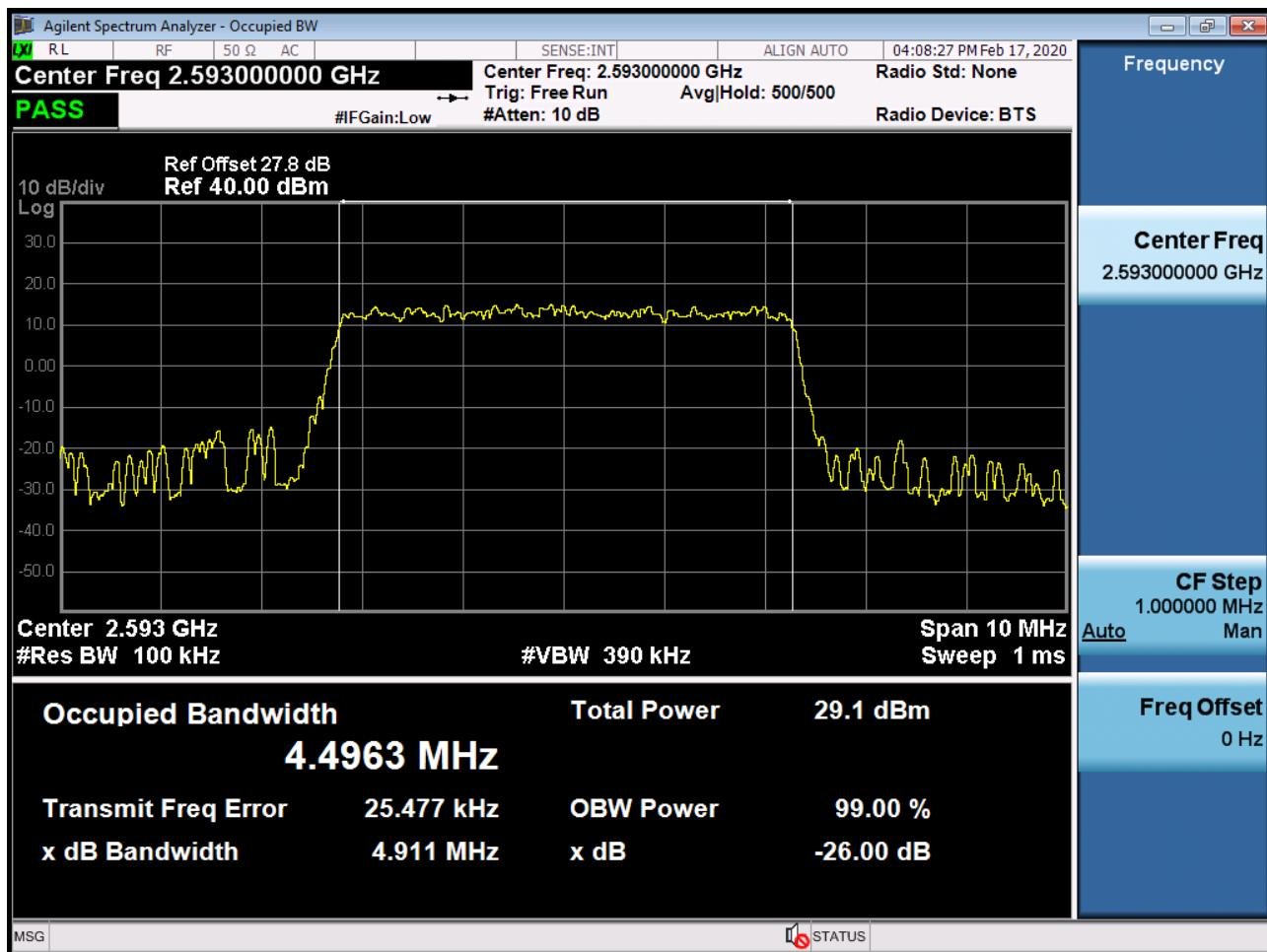
BAND 41. Occupied Bandwidth Plot (5 MHz Ch.40620 16-QAM RB 25)
