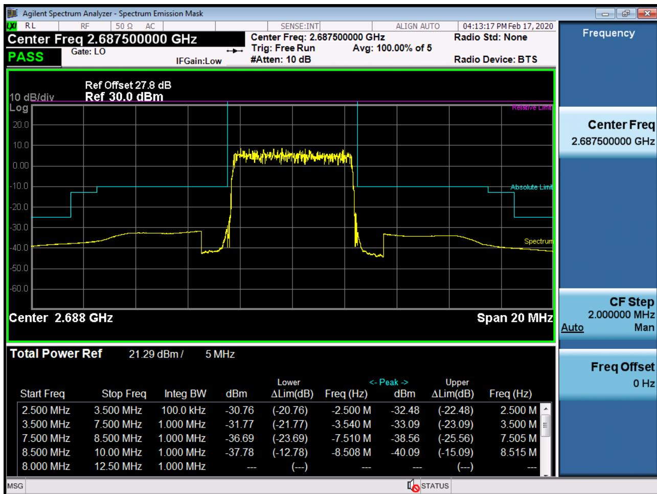
BAND 41. Low Channel Edge Plot (10 MHz Ch.39700 QPSK RB 1, Offset 0)-1
