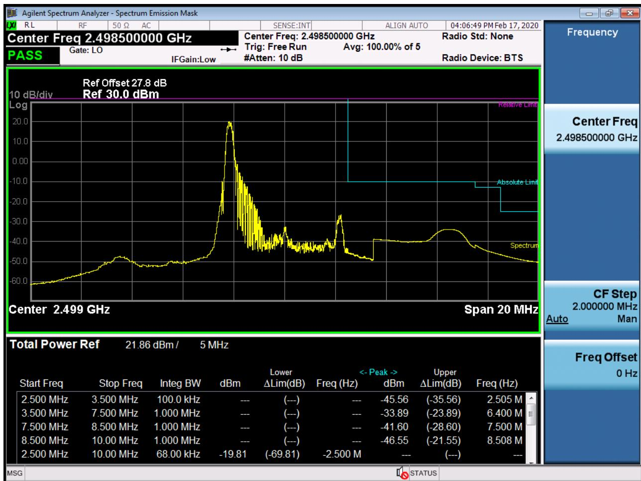
BAND 41. Low Channel Edge Plot (5 MHz Ch.39675 QPSK\_RB25\_Offset 0)-2
