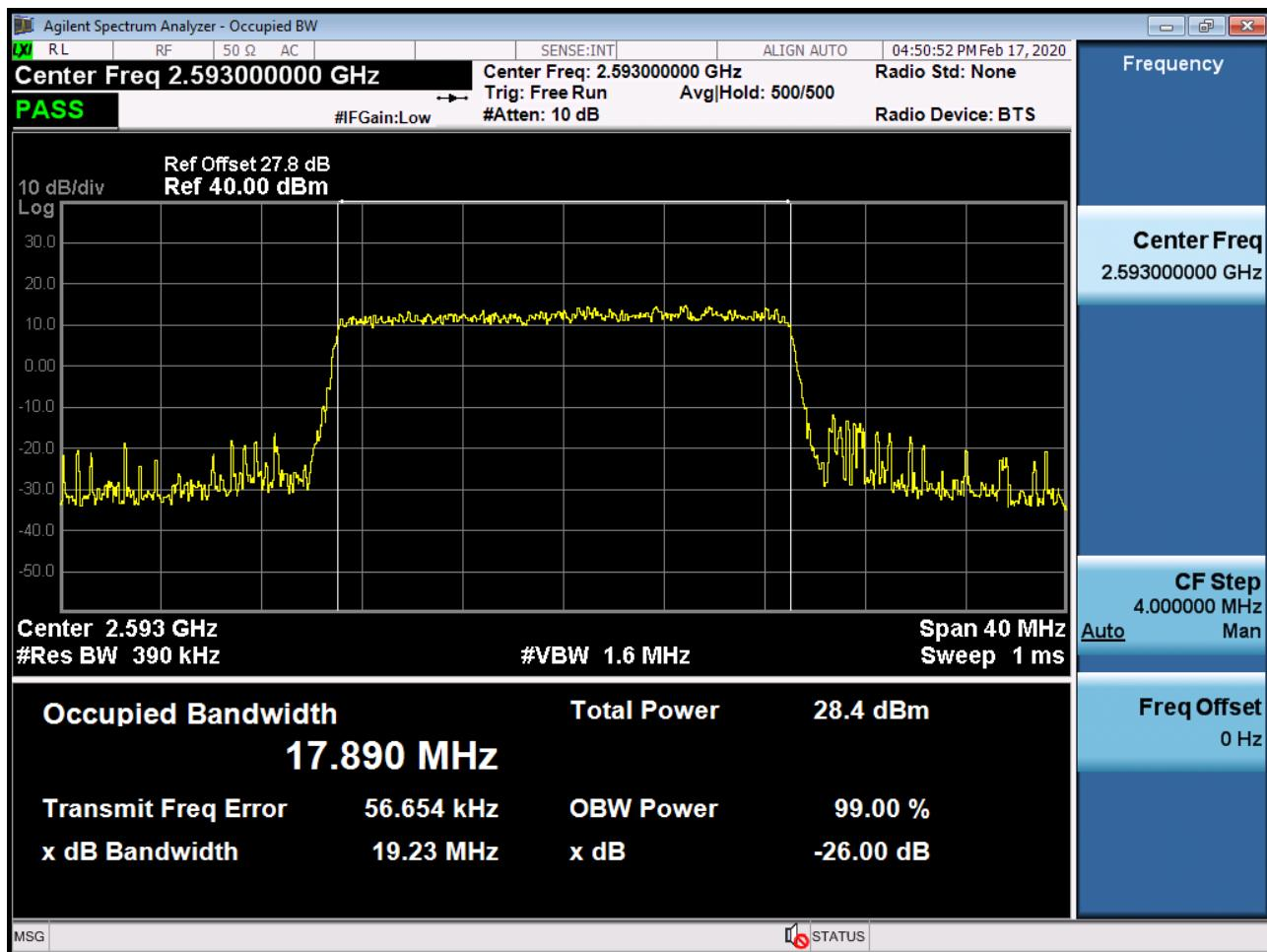
BAND 41. Occupied Bandwidth Plot (20 MHz Ch.40620 64-QAM RB 100)
