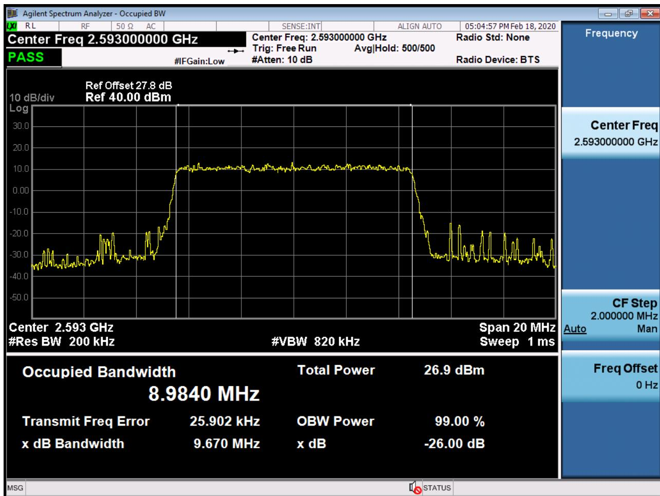
BAND 41. Occupied Bandwidth Plot (15 MHz Ch.40620 QPSK RB 75)
