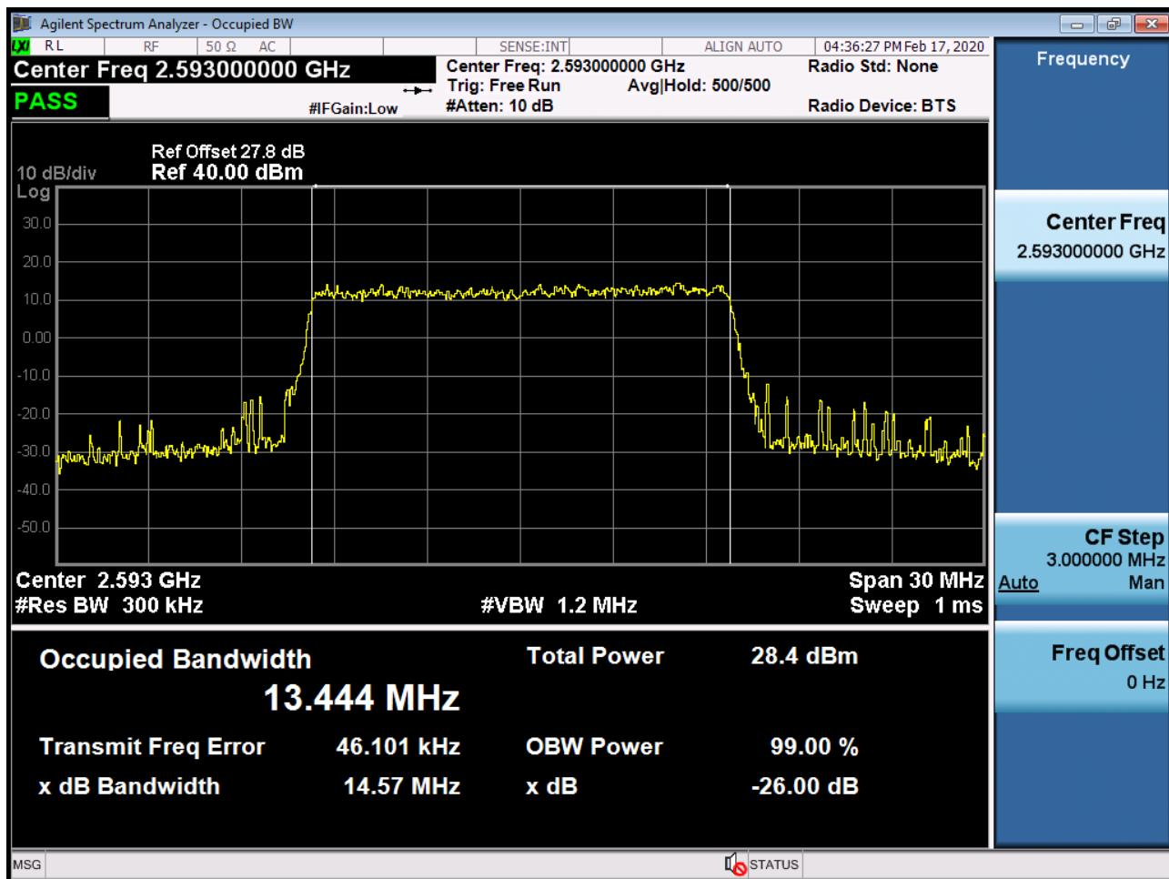
BAND 41. Occupied Bandwidth Plot (15 MHz Ch.40620 64-QAM RB 75)
