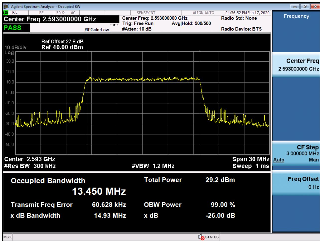
BAND 41. Occupied Bandwidth Plot (15 MHz Ch.40620 16-QAM RB 75)
