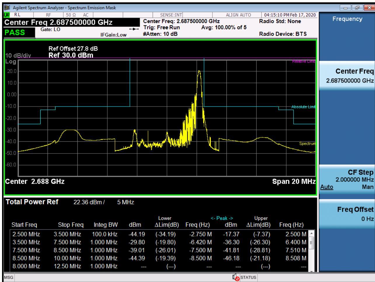
BAND 41. High Channel Edge Plot (5 MHz Ch.41565 QPSK\_RB25\_Offset 0)
