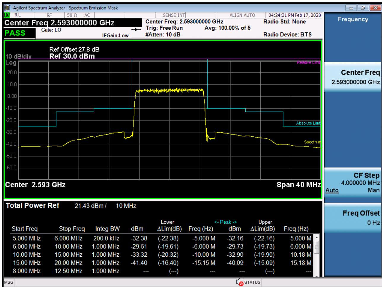
BAND 41. High Channel Edge Plot (10 MHz Ch.41540 QPSK RB 1, Offset 49)
