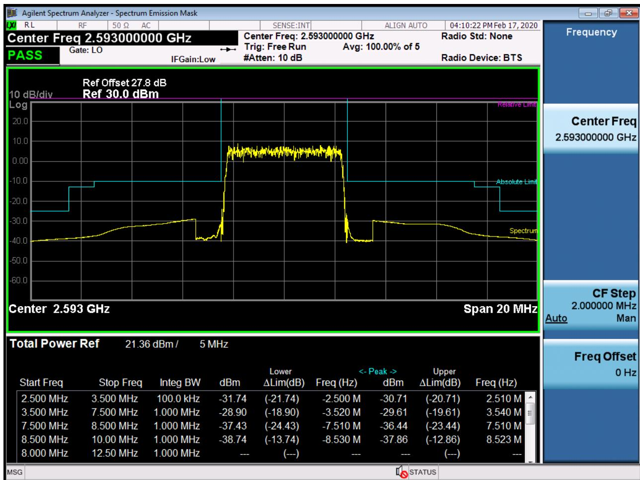
BAND 41. High Channel Edge Plot (5 MHz Ch.41565 QPSK RB 1, Offset 24)
