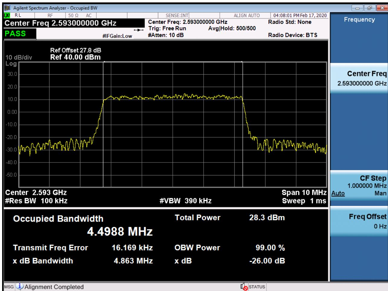
BAND 41. Occupied Bandwidth Plot (5 MHz Ch.40620 64-QAM RB 25)
