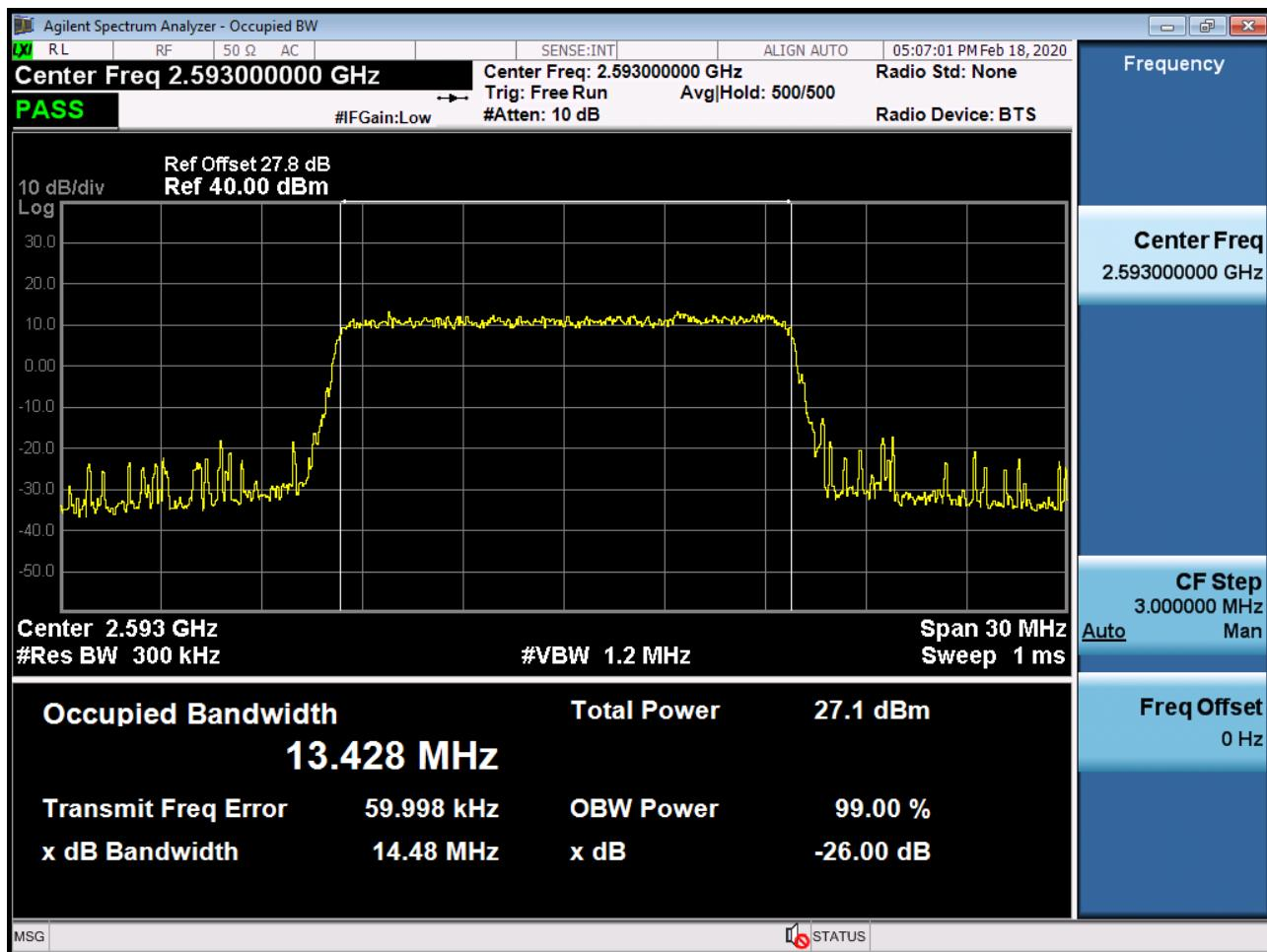
BAND 41. Occupied Bandwidth Plot (20 MHz Ch.40620 QPSK RB 100)
