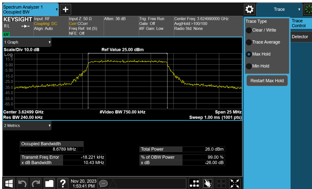
Plot 7-30. Occupied Bandwidth Plot (NR Band n48 - 10MHz QPSK - Full RB Configuration)
