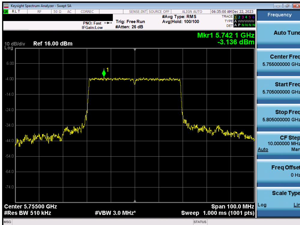
Plot 7-110. Power Spectral Density Plot MIMO ANT2 (40MHz BW 802.11ax (UNII Band 3) – Ch. 151)
